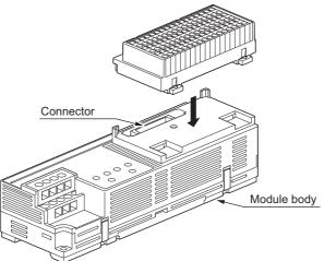
3) Tighten the fixing screws. (Tightening torque range: 0.34 to 0.46N•m)
