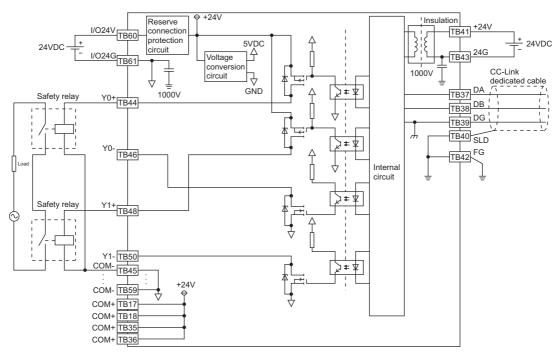
Figure 6.16 Wiring example (source and source outputs)
