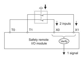
Figure 4.1 Double input wiring
