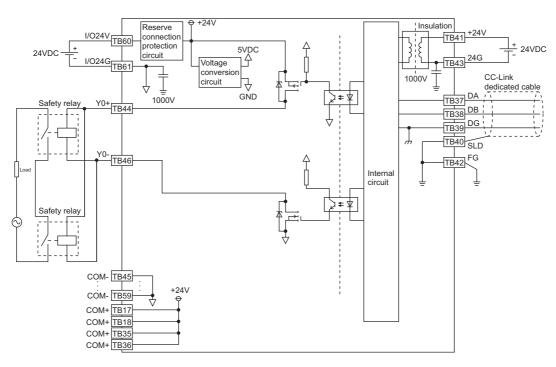
Figure 6.15 Wiring example (sink and source outputs)
