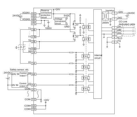
Figure 6.17 Wiring example (with a safety switch (2 NC contacts) and a safety sensor)
