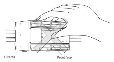
Figure 6.4 Installation to DIN rail
