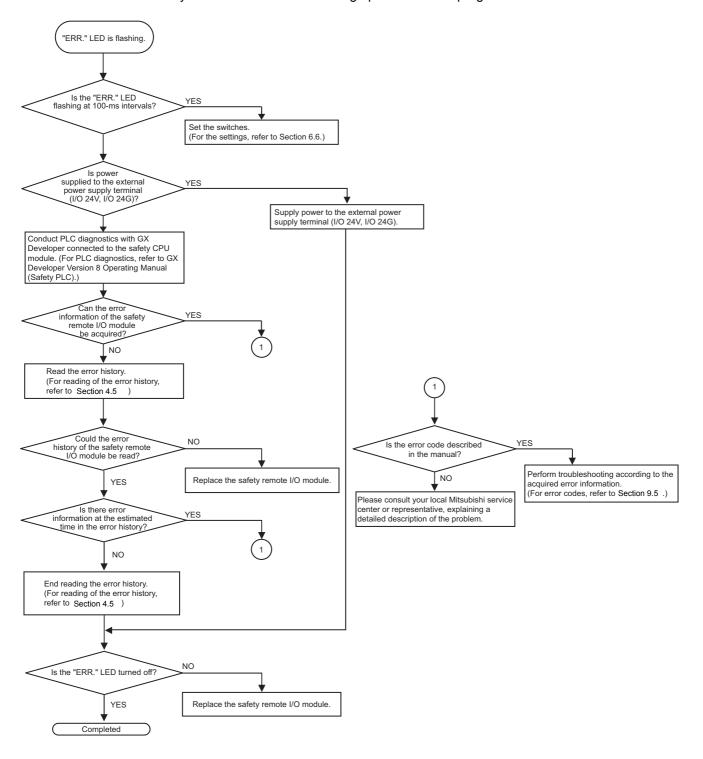
Figure 9.4 Flowchart for when the "ERR." LED flashes
