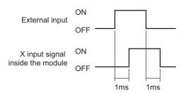
Figure 4.3 Delay of input signal
