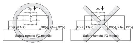
Figure 6.10 Combination example of input terminals
