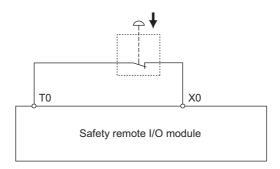
Figure 4.2 Single input wiring
