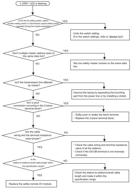
Figure 9.7 Flowchart for when the "L ERR." LED flashes
