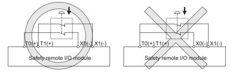
Figure 6.11 Combination example of test pulse terminals
