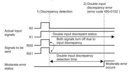
Figure 5.12 Operation of the double input discrepancy detection
