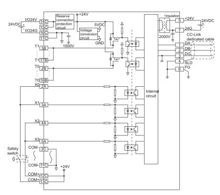
Figure 6.18 Wiring example (with a safety switch (1 NC/1 NO contacts))
