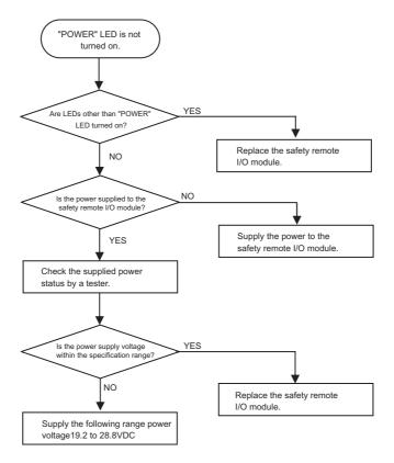
Figure 9.2 Flowchart for when the "POWER" LED does not turn on
