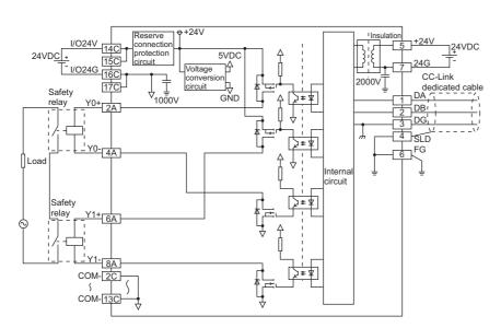
Figure 6.19 Wiring example (sink and source outputs)
