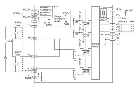
Figure 6.20 Wiring example (source and source outputs)
