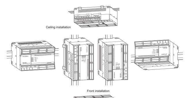
Figure 1.1 Module installation orientation
