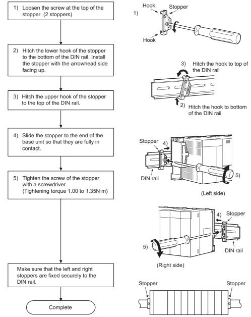
Figure 10.10 Fixture mounting procedure
