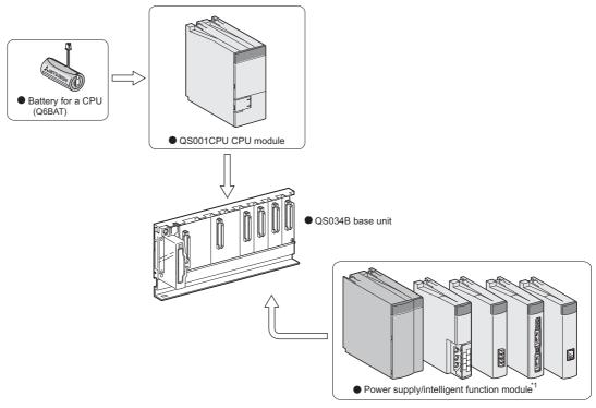
Figure 2.1 System configuration
