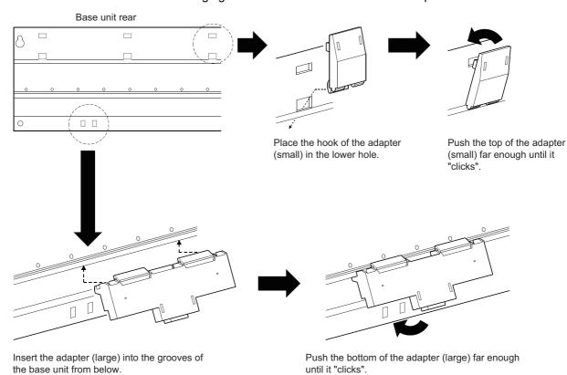
Figure 10.5 Adapter installation method
