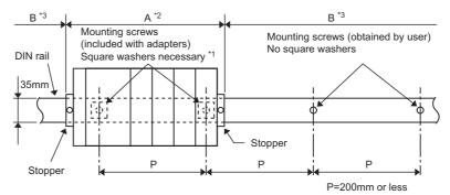
Figure 10.7 DIN rail mounting screw intervals
