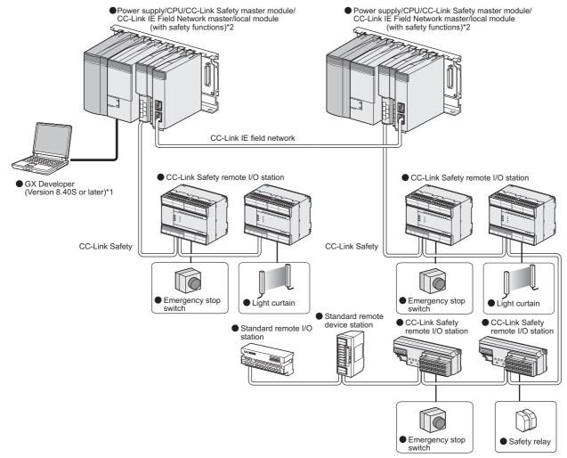
Figure 1.1 Safety programmable controller system
