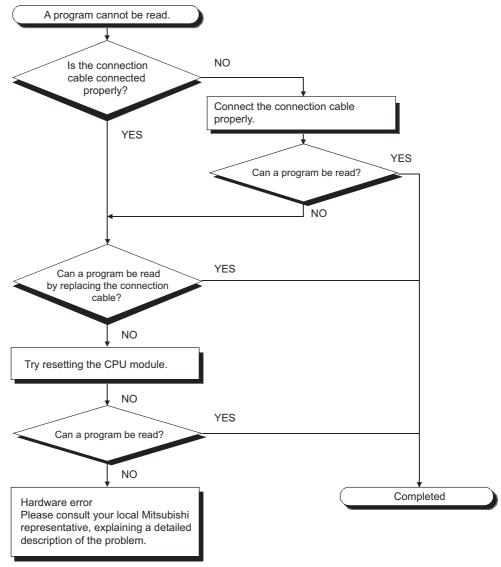
Figure 12.6 Flowchart for when a program cannot be read
