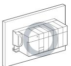
Figure 10.14 Orientation in which modules can be mounted
