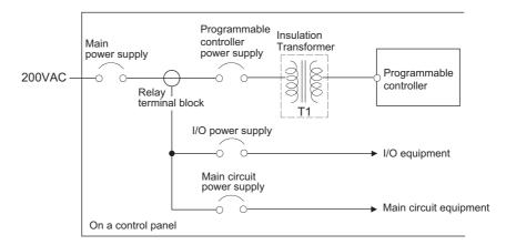
Figure 10.21 Power supply connection diagram
