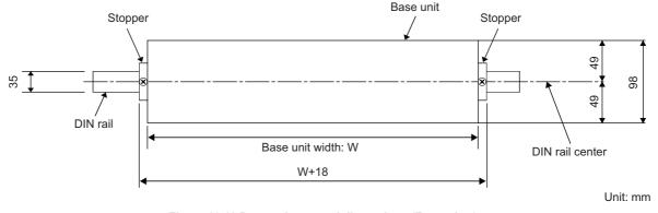
Figure 10.11 Base unit external dimensions (Front view)
