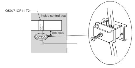
Figure 9.9 AD75CK cable clamp mounting position
