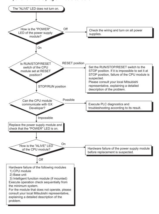
(2) When the "ALIVE" LED of the CPU module turns off during operation of the programmable controller
