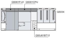
Figure 10.1 System configuration
