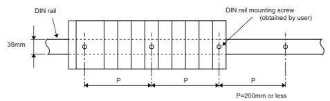
Figure 10.6 DIN rail mounting screw intervals
