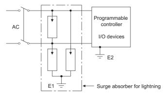
Figure 10.22 Connecting a lightning surge absorber
