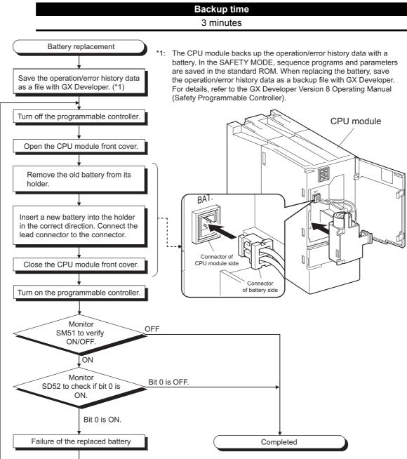
Figure 11.2 Replacement procedure for the Q6BAT battery
