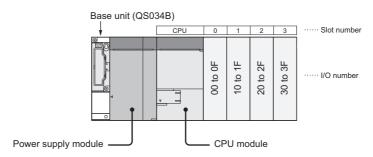
Figure 2.2 System configuration
