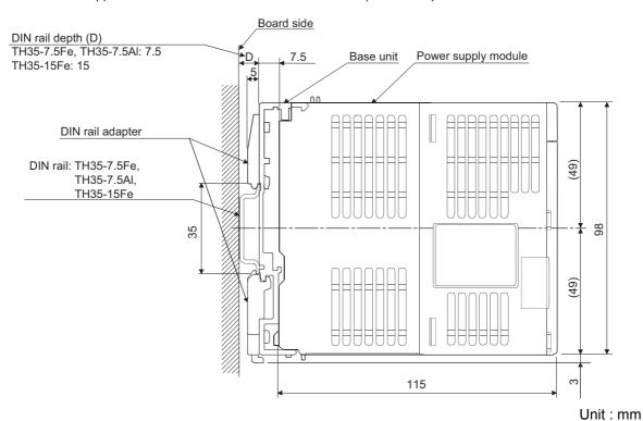
Figure 10.12 External dimensions (Side view)
