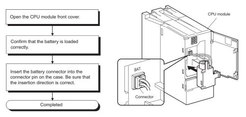
Figure 7.1 Q6BAT battery setting procedure
