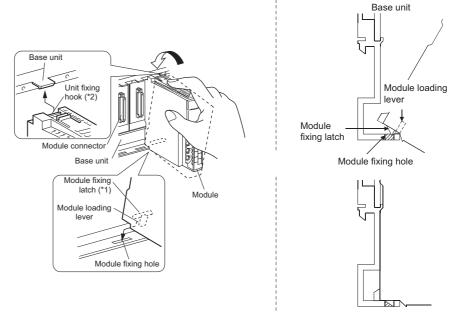
Figure 10.17 Module mounting procedure
