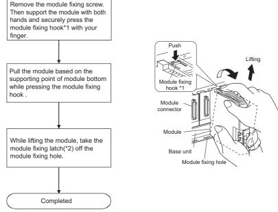
Figure 10.19 Module removal procedure
