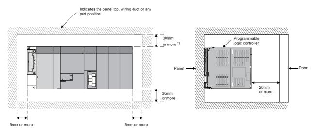
\* 1: For wiring duct with 50mm or less height. For other cases, 40mm or more.
