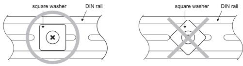
Figure 10.9 Precautions when mounting a square washer
