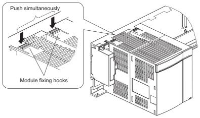
Figure 10.20 Power supply module and CPU module removal procedure
