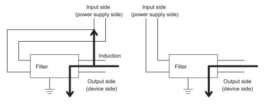
The noise will be induced when the input and output wires are bundled.
