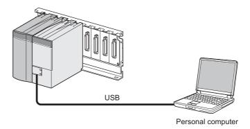
Figure 1.3 Connection to a personal computer using USB
