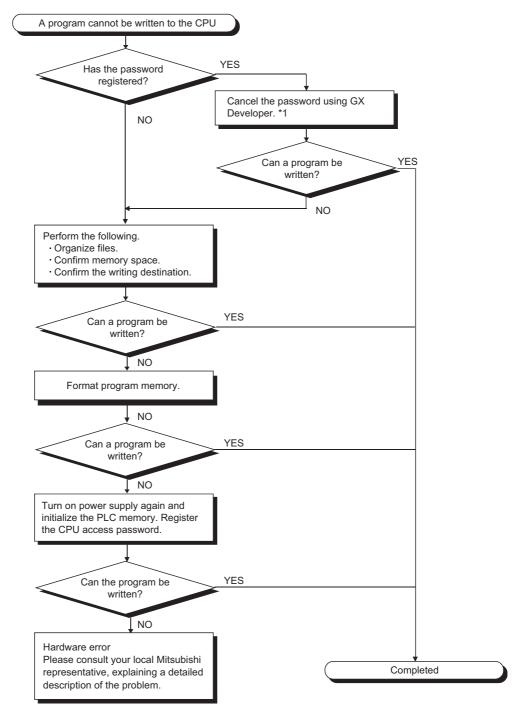
\* 1: If the password registration cannot be canceled due to the loss of password, initialize the PLC memory with GX developer. The PLC memory initialization initializes the memory of the CPU module (i.e. deletes all information in the CPU module) and resets the memory to the factory default.
