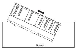
Figure 10.3 Install a base unit
