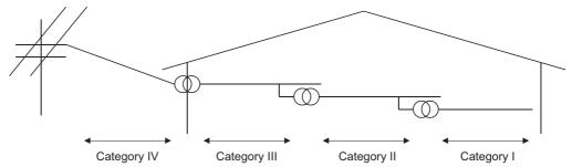
Figure 9.12 Installation category for power supply module
