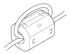
Figure 9.10 For number of winding is two turns or more
