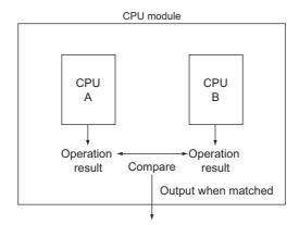
Figure 1.2 Redundant CPU
