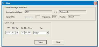
Diagram 6.23 Clock data write from GX Developer
