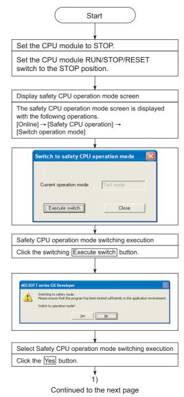
Diagram 6.5 TEST MODE to SAFETY MODE switching
