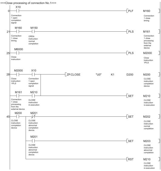
Fig.App.2 Program example using I/O signals
