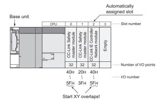
Diagram 4.5 Start XY set by above I/O assignment
