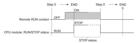
Diagram 6.24 Time Chart for RUN/STOP with RUN Contact
