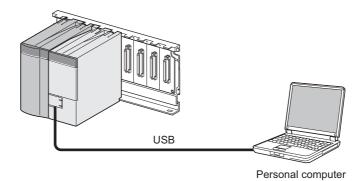
Figure 1.3 Connection to a personal computer using USB
