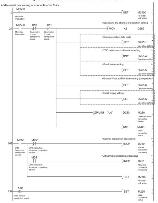
Fig.App.5 Program example using I/O signals
