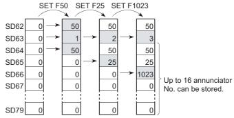
Diagram 9.11 Processing at annunciator ON
