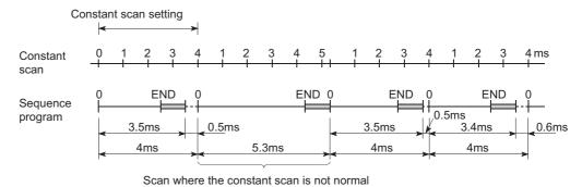
Diagram 6.17 Operation when the Scan Time is longer than the Constant Scan setting time
