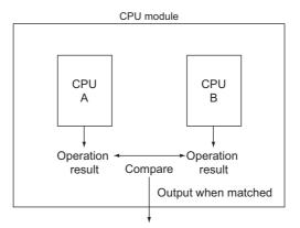
Figure 1.2 Redundant CPU
