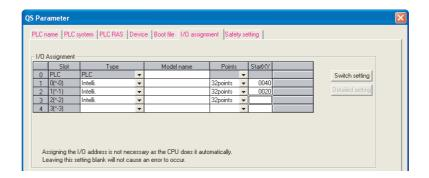
Diagram 4.4 I/O assignment with overlapping start XY
