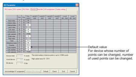
Diagram 9.1 Device in PLC parameter dialog box
