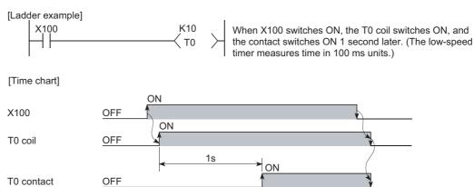
Diagram 9.18 Ladder example and timing chart of low-speed timer
