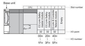
Diagram 4.6 System configuration and I/O number assignment
