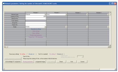
Diagram 8.11 Setting the number of Ethernet/CC IE/MELSECNET cards screen (for Ethernet setting)
