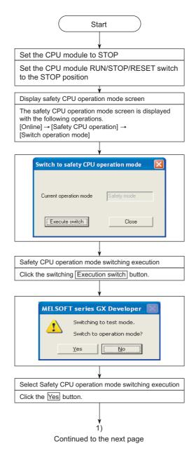
Diagram 6.6 SAFETY MODE to TEST MODE switching
