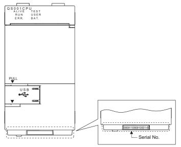
Diagram 1.12 CPU module front display
