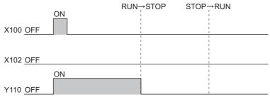
Diagram 6.20 Timing chart when output (Y) is set to clear
