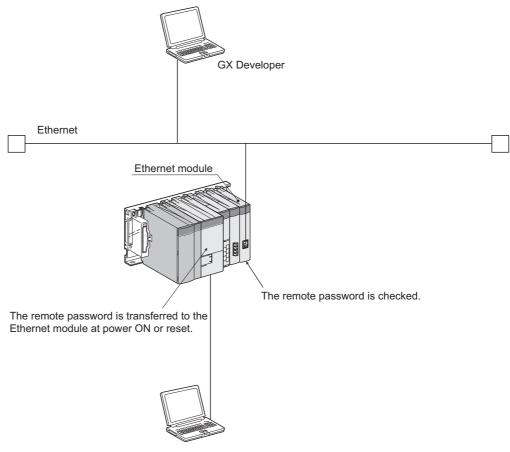
GX Developer sets, changes or deletes the remote password and then write the result to the CPU module.
