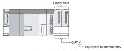
Diagram 9.8 Substitute for internal relay
