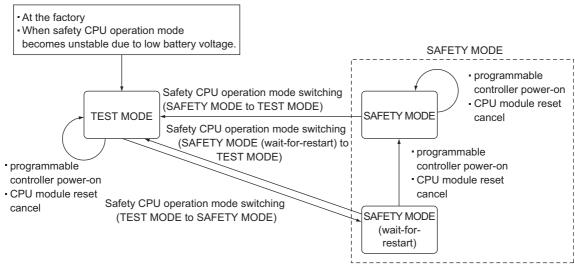
Diagram 6.3 State when the safety CPU operation mode is switched
