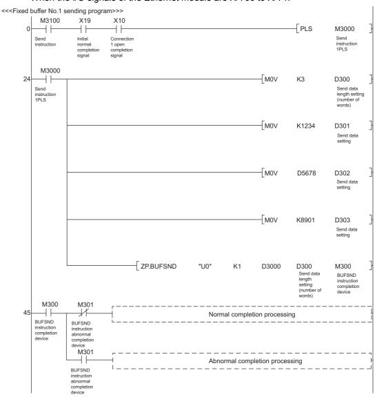
Fig.App.4 Program example using I/O signals
