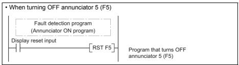
Diagram 9.12 Example of turning OFF the annunciators
