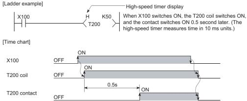
Diagram 9.19 Ladder example and timing chart of high-speed timer
