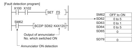
Diagram 9.10 Detection and storage of annunciator ON
