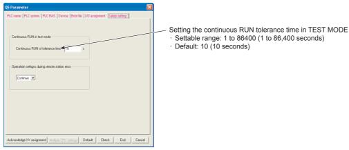
Diagram 6.12 PLC parameter safety setting screen
