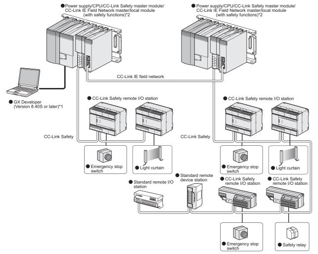
Figure 1.1 Safety programmable controller system
