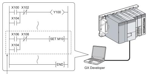
Change by GX Developer and write in CPU module at the conversion
