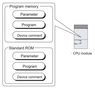
Diagram 5.1 Data handled by CPU module
