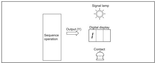
Diagram 9.6 Output from CPU module to external devices
