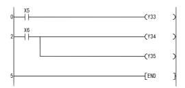
(2) When Bit Designation has been Made for Word Device [Ladder Mode]
