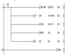
If the data set at X10 to X37 is a BCD value which exceeds 2147483647, the value at D0 and D1 will be a negative value, because it exceeds the range of numerical values that can be handled by a 32-bit device.
