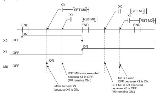
When specifying output (Y) in SET/RST instruction, the ON/OFF status of the device at the execution of the last instruction in the scan is returned as the output (Y).
