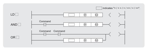
🛐 , 🥹 : Data for comparison or start number of the devices where the data for comparison is stored (BIN 16 bits)
