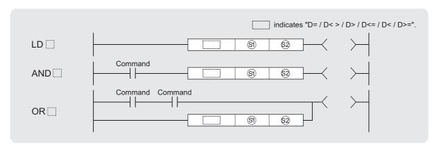
§1, §2 : Data for comparison or start number of the devices where the data for comparison is stored (BIN 32 bits)
