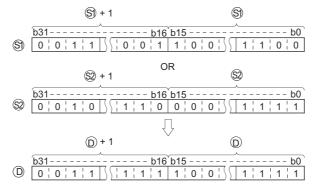
(2) When bit devices are designated, the bit devices below the points designated as digits are regarded as "0" in the operation. (See Program Example (2))
