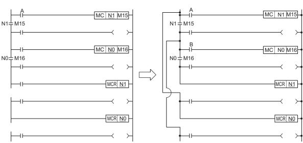
(2) If the nesting architecture results in MCR instructions concentrated in one location, all master controls can be terminated by use of just the lowest nesting number (N).
