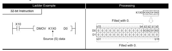
Fig 3.5 Ladder Example and Processing Conducted
