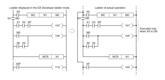
Inputting contacts on the vertical bus is not necessary when programming in the write mode of the GX Developer.
