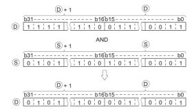
(2) When bit devices are designated, the bit devices below the points designated as digits are regarded as "0" in the operation. (See Program Example (2))
