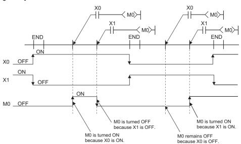
When specifying output (Y) in OUT instruction, the ON/OFF status of the device at the execution of the last OUT instruction in the scan is returned as the output (Y).
