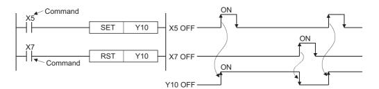
(3) When the execution command is OFF, the status of devices does not change.
