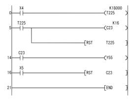
When T225 is set as retentive timer, it is turned ON when X4 ON time reaches 30 min.
