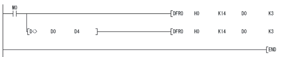
Figure 5.13 Periodic pulse counter value reading program example
