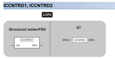
The following instruction can go in the dotted squares. ICCNTRD1, ICCNTRD1P, ICCNTRD2, ICCNTRD2P
