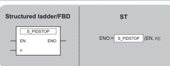
The following instruction can go in the dotted squares. S\_PIDSTOP, SP\_PIDSTOP, S\_PIDRUN, SP\_PIDRUN
