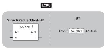
The following instruction can go in the dotted squares. ICLTHRD1, ICLTHRD1P, ICLTHRD2, ICLTHRD2P
