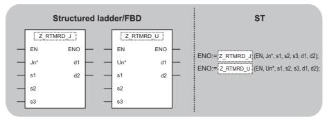
The following instruction can go in the dotted squares. Z\_RTMRD\_J, ZP\_RTMRD\_J, Z\_RTMRD\_U, ZP\_RTMRD\_U
