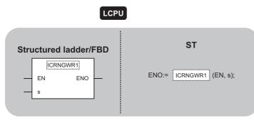
The following instruction can go in the dotted squares. ICPREWR1, ICPREWR1P, ICPREWR2, ICPREWR2P
