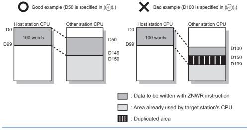
\*3 End device No. of the device in the host station CPU, and whose device name is same as in (d1)
