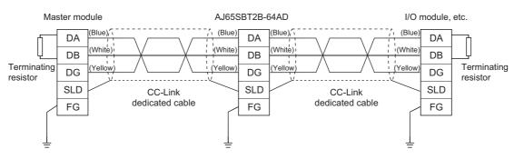
Figure 4.5 Connecting modules using CC-Link dedicated cables
