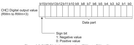
Figure 3.7 CH Digital output value (RWrn to RWrn+3)
