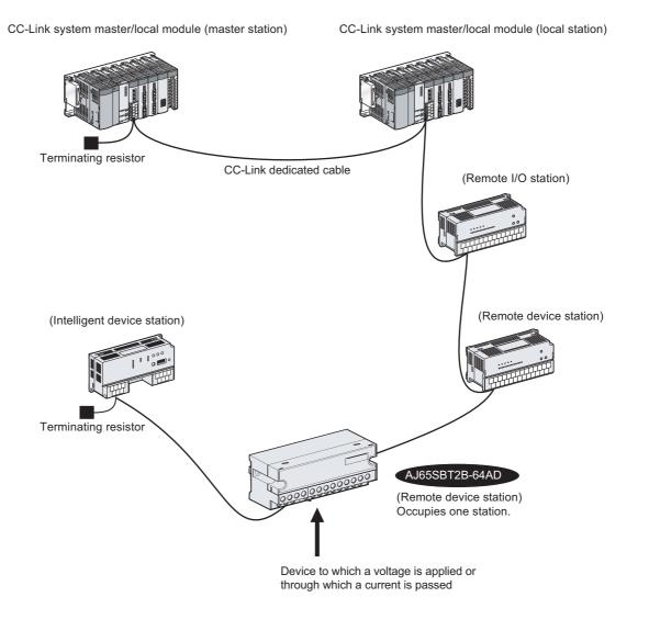
Figure 2.1 Overall configuration when using the AJ65SBT2B-64AD
