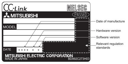
Figure 2.2 Checking the hardware version
