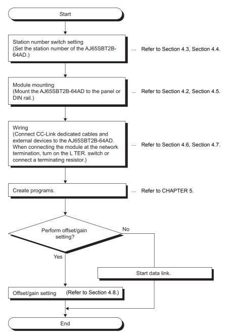
Figure 4.1 The procedure before operation
