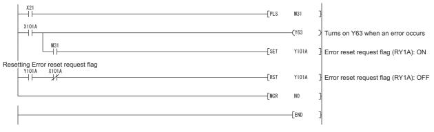
Figure 5.15 Program example (when using the QnACPU) 2/2
