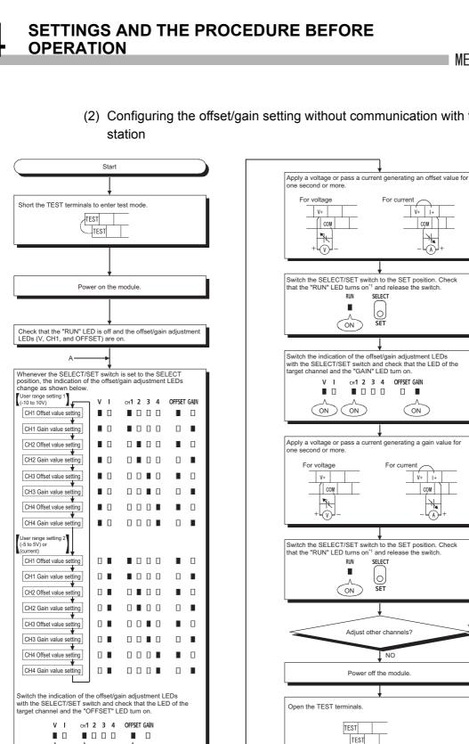
(2) Configuring the offset/gain setting without communication with the master
