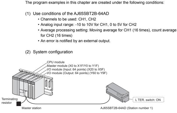
Figure 5.2 System configuration and wiring diagram
