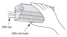
Figure 4.2 Mounting a module to a DIN rail
