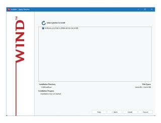
**3.** Check that the checkbox of a patch to be installed is selected, and click the [Install] button.
