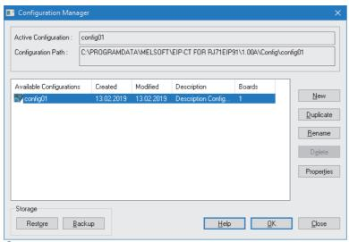
**2.** Click the [Restore] button to import the setting file to EtherNet/IP Configuration Tool.
