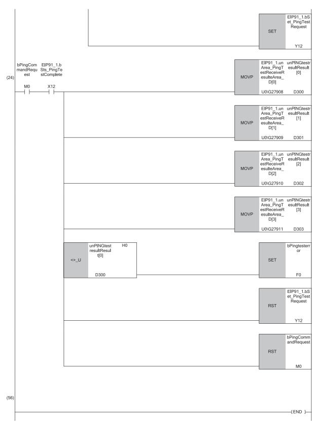
(0) PING test request processing (24)PING test response processing
