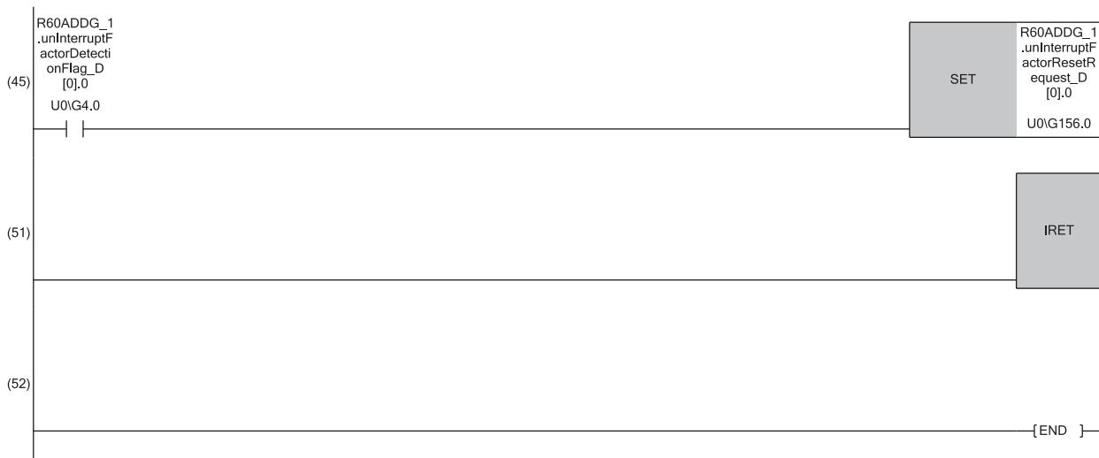
(45) Turn on 'Interrupt factor reset request [1]' (U0\G156) when 'Interrupt factor detection flag [1]' (U0\G4) turns on.
