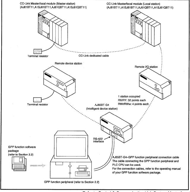
Refer to Control & Communication Link System Master/Local Module User's Manual for the maximum distance of the total system extension.
