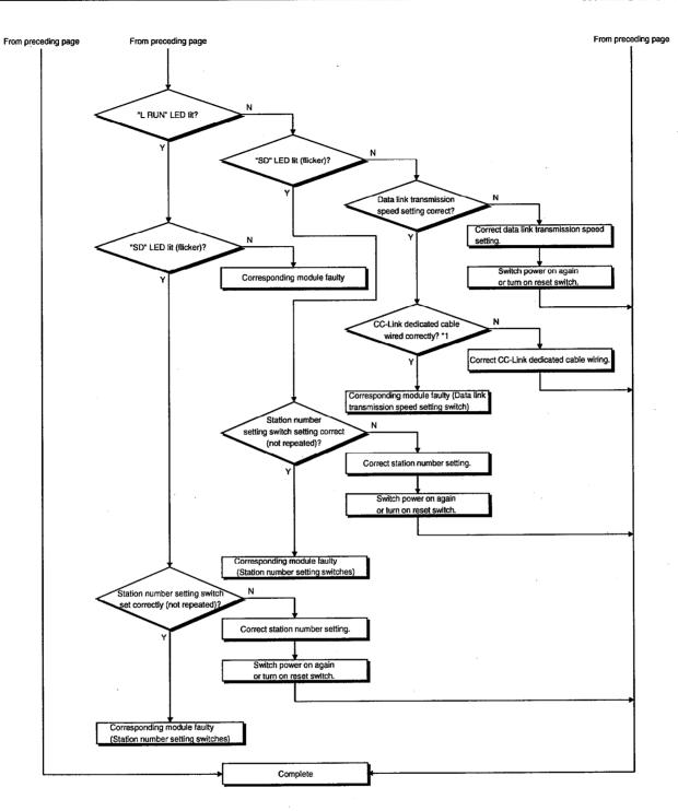
\*1: Check for short circuit, reverse connection, wire breakage, no terminal resistor, improper FG connection, improper overall distance and improper interstation distance.
