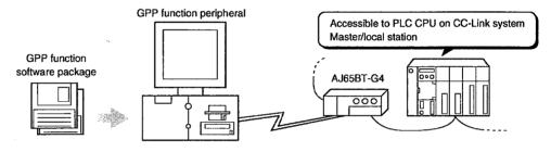
(b) If the Master and Local stations of the CC-Link system are incorporated in the MELSECNET/10 system, the GPP functions are accessible to other station PLCs on the network when the AJ65BT-G4 is operating in the QnA mode. (If the PLC CPUs on the midway station and access destination are the MELSEC-QnA series)
