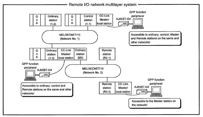
(c) If the Master and Local stations in the CC-Link system are incorporated in the MELSECNET(II) system, the GPP functions can access other station PLCs in the data link when the AJ65BT-G4 is operating in the QnA mode. (If the PLC CPUs in the midway station and access destination are the MELSEC-QnA series)
