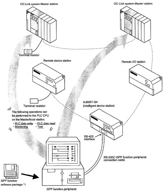
\*1: GPPW: GPP function software for Windows (SW2D5C/F-GPPW-E and above, hereafter referred to as the "GPPW") GPPQ: SWn-GPPQ type GPP function software package (hereafter referred to as the "GPPQ") GPPA: SWn-GPPA type GPP function software package (hereafter referred to as the "GPPA")
