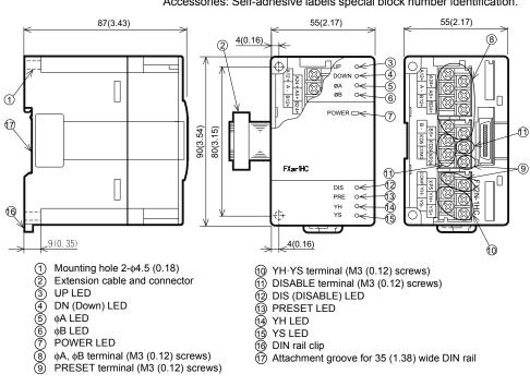
Mass (weight): Approx. 0.3 kg (0.66 lbs) Dimensions: mm (inches) Accessories: Self-adhesive labels special block number identification.
