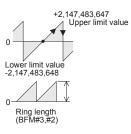
The counter mode is selected form the PLC. As shown below, values between K0 and K11 are written to buffer memory BFM #0 form the PLC. When a value is written to BFM #0 the contents of BFM #1 to BFM #31 are reset to default values. When setting this value use a TOP (pulsed) instruction use M8002 (initial pulse) to drive the TO
