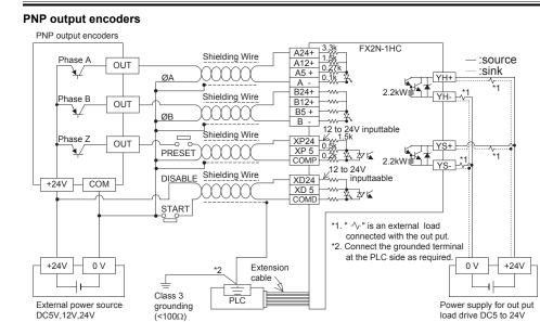
If using on NPN output encoder please take care to match the polarity of the terminals of the encoder to those of the FX2N-1HC.
