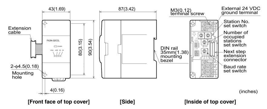
POWER LED: Lit when 5 VDC power is supplied from the PC main unit.
