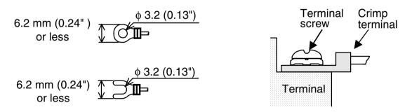
Handle the crimp terminal of the following size when 2 wires are used per terminal.
