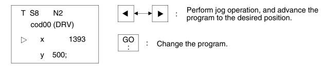
9) Move the cursor to the Y-axis address data. Perform jog operation.
