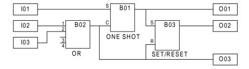
The input pins are shown on the left side of the FB and Outputs while output pins are shown on the right side of the blocks. Note that each input pin can receive only one signal but the output pins can provide signals to multiple sources.
