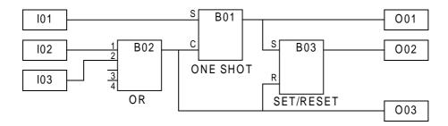
The base upon which the blocks are programmed is the Function Block Diagram (Fbd) base. A complete function block diagram is shown above, where I = Input and O = Output. The user can build a complex circuit in small easy steps by starting at the input and working forward in a logical manner. The Alpha will gather information, process that information, and provide control for the system.
