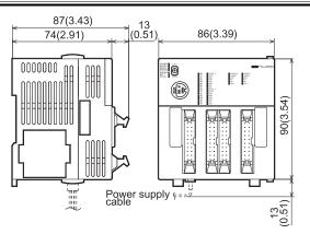
Din rail width: 35mm Weight: approx.0.4kg Dimensions mm(inch)
