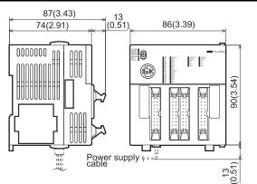
Din rail width: 35mm Weight: approx.0.4kg Dimensions mm(inch)
