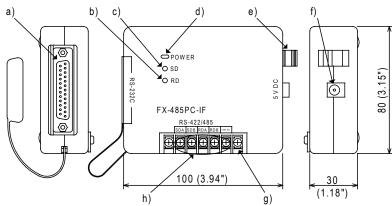
a) RS232C connector: Used for connection between 485PC-IF and computer.
