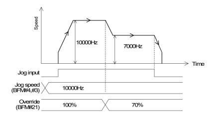
• According to the override setting (BFM#21), the actual operation speed is instructed or changed with the ratio in reference to the jog speed (BFM#4, #3).
