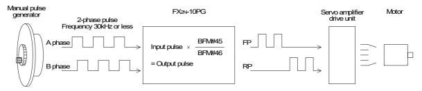
The output pulse (frequency and pulse amount) of FX2N-10PG is gained as follows:
