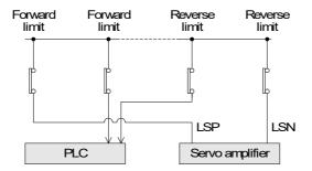
• Since such terminals are not provided on the drive amplifier for the stepping motor, be sure to provide the terminals in the PLC.
