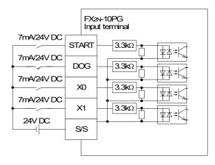
2) When NPN open collector transistors are used
