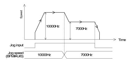
When speed change disable (BFM#26 b10) during operation is ON, the change of jog speed (BFM#4, #3) is not permitted.
