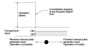
• The operation speed is proportional to the frequency of pulse chain input from the manual pulse generator with the electronic gearing (BFM#45, #46) for manual pulse generator input.
