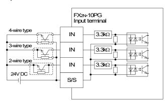
Reread IN terminal as START, DOG, X0 or X1 according to the application.
