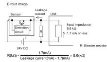
The power capacity W of the bleeder resistor R is as follows W =  $\frac{(\text{Input voltage})^2}{(\text{Input voltage})^2}$
