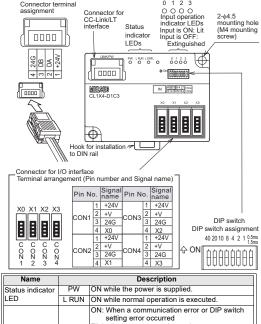
Flickering at a constant interval: When the setting of the DIP switch was changed
