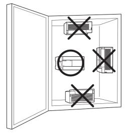
• Arrange the extension cable in such a way that the left connectors of the I/O extension units/blocks or special extension units/blocks are connected on the side closer to the main unit.
