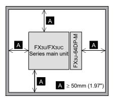
• To prevent temperature rise, do not install the PLC on a floor or a ceiling or in the vertical direction. Install it horizontally on a wall as shown below.
