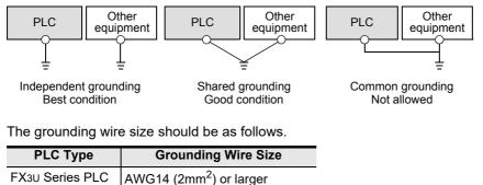
The grounding point should be close to the PLC, and all grounding wire should be as short as possible.
