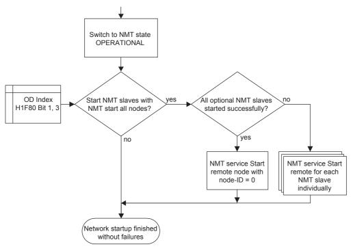
Figure 5.2: NMT Master simple startup
