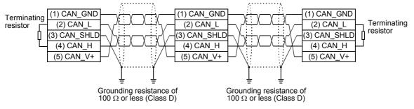
For electromagnetic compatibility (EMC), it is recommended to ground the cable shield at both ends.
