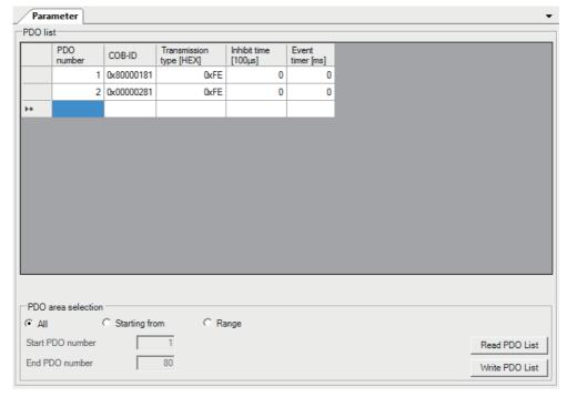
"Navigator"  $\rightarrow$  "CANopen Configuration"  $\rightarrow$  Node name  $\rightarrow$  "Receive PDO"
