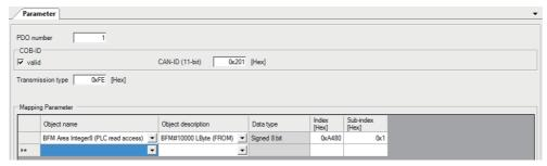
4) In the "NMT master / slave" window, set parameters for the NMT master and NMT slaves.
