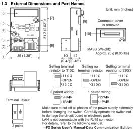
[1] Terminal block to connect ground [6] Connector cover
