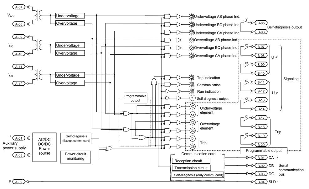
Figure 5.2 Internal function block diagram of Type CBV2-A01D1 relay
