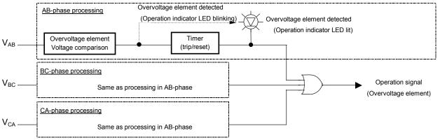
Figure 4.2 Overvoltage element internal function diagram
