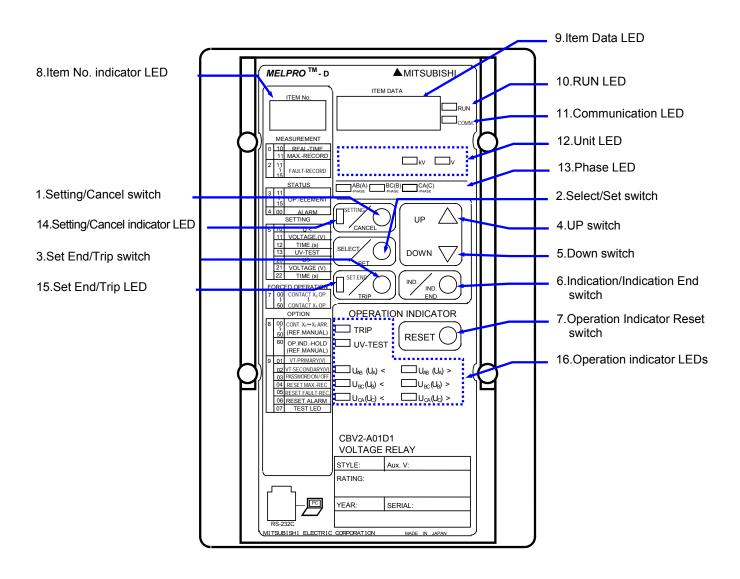
Figure 6.2 Front view of type CBV2-A01D1 relay
