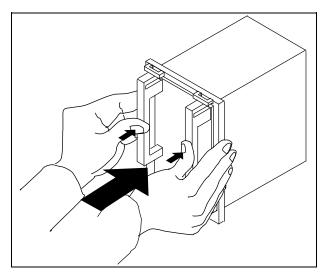
Fully insert the sub unit into the case until you hear a click while pressing the handles located on both sides of the front of the sub unit, and also the front face of subunit (ie, 4 corners of front face) is becoming flush with the vertical surface of the case.
