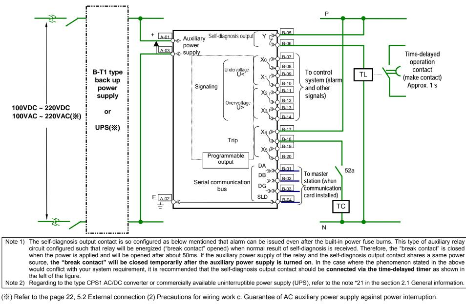
Figure 5.5 Auxiliary power supply circuit connection example of type CBV2-A01D1 relay
