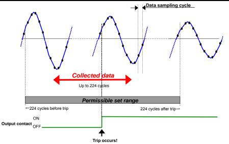
Figure 4.4 Concept of recording fault waveform
