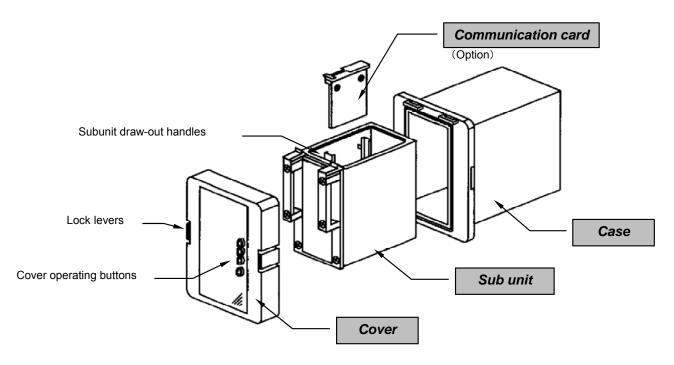
Figure 6.1 Outside view of type CBV2-A01D1 relay
