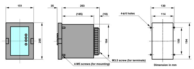
Figure 7.1 Outside dimension /drilling drawing
