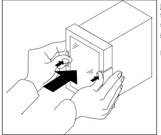
Fit the cover straight to the case. Hold the cover frame to fully push the lock levers, located both side of the cover, to case side <u>until it is clicked</u> and locked.
