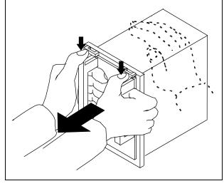
Grip the draw-out handles (located at both sides of the front of the sub unit). <u>Press the locking pieces</u> <u>installed in the upper portion of the draw-out</u> <u>handles with your thumbs to pull the sub unit</u> <u>towards you</u>.
