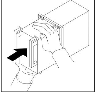
Hold the sub unit on the top and bottom to push the unit into the case approx. a half of the unit.
