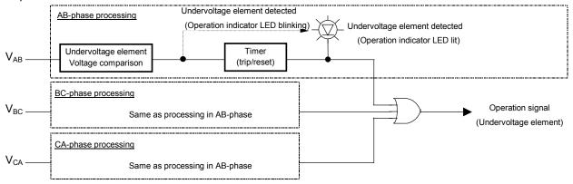
Figure 4.1 Undervoltage element internal function diagram
