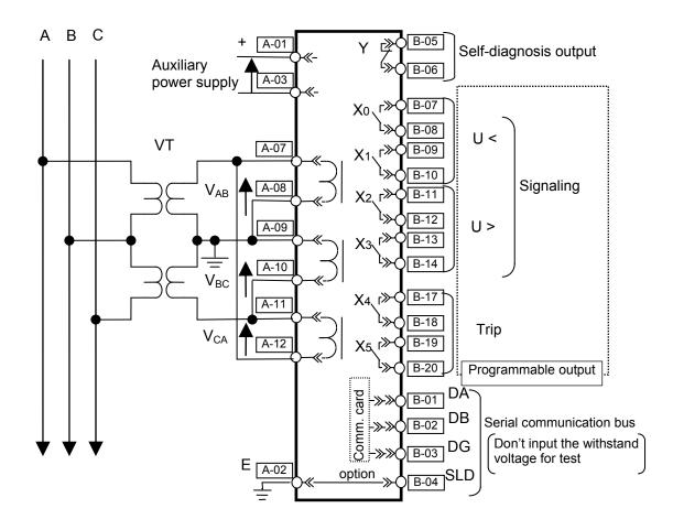
Figure 5.4 External connection diagram for CBV2-A01D1 relay
