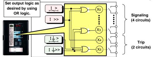
Figure 4.3 Schematic image of Programmable Outputs (example: COC4-A01)
