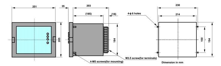
Figure 7.1 Outside dimension /drilling drawing (D2 Case)
