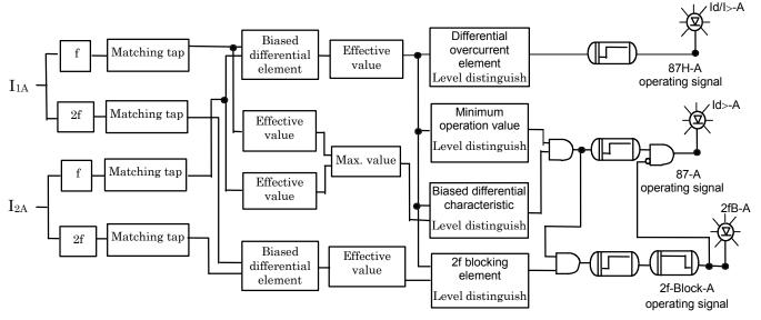
Figure 4.1 Biased differential element • Differential overcurrent element Internal function diagram (Only one phase expressed)
