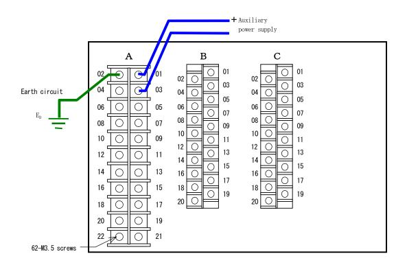
Figure 5.10 Rear view of type CAC1-A01D2 relay
