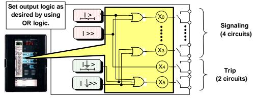
Figure 4.4 Schematic image of Programmable Outputs (example: COC4-A01D1)
