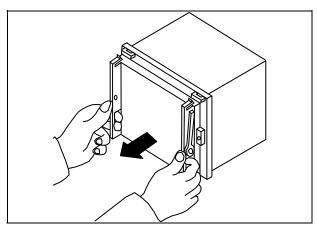
Grip the draw-out handles (located at both sides of the front of the sub unit), and **pull the sub unit towards you** until about a half portion of the sub unit is pulled out of the case.
