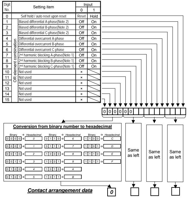
When the product is shipped from the factory, contact arrangement data are set as follows.
