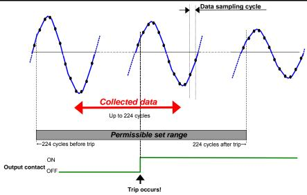
Figure 4.5 Recording concept of fault waveform
