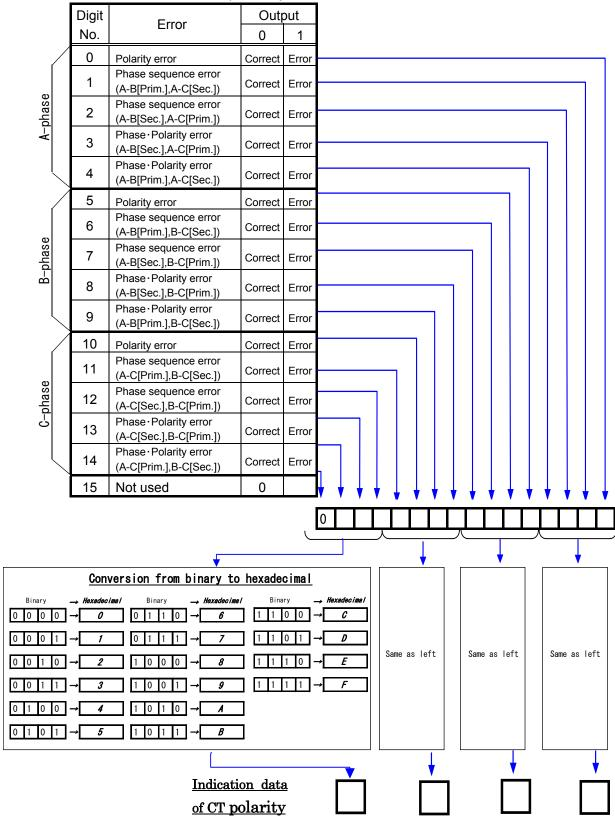
How to read and understand the CT polarity check codes
