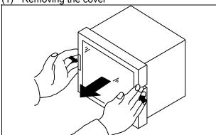
Hold the <u>lock levers</u>, which are located at both sides of the cover, on their front sections. Take off the cover <u>straight toward you</u> while pushing the levers <u>inwards</u>.
