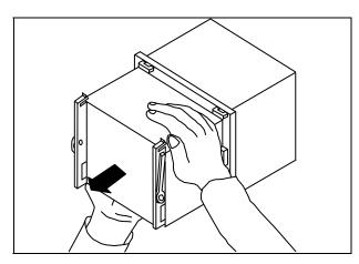
When about a half portion of the sub unit is pulled out of the case, just stop the drawing motion. Then, hold the top and bottom of the sub unit to pull it out completely, in order to prevent the unit from falling.
