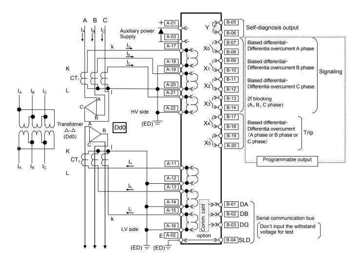
CT secondary circuit should be connected so as HV side current to be inflow to the Ry terminal of HV side and LV side current to be out flow from the Ry terminal of LVside with keeping same phase angle between bothside, when flow –through current is placed.
