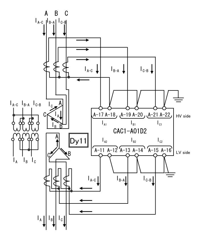
CT secondary circuit should be connected so as HV side current to be inflow to the Ry terminal of HV side and LV side current to be out flow from the Ry terminal of LVside with keeping same phase angle between bothside, when flow –through current is placed.
