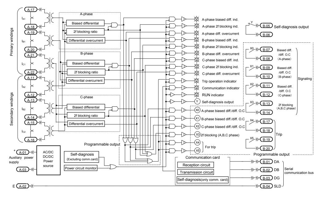
Figure 5.2 Internal function block diagram of type CAC1-A01D2
