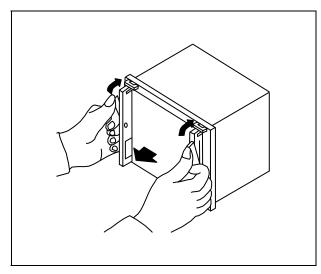
With the draw-out auxiliary levers touching the metallic parts, exert your strength to turn round the levers continuously, the sub unit will be drawn out a little from the case.
