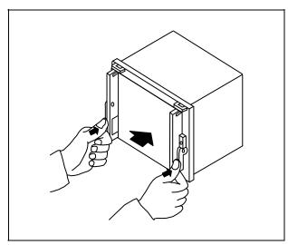
Exert your strength to press the lower parts of the auxiliary levers to fully insert the sub unit into the case until you hear a click.
