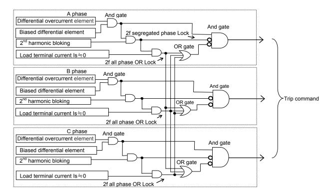
Figure 4.3 Load terminal current Is=1/2×setting value of biased differential element 17
