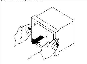
Hold the <u>lock levers</u>, which are located at both sides of the cover, on their front sections. Take off the cover <u>straight toward you</u> while pushing the levers <u>inwards</u>.
