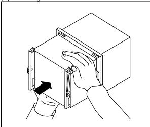
Hold the sub unit on the top and bottom to push the unit into the case approx. a half of the unit.
