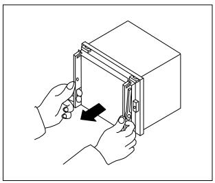
Grip the draw-out handles (located at both sides of the front of the sub unit), and **pull the sub unit towards you** until about a half portion of the sub unit is pulled out of the case.
