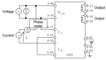
The current value measured by this test circuit is expressed as I.
