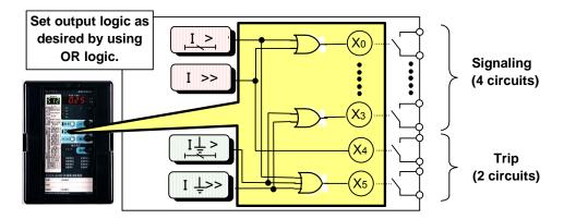
Figure 4-13 Schematic image of Programmable Outputs (example: COC4-A01)
