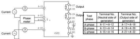
(3) Biased differential element (phase characteristics test)
