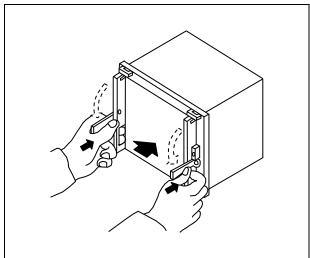
More fully insert the sub unit into the case until the auxiliary levers fall down automatically and catch the metal holes inside with its hooks.
