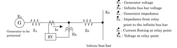
Figure 4-5 System diagram
