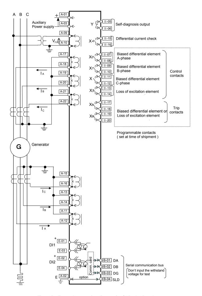
Figure 5-4 External connection diagram for CGP2-A01D2 relay
