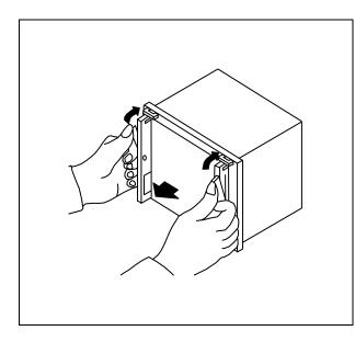
With the draw-out auxiliary levers touching the metallic parts, <u>exert your strength to turn round</u> <u>the levers</u> continuously, the sub unit will be drawn out a little from the case.
