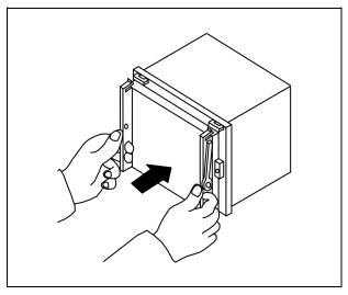
Under holding the auxiliary levers locked status by the with-holder (not to let the draw-out auxiliary levers fall down), Insert the sub unit into the case until the auxiliary levers touch the metallic parts while pressing the handles located on both sides of the front of the sub unit.
