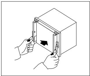
Exert your strength to press the lower parts of the auxiliary levers to fully insert the sub unit into the case until you hear a click.
