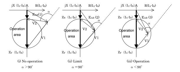
Figure 4-9 Operating principle (phase discriminating principle)
