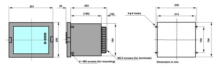
Figure 7-1 Outside dimension /drilling drawing
