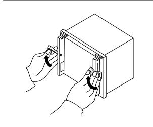
Please from under to upper direction turn round the draw-out auxiliary levers located on both sides of the front of the sub unit until the levers touch the metallic parts located on both sides of draw-out handles completely.
