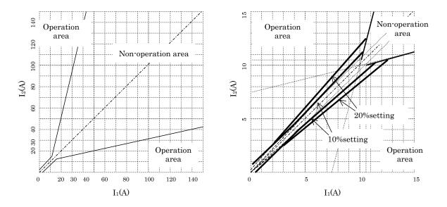
Figure 4-2 Biased differential characteristics between  $I_1$  and  $I_2$
