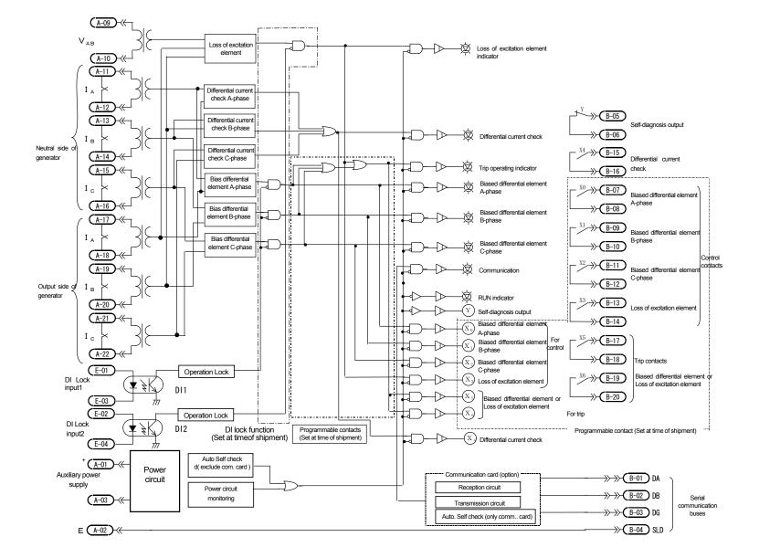
Figure 5-2 Internal function block diagram of Type CGP2-A01D2 relay
