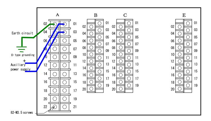
Figure 5-7 Rear view of type CGP2-A01D2 relay
