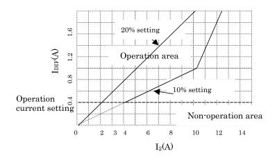
Figure 4-3 Biased differential characteristics between I<sub>2</sub> and I<sub>DIF</sub>
