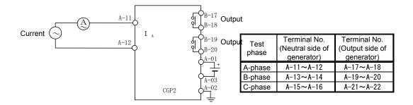
(2) Biased differential element (bias ratio characteristics test)
