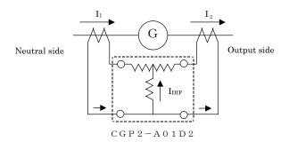
Figure 4-1 Operating principle
