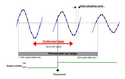
Figure 4-15 Concept of recording fault waveform
