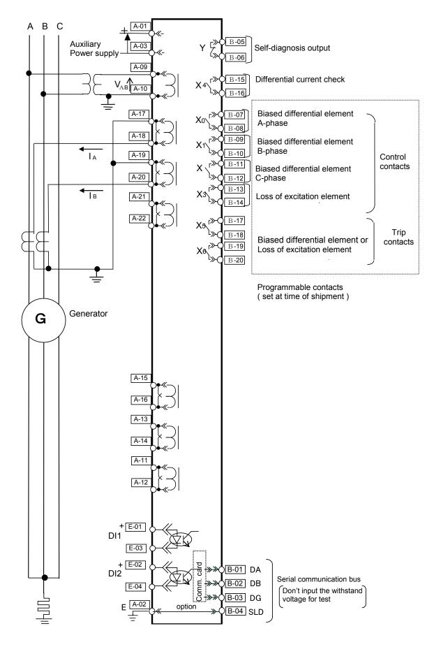
Figure 5-5 External connection diagram for CGP2-A01D2 relay (In the case of applying loss of excitation element alone)
