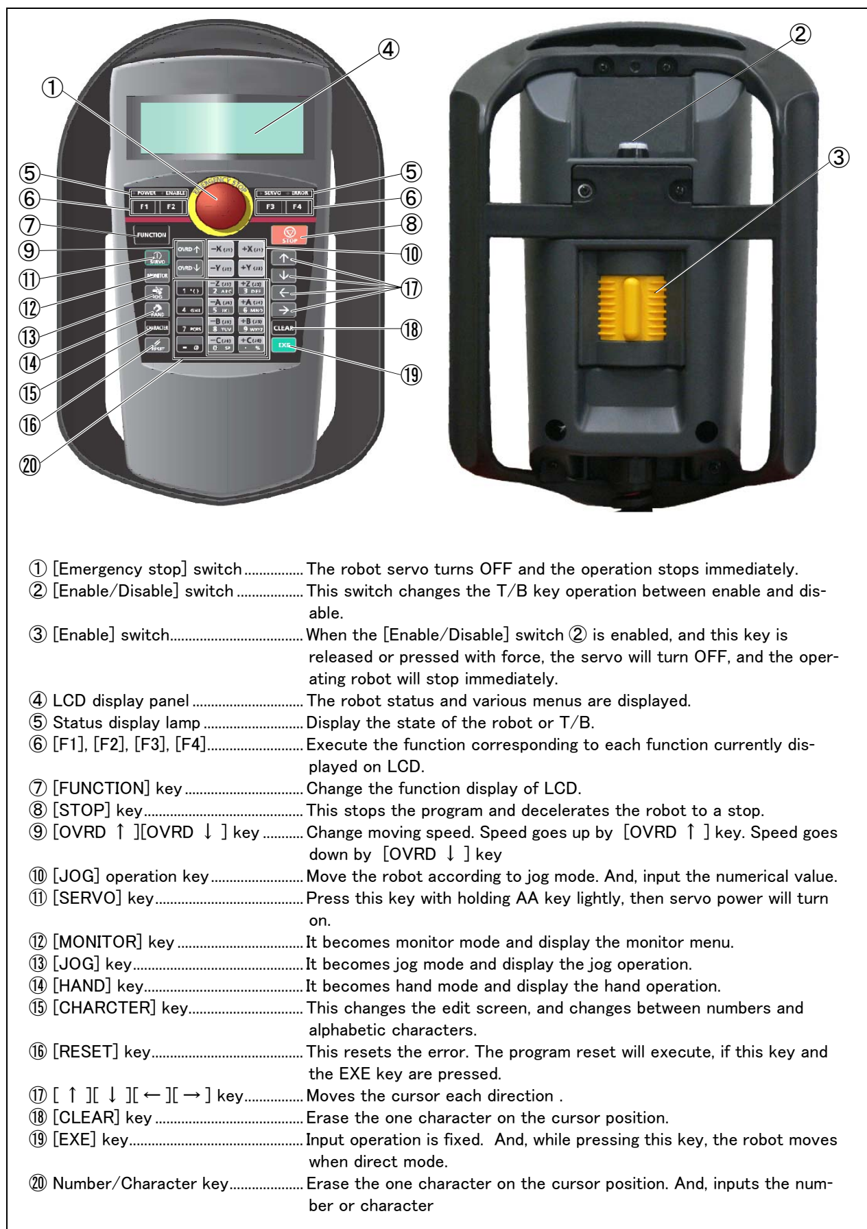
Fig.3-20 : Teaching pendant key layout and main functions
