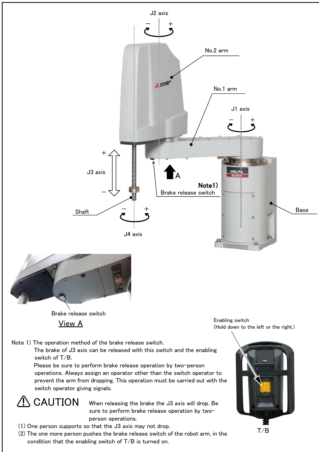
Fig.2-9 : Names of each part of the robot
