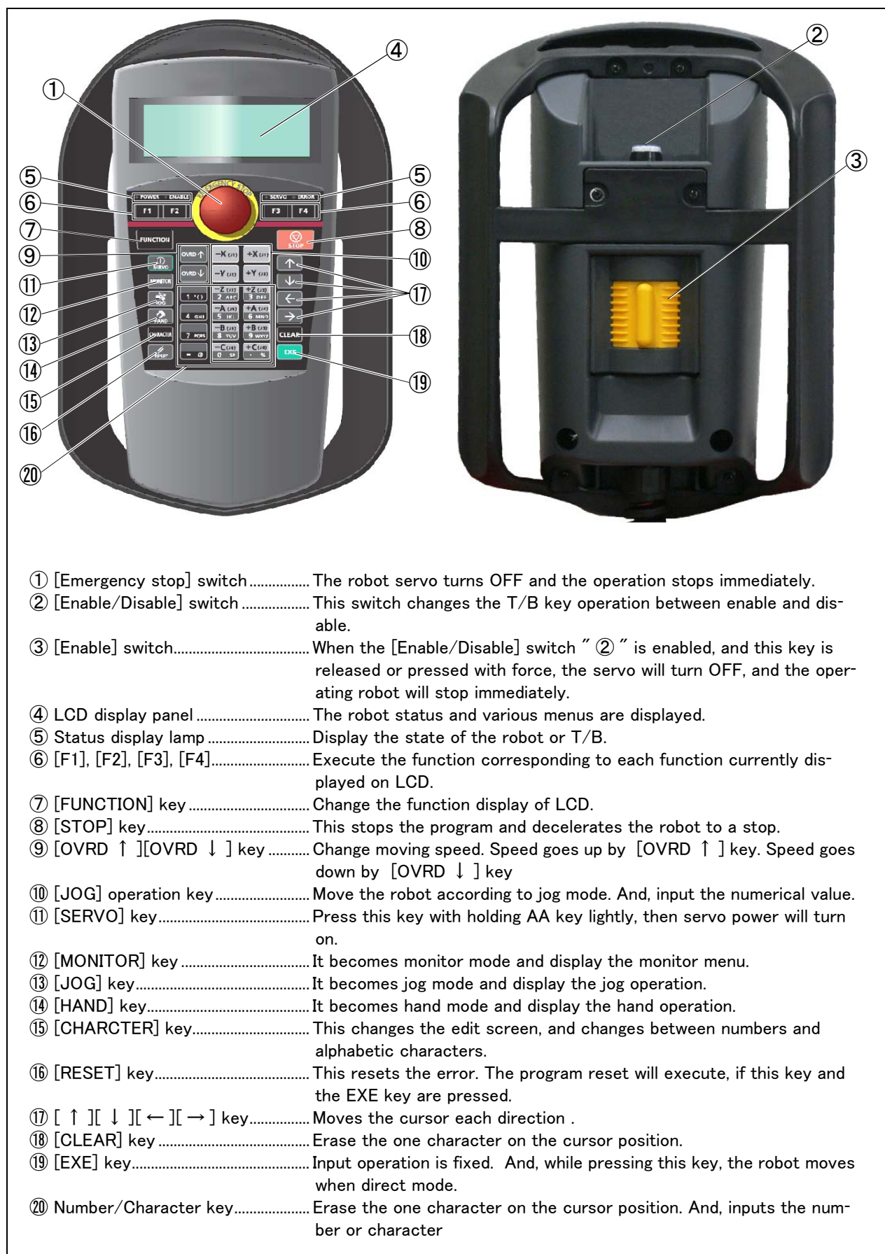
Fig.3-32 : Teaching pendant key layout and main functions
