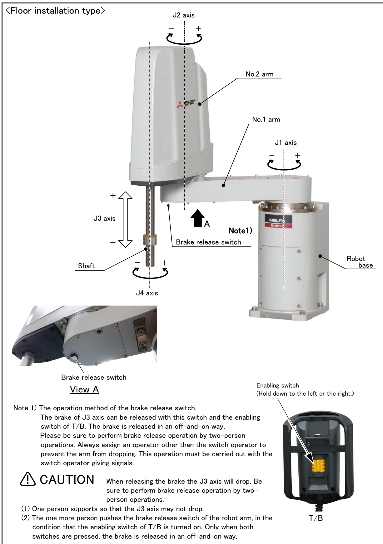
Fig.2-16 : Names of each part of the robot (Floor installation type)
