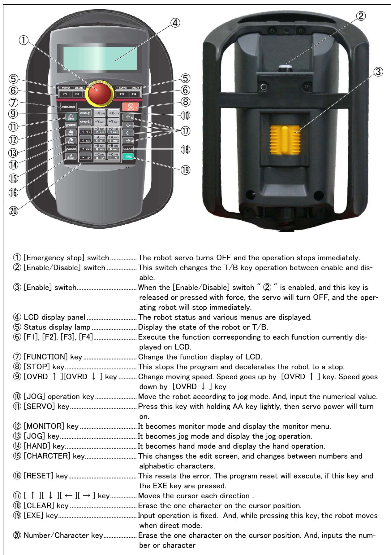
Fig.3-32 : Teaching pendant key layout and main functions
