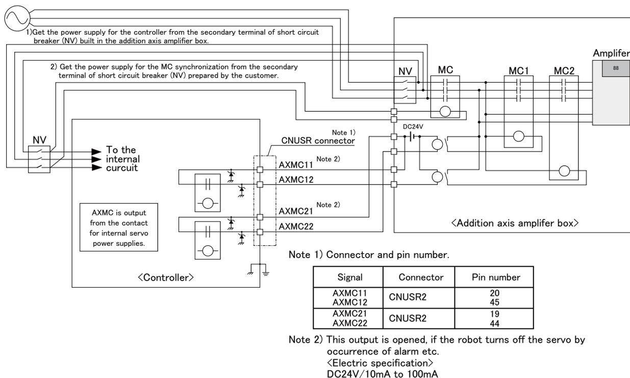
[Note] For the input/output cable (CNUSR connector cable) that connects customer's system and the controller, prevent ground faults from occurring at the + side of the 24V power supply prepared by customer. A ground fault may lead to a failure of the protection device in the controller.
