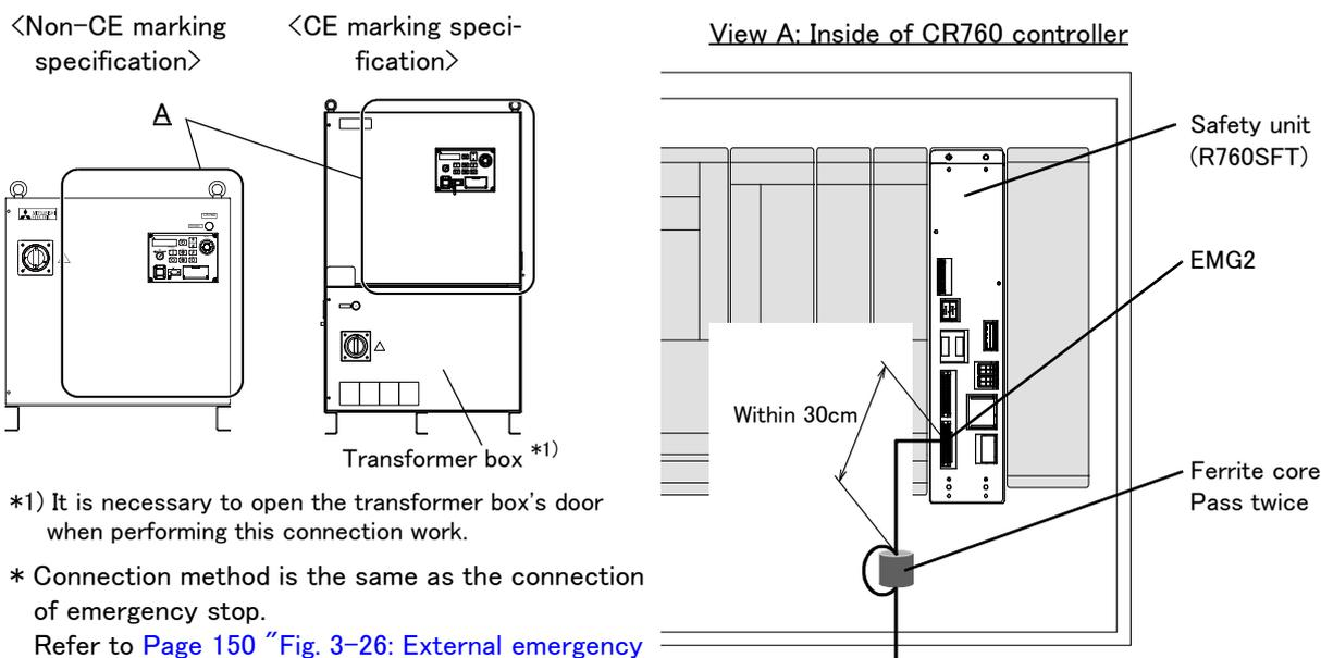
\*1) It is necessary to open the transformer box's door when performing this connection work.
