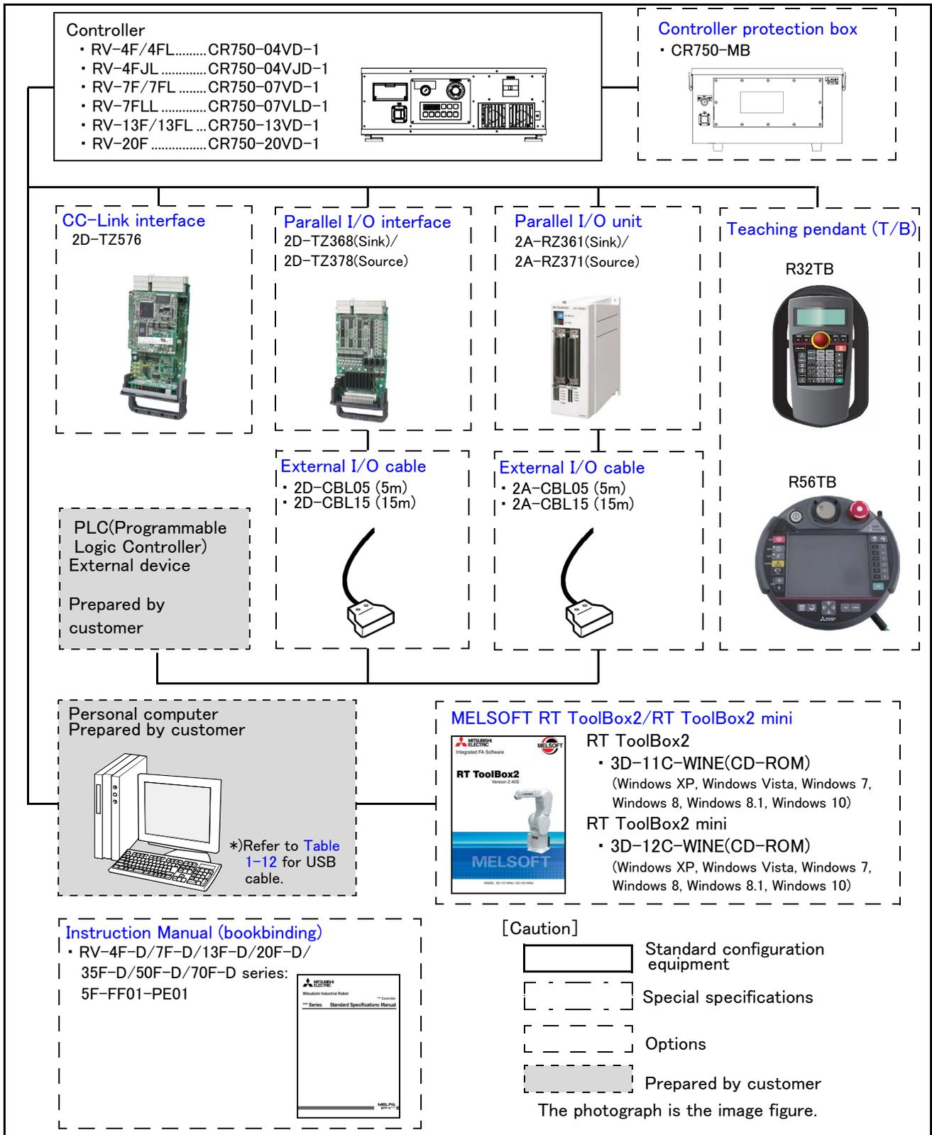
Fig.1-3 : Structural equipment (CR750 controller)
