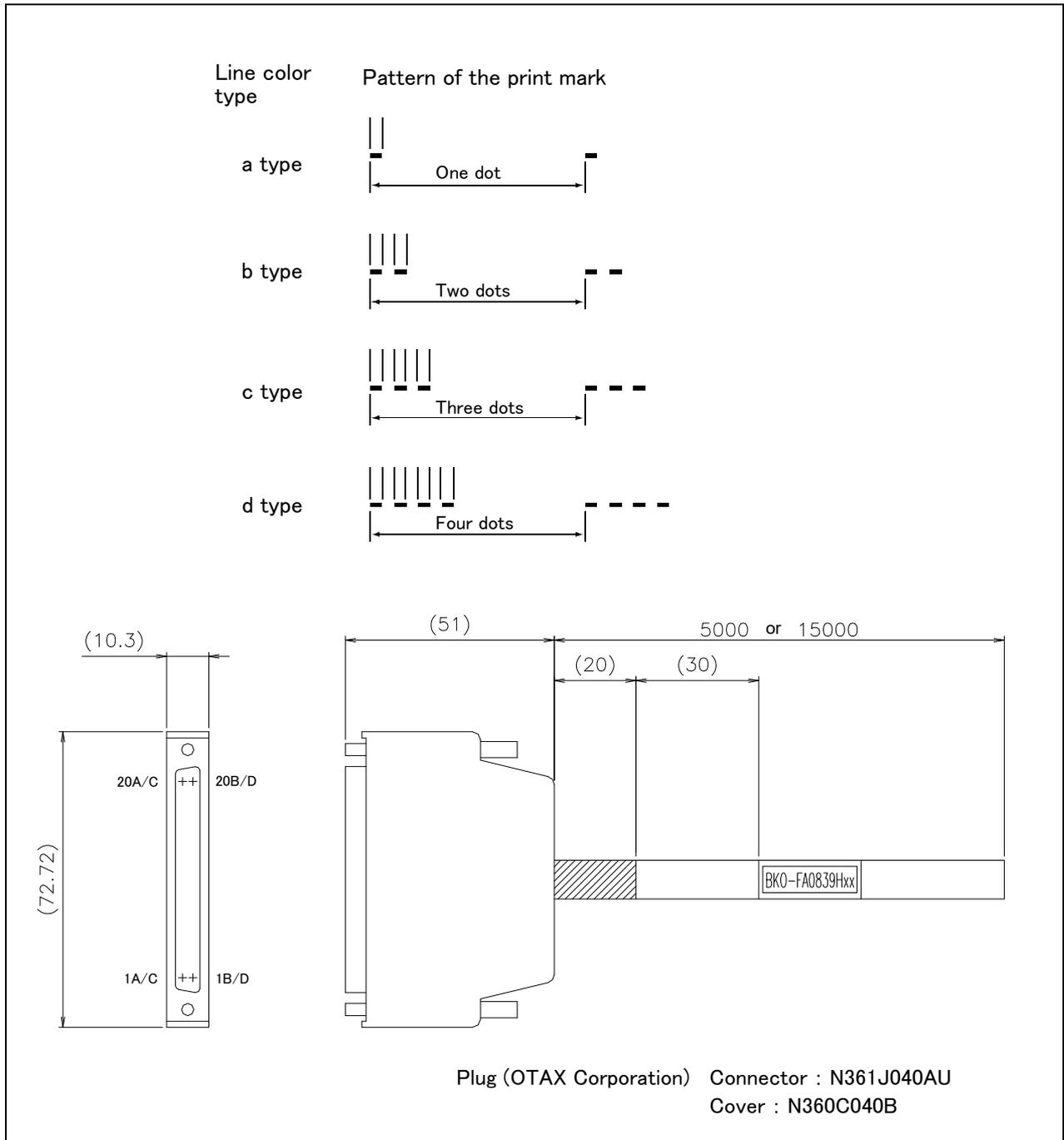
Fig.3-54 : Connections and outside dimensions
