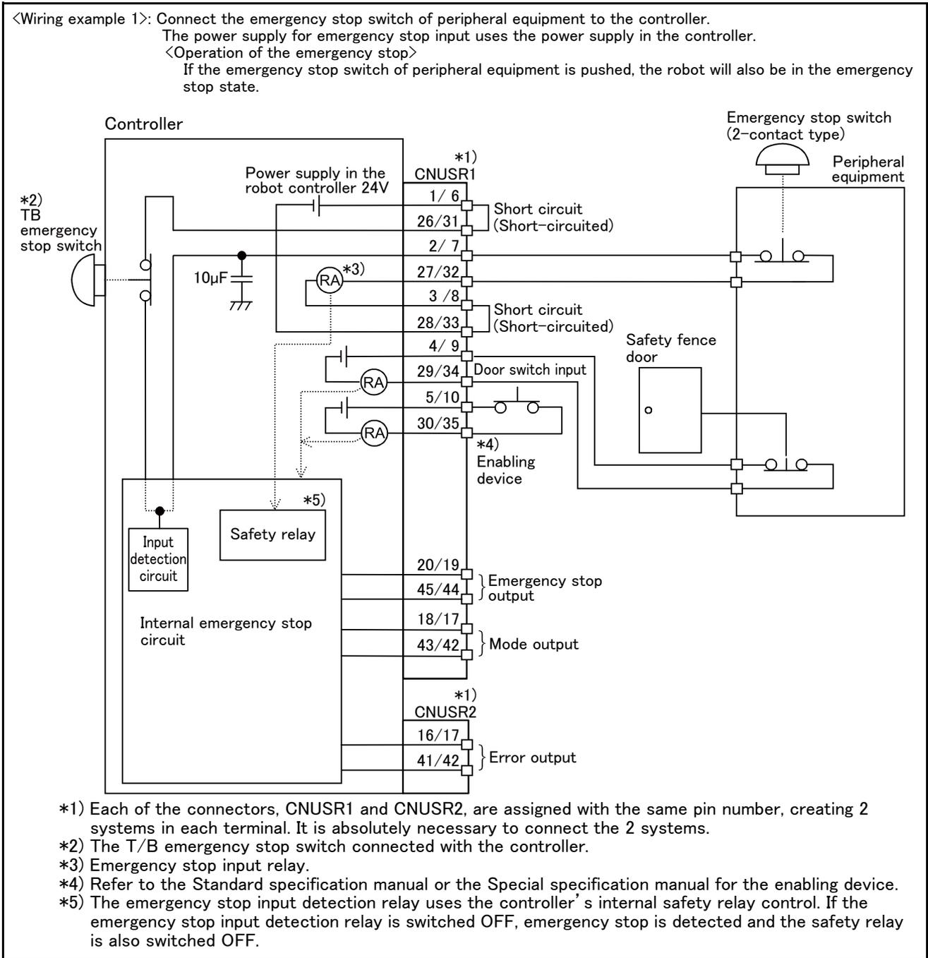
Fig.6-6 : Example of safety measures (CR751 wiring example 1)
