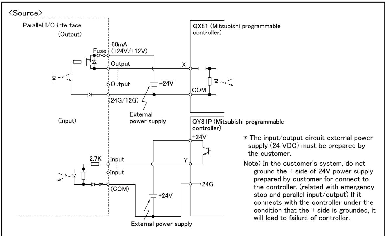
Fig.3-53 : Connection with a Mitsubishi PLC (Example of source type)
