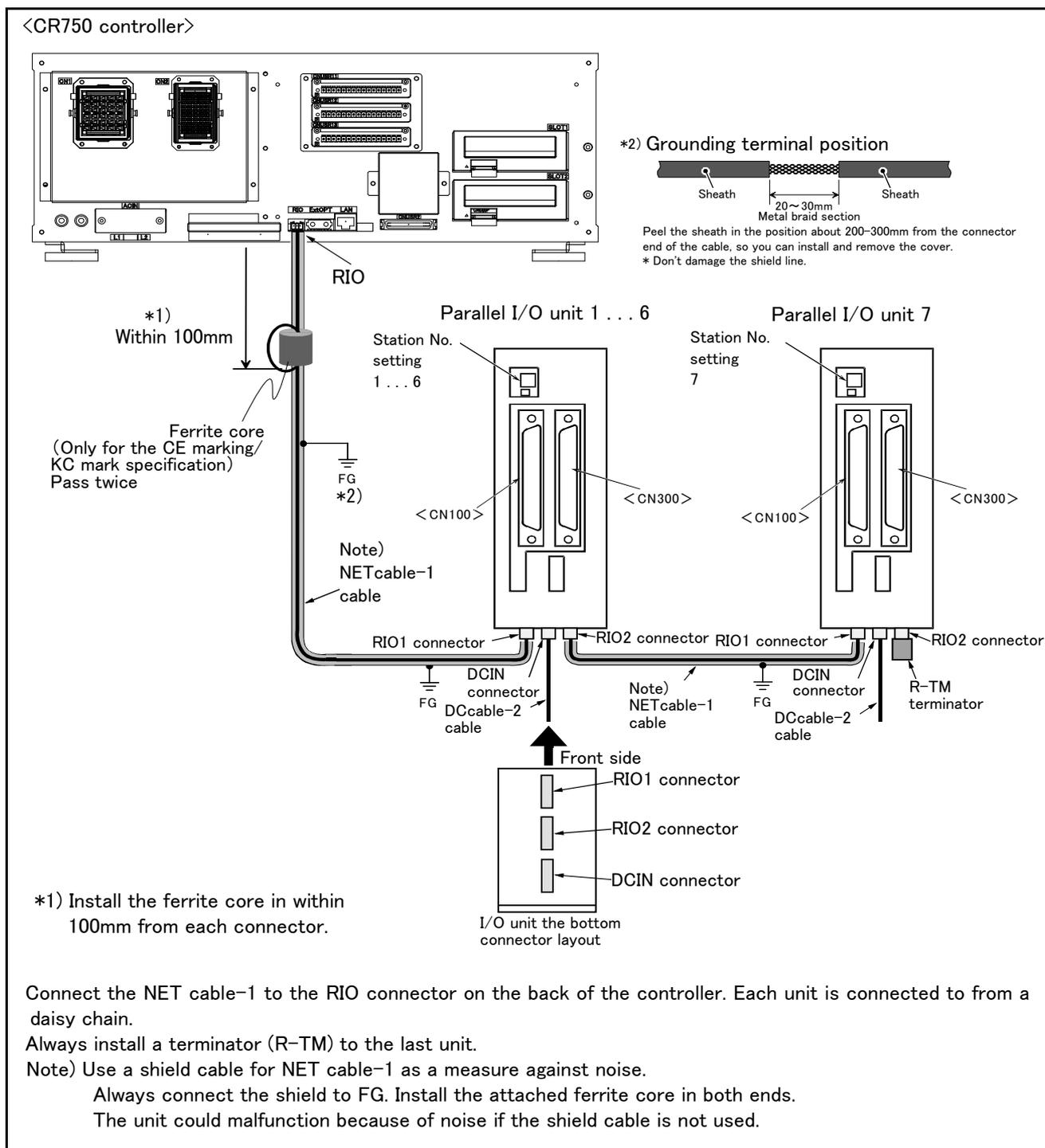
Fig.3-59 : Connection method of expansion parallel I/O unit (CR750)
