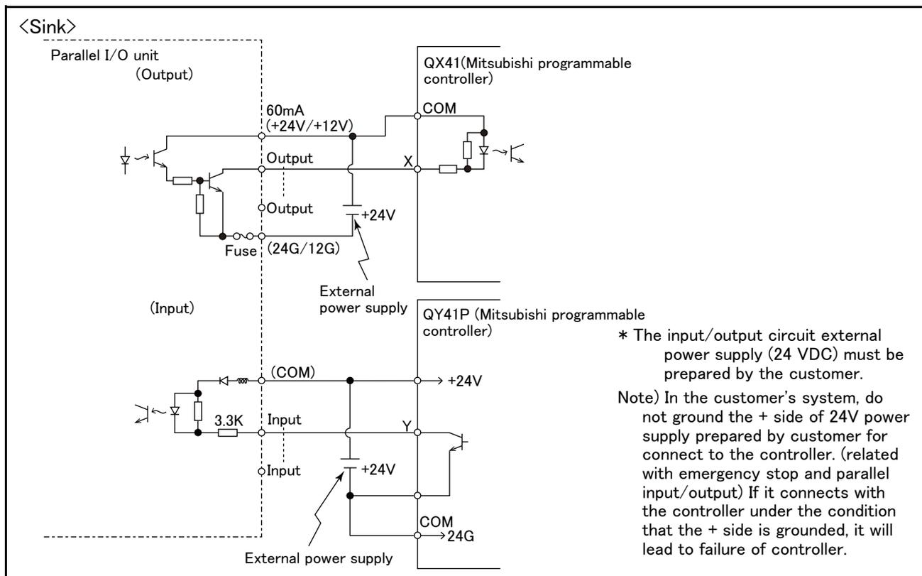
Fig.3-63 : Connection with a Mitsubishi PLC (Example of sink type)
