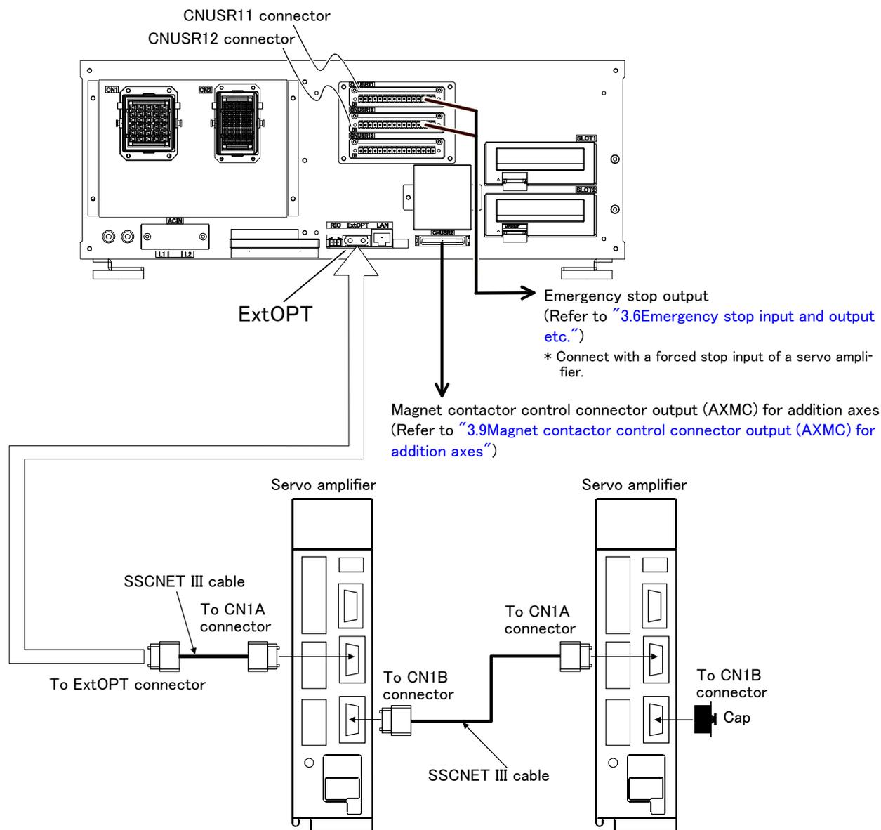
\* It cannot communicate, if connection of CN1A and CN1B is mistaken.
