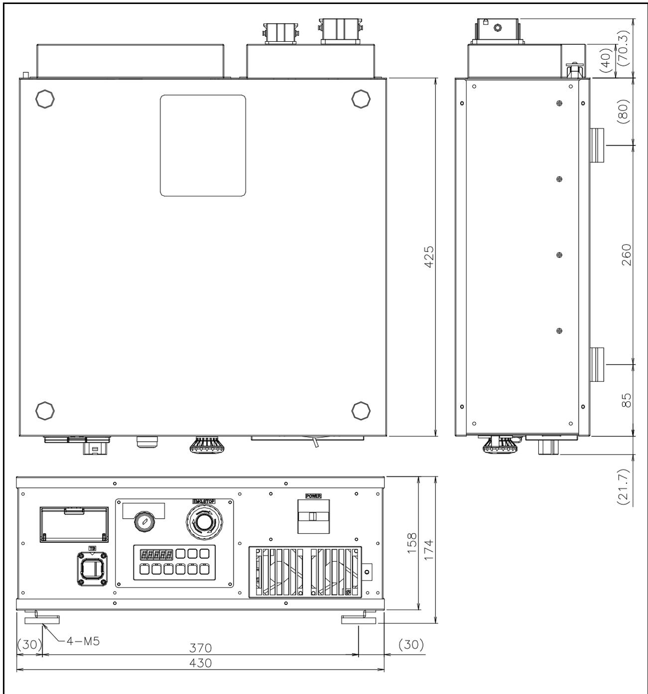
Fig.3-6 : Outside dimensions of controller (CR750)
