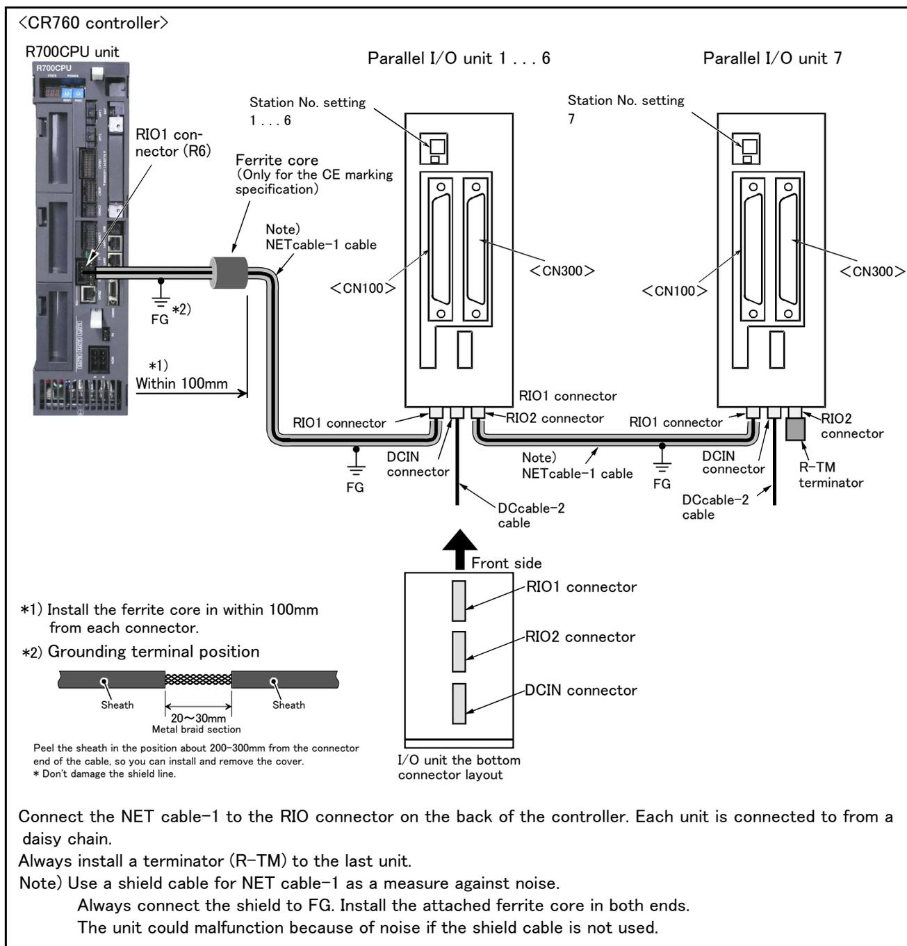
Fig.3-61 : Connection method of expansion parallel I/O unit (CR760)
