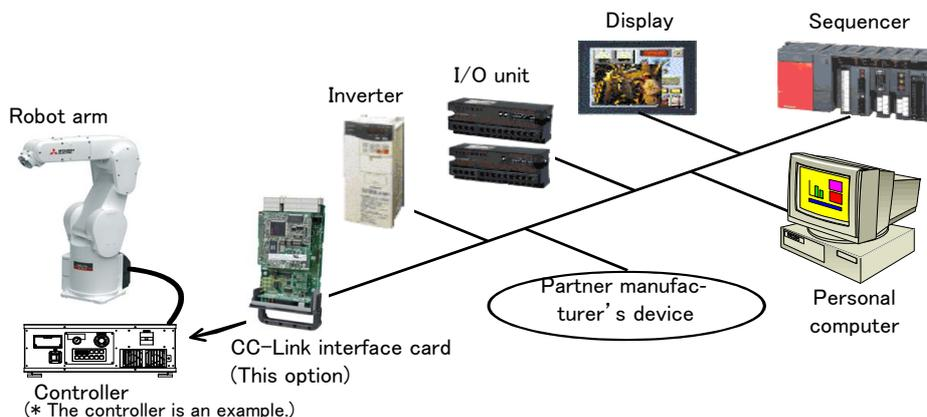
Fig.3-67 : Example of CC-Link Product Configuration
