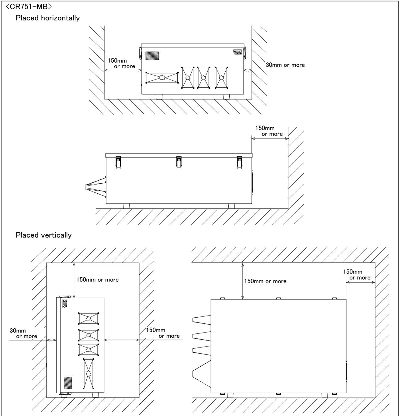
Fig.3-75 : Installation dimensions (CR751-MB)
