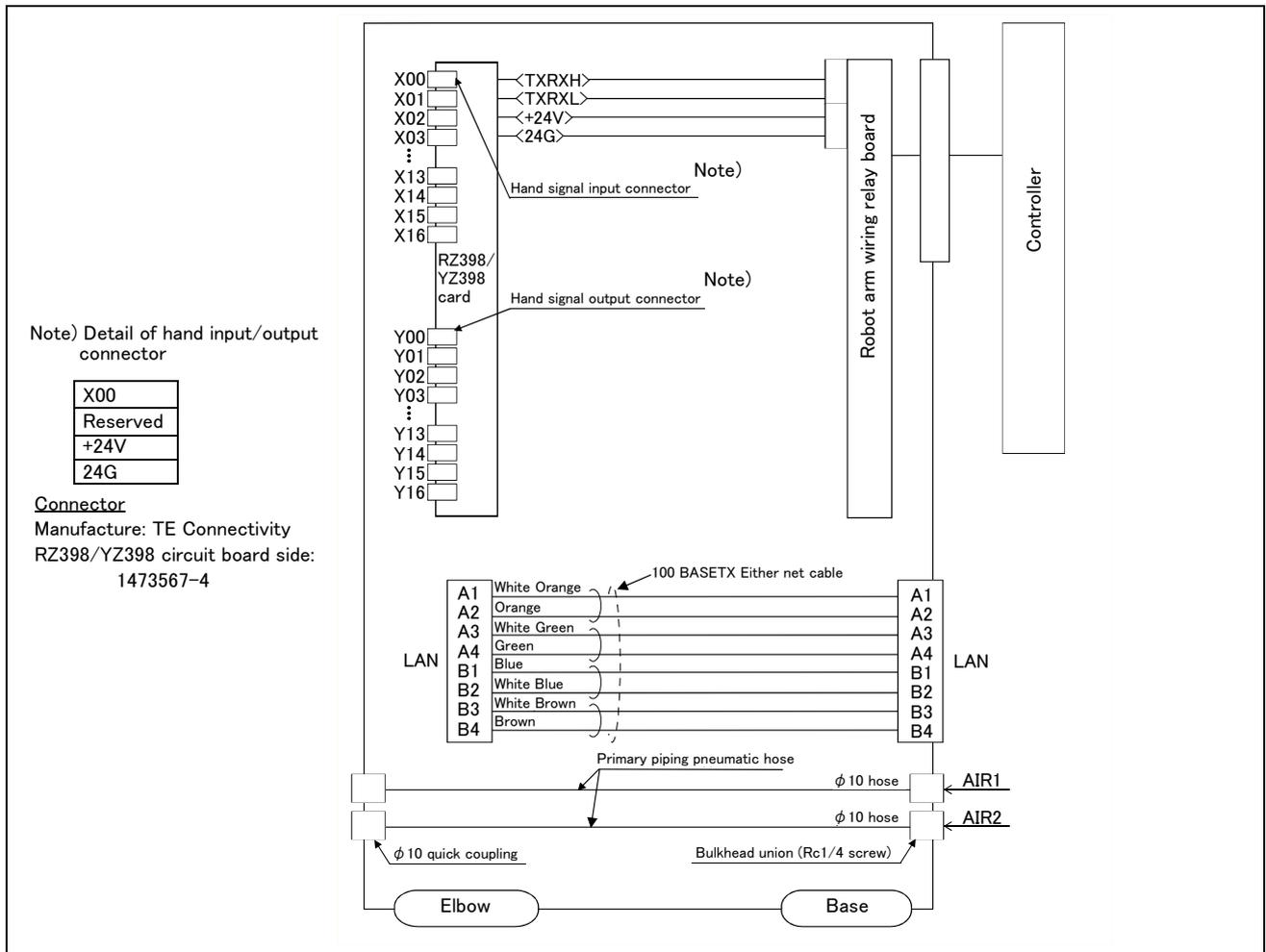
Fig.2-39: Wiring and piping system diagram for hand and example the solenoid valve installation: RV-35F/50F/70F series
