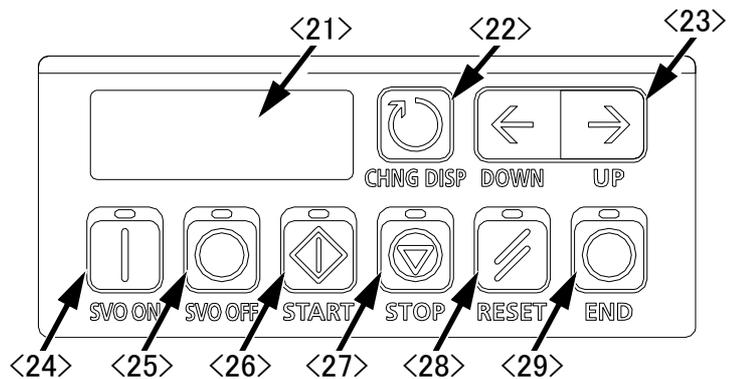
Fig.3-1 : Names of controller parts (CR750)
