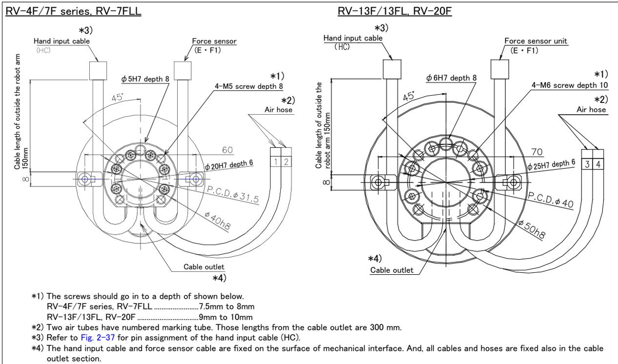
\* For details, refer to Page 65, "2.5.6 Wiring and piping system diagram for hand".
