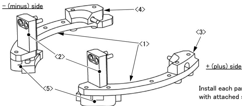
Install each parts to the upper arm lower part with attached screw.
