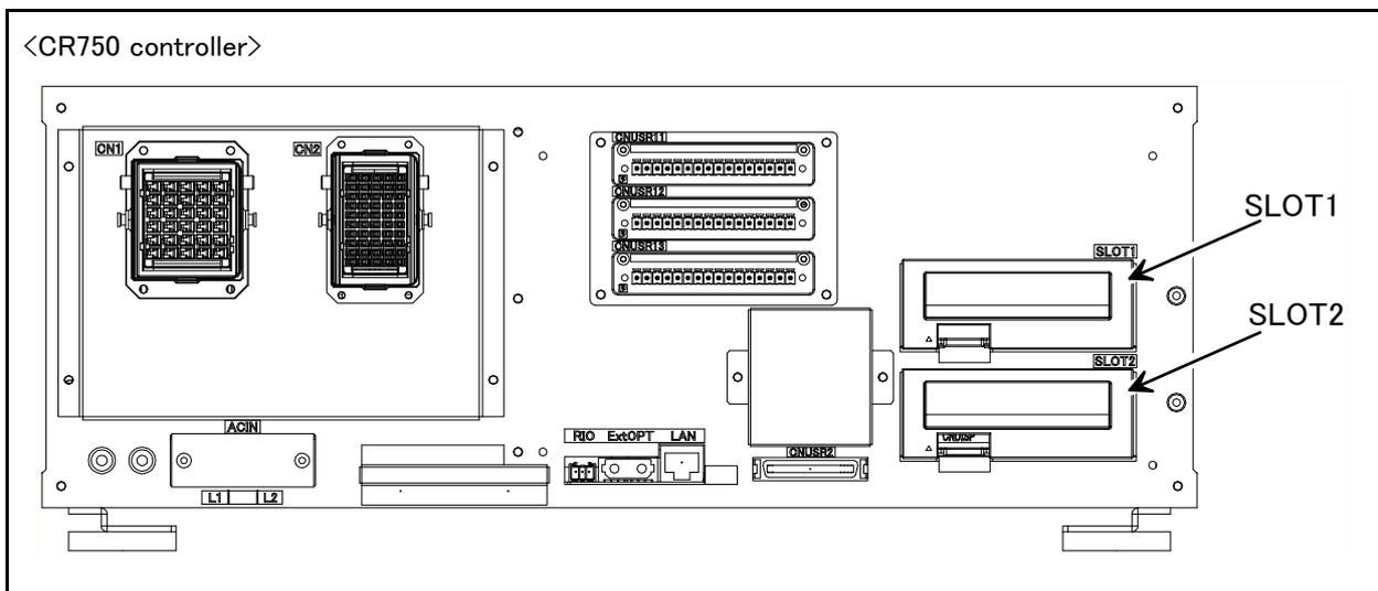
Fig.3-48 : Parallel I/O interface installation position (CR750)
