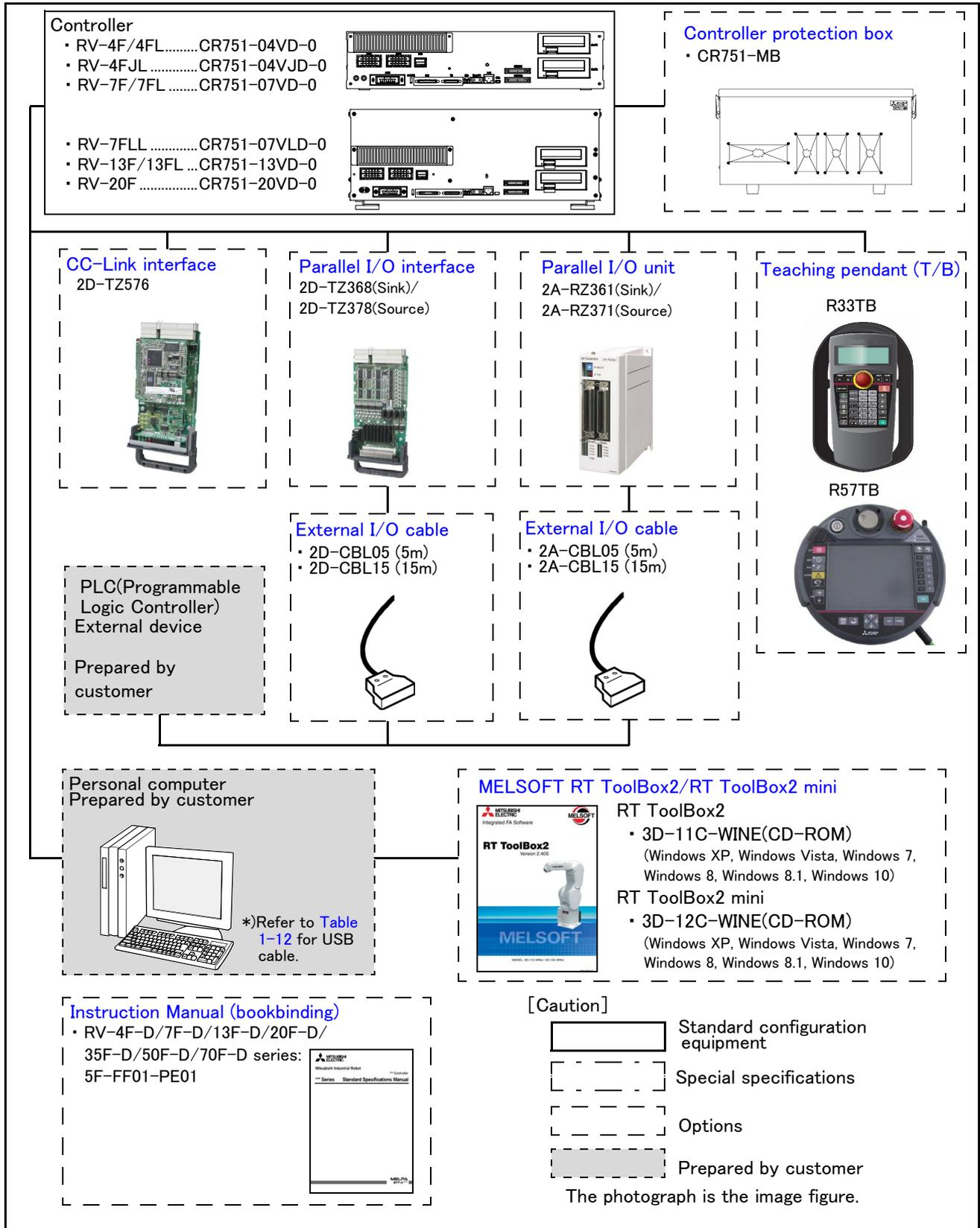
Fig.1-4 : Structural equipment (CR751 controller)
