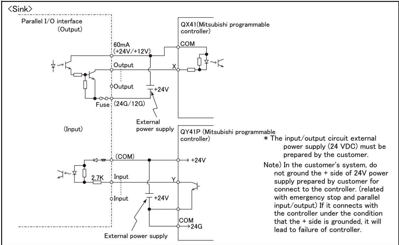
Fig.3-52 : Connection with a Mitsubishi PLC (Example of sink type)
