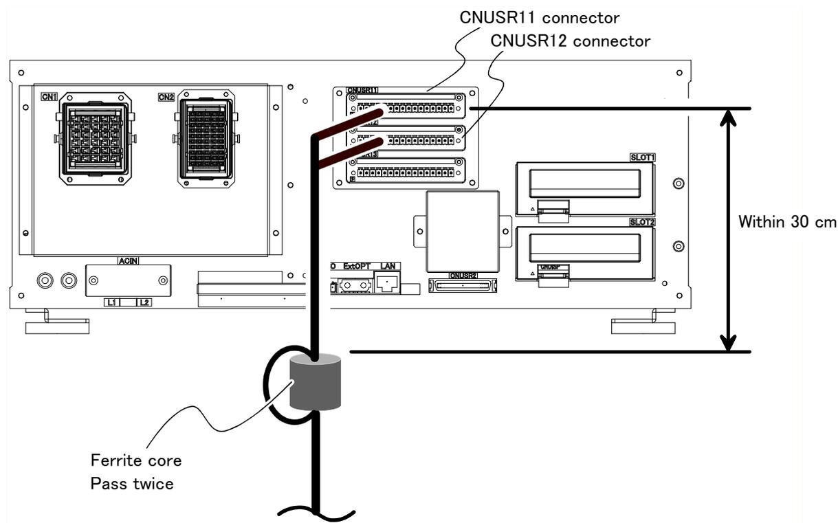
Fig.3-18 : Emergency stop cable connection (CR750)
