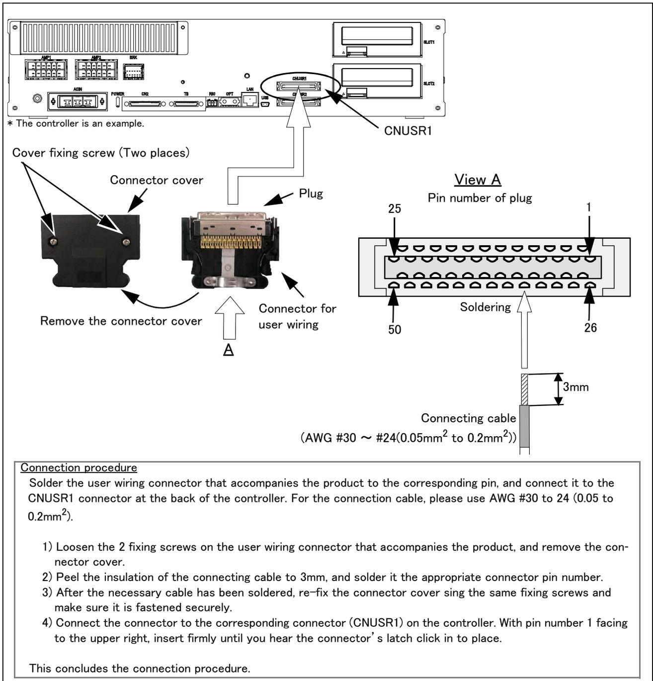
Fig.3-34 : Connection of the mode changeover switch input (CR751)
