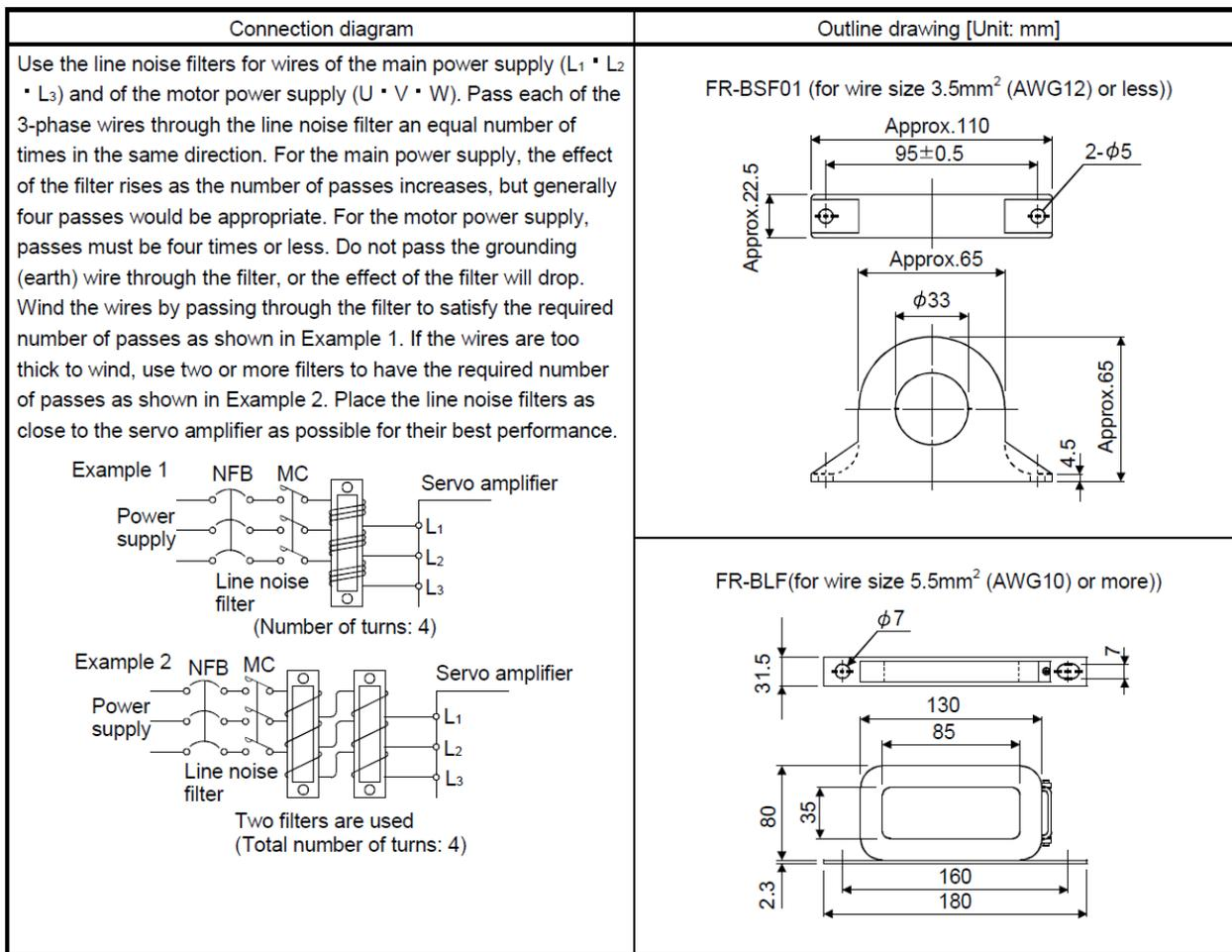
Fig.3-39 : Example of noise filter installation
