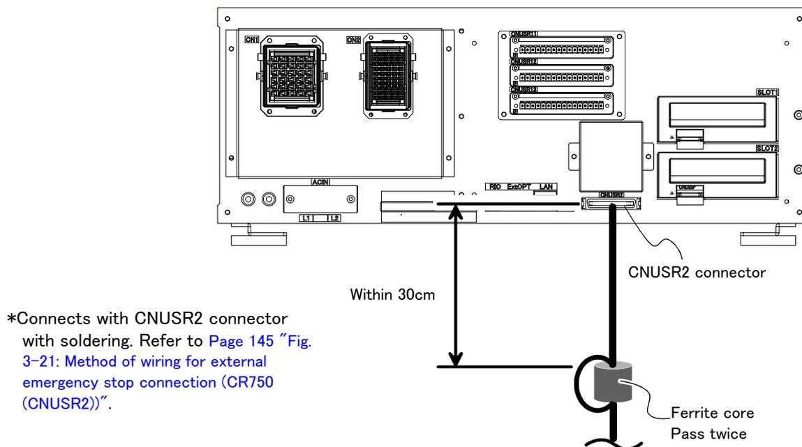
Fig.3-43 : AXMC terminal connector (CR750)
