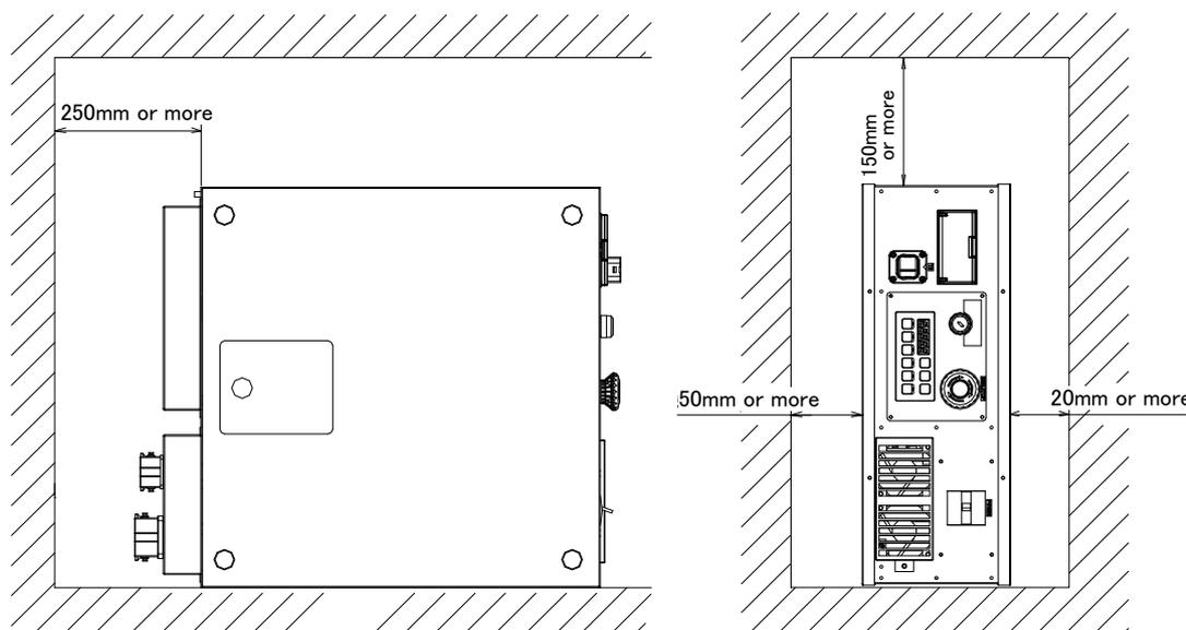
Fig.3-11 : Installation of controller (CR750)
