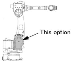
This cover protect the J2 axis motor from dust and water. Oil mist specification robot is equipped with the cover as standard.
