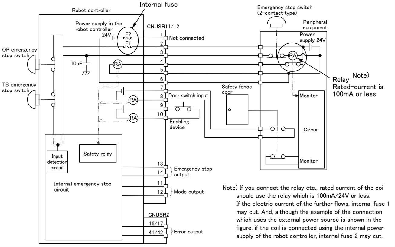
Fig.6-16 : Limitations when connecting the relay etc. (CR750)
