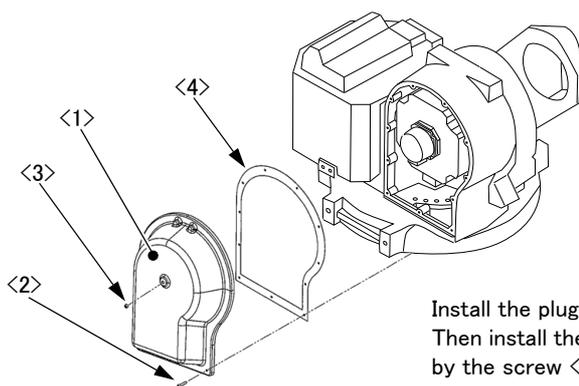
Install the plug with hole <3> to the cover <1>. Then install the cover <1> to the J2 motor portion of the robot arm by the screw <2> with the packing <4> in between.
