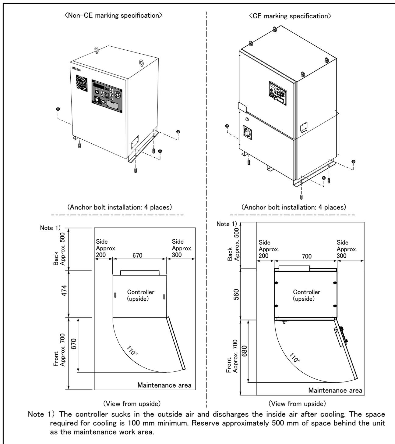
Fig.3-17 : Installation of controller (CR760)
