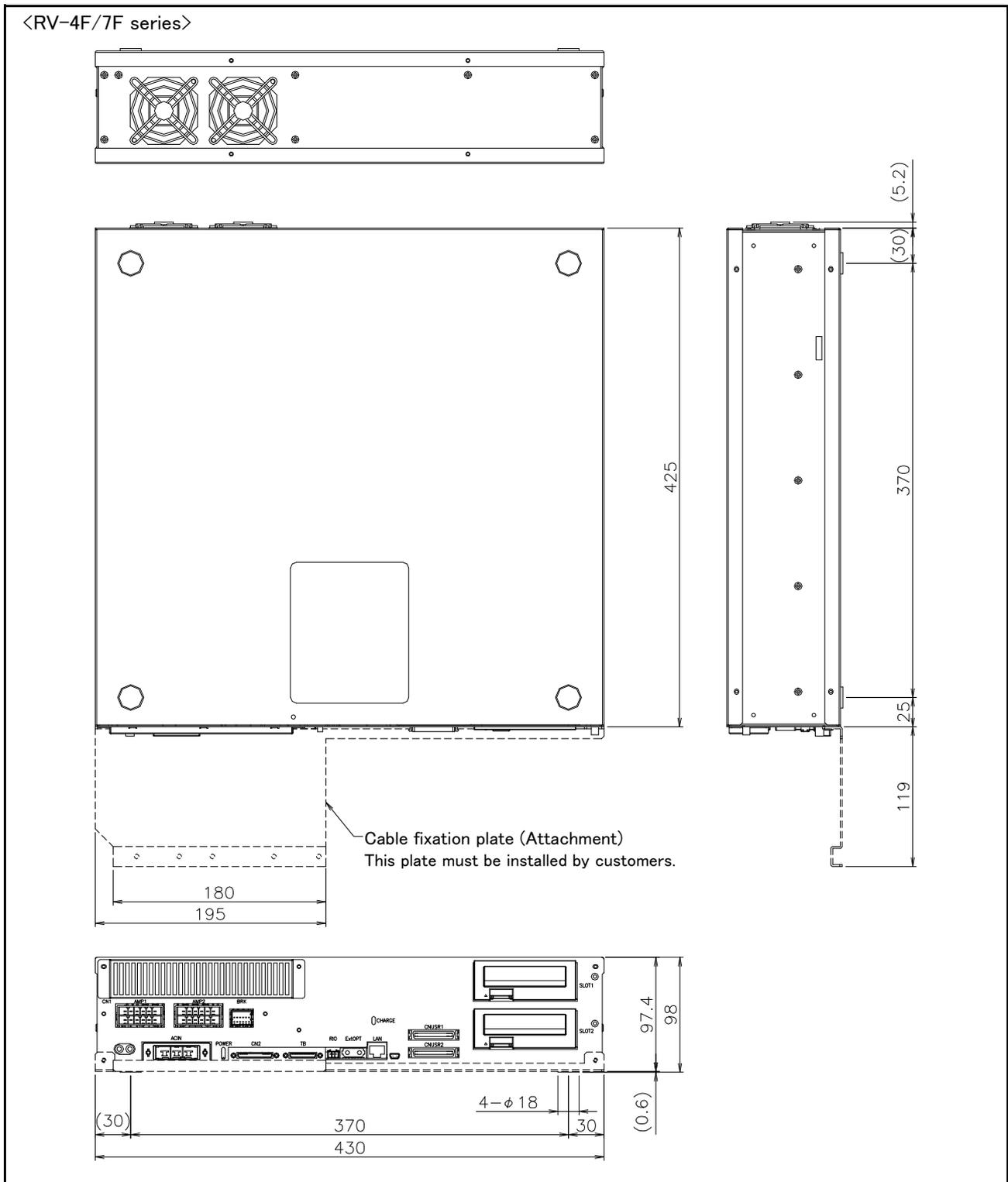
Fig.3-7 : Outside dimensions of controller (CR751: RV-4F/7F series)
