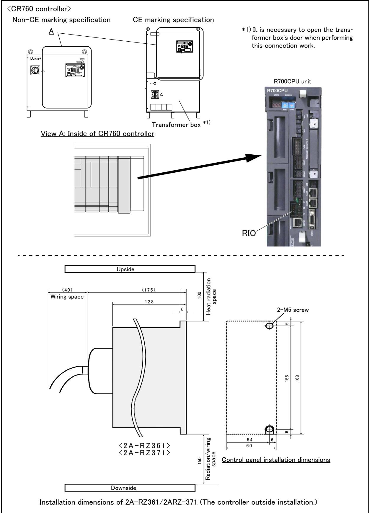
Fig.3-58 : Installing the parallel I/O unit (CR760)
