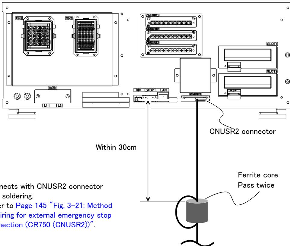
\* Connects with CNUSR2 connector with soldering.
