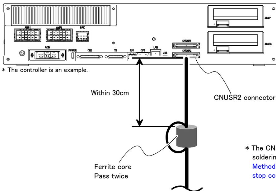
Fig.3-44 : AXMC terminal connector (CR751)
