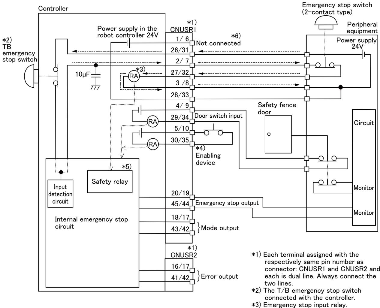
Fig.6-8 : Example of safety measures (CR751 wiring example 3)
