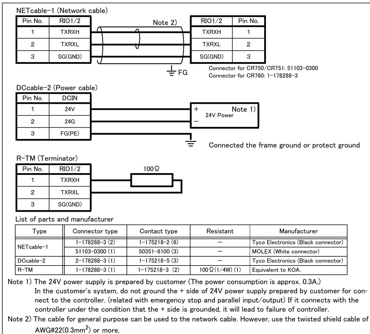
Fig.3-55 : Specifications for the connection cable
