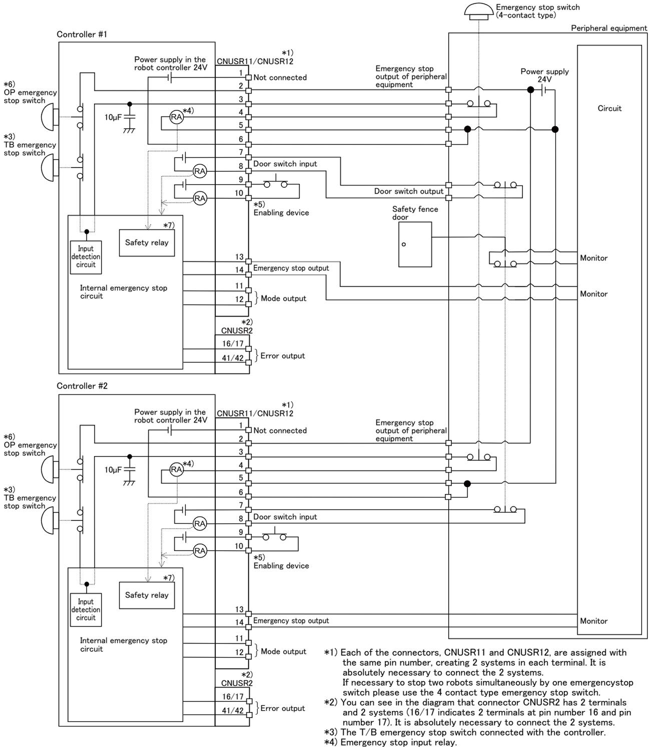
Fig.6-4 : Example of safety measures (CR750 wiring example 4)
