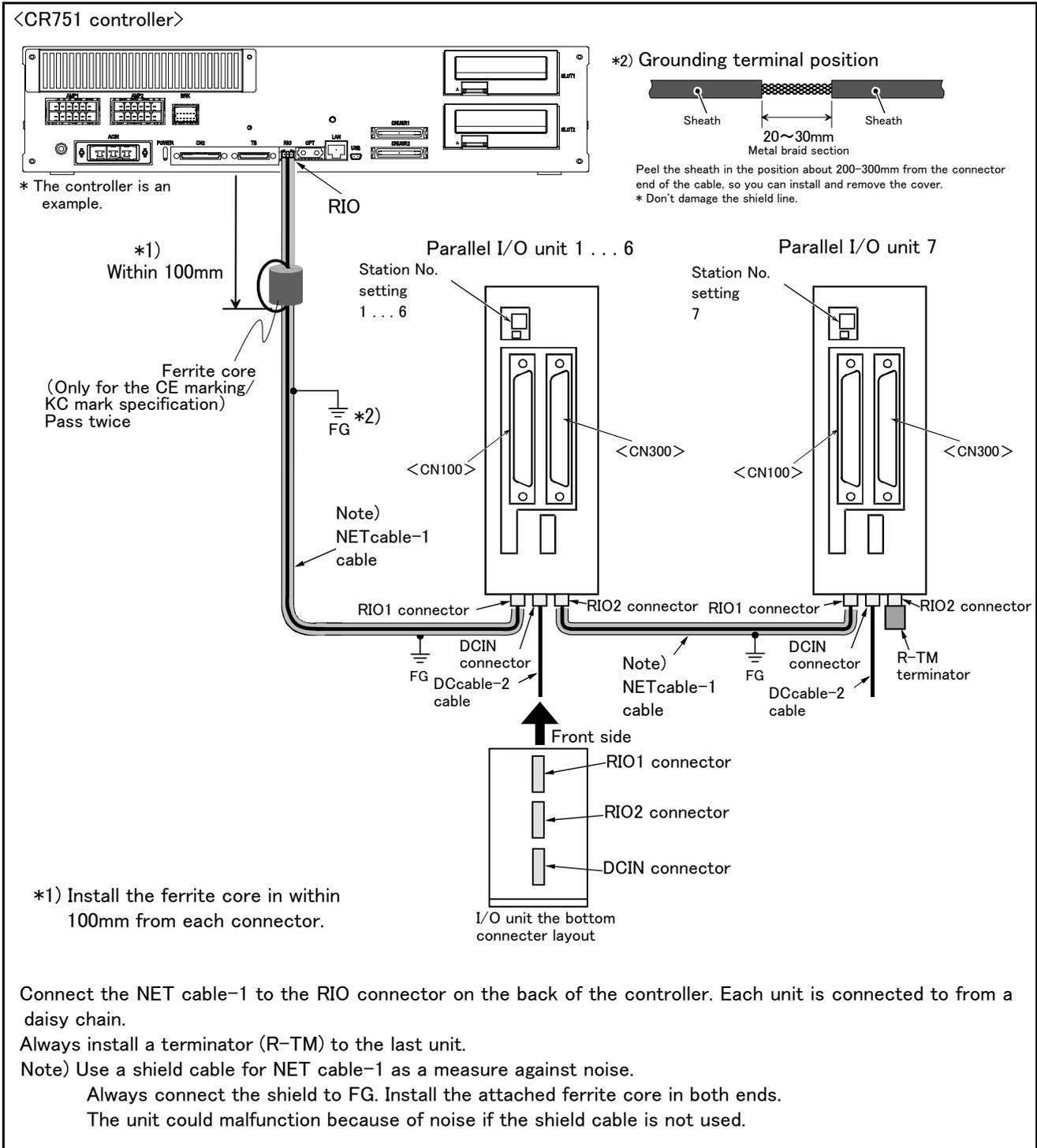
Fig.3-60 : Connection method of expansion parallel I/O unit (CR751)
