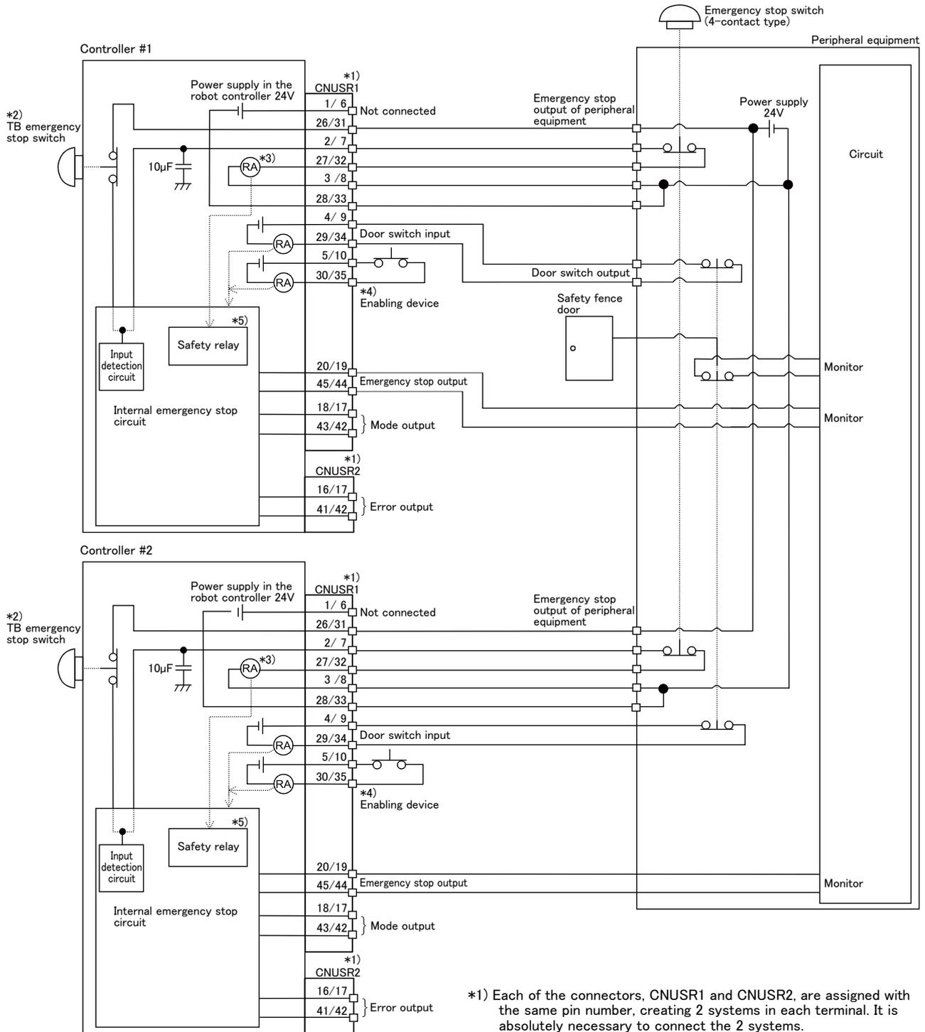
\*1) Each of the connectors, CNUSR1 and CNUSR2, are assigned with the same pin number, creating 2 systems in each terminal. It is absolutely necessary to connect the 2 systems.
