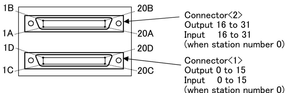
Fig.3-51 : Pin layout of connector
