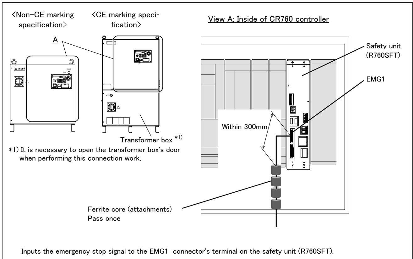
Fig.3-25 : Emergency stop cable connection (CR760)
