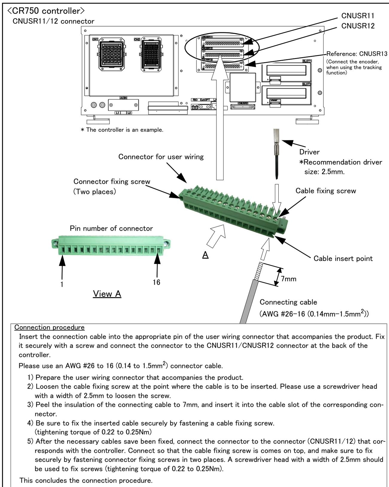
Fig.3-20 : Method of wiring for external emergency stop connection (CR750 (CNUSR11/12))
