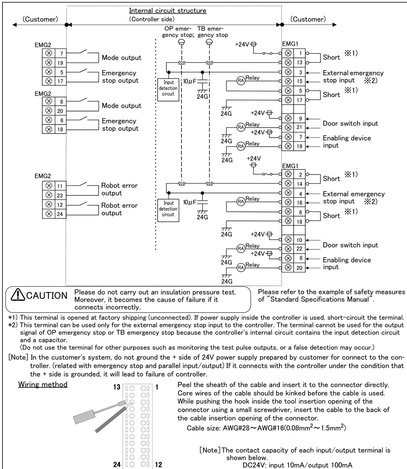
Fig.3-26 : External emergency stop connection (CR760)
