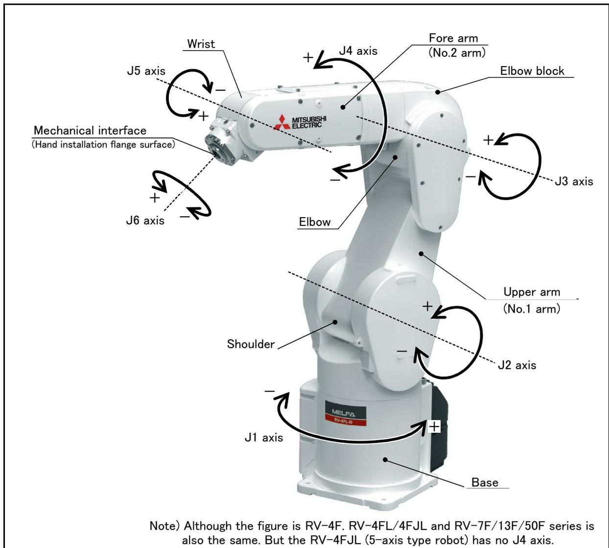
Fig.2-8 : Names of each part of the robot
