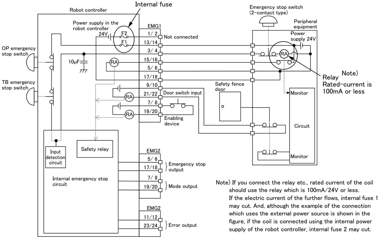
Fig.6-18 : Limitations when connecting the relay etc. (CR760)
