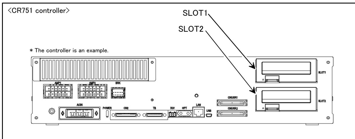
Fig.3-49 : Parallel I/O interface installation position (CR751)
