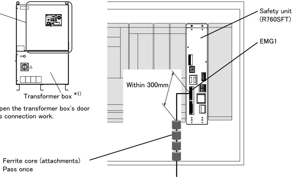
\* Connection method is the same as the connection of emergency stop.
