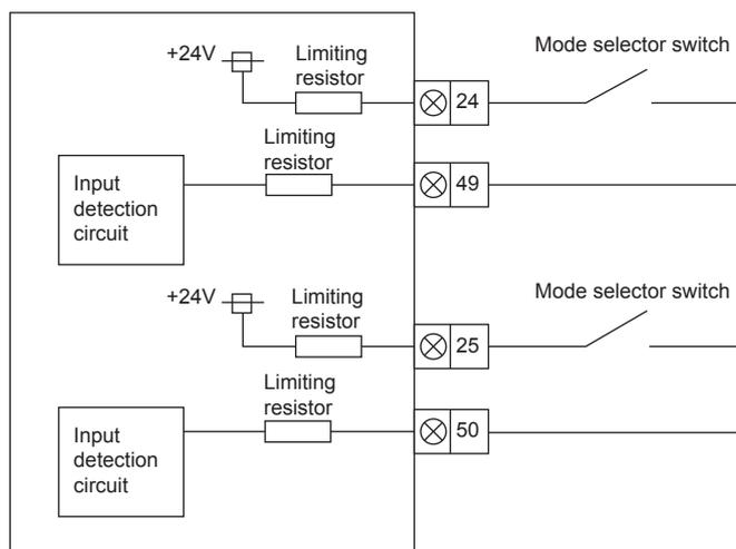
Fig.3-33 : Mode selector switch connection diagram
