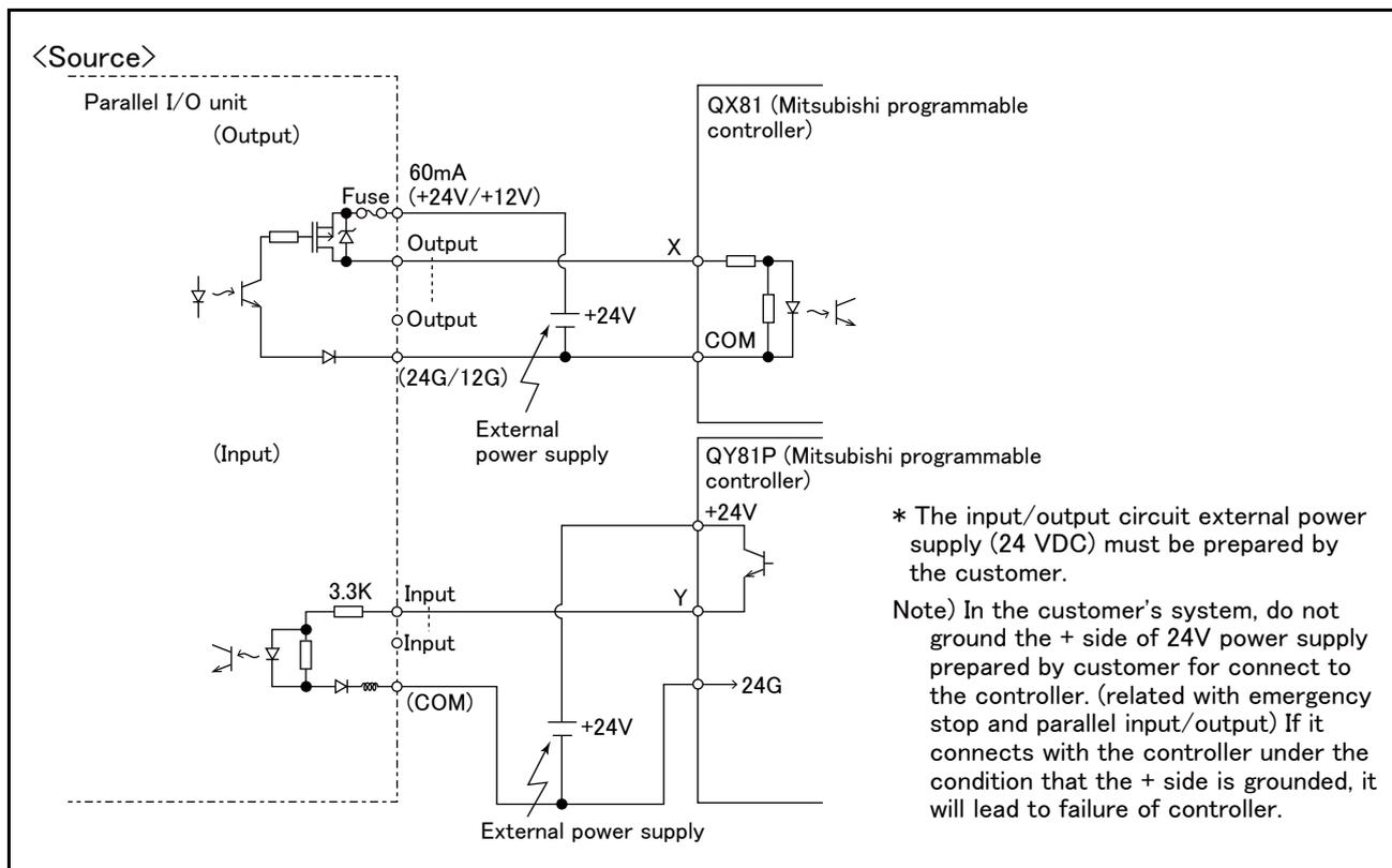
Fig.3-64 : Connection with a Mitsubishi PLC (Example of source type)
