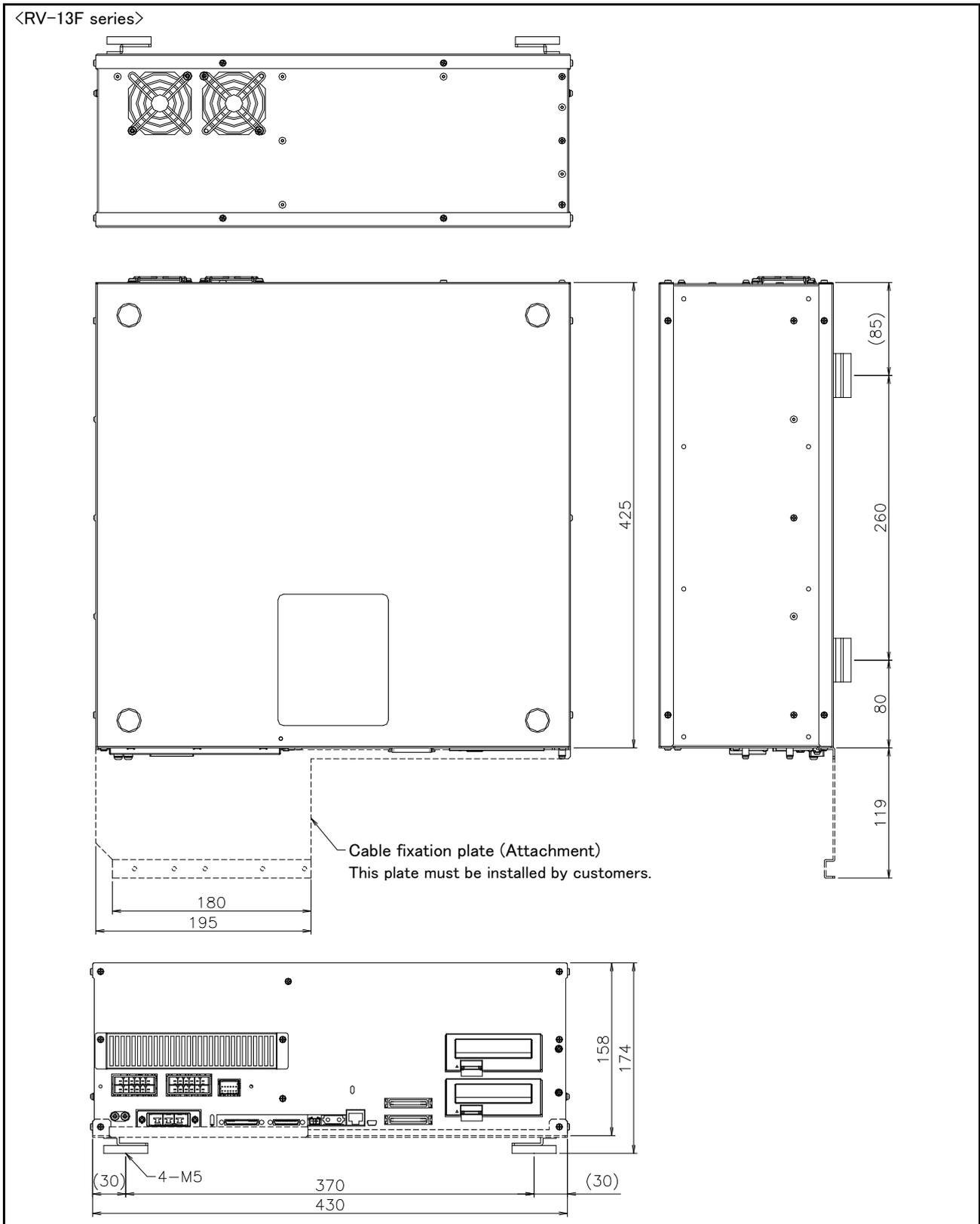
Fig.3-8 : Outside dimensions of controller (CR751: RV-13F series)
