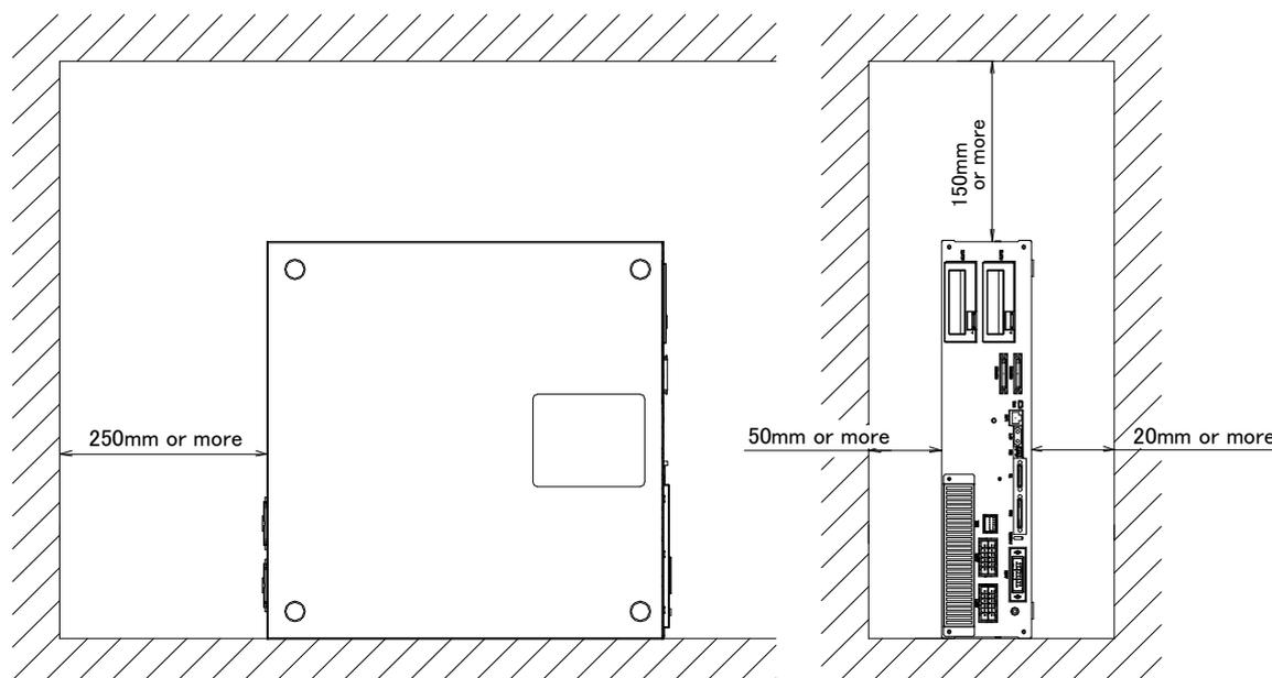
Fig.3-13 : Installation of controller (CR751: RV-4F/7F series)
