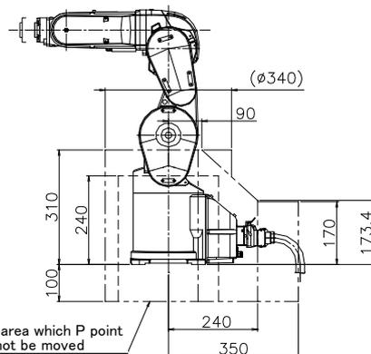
Fig.2-10 : Operating range diagram: RV-4F
