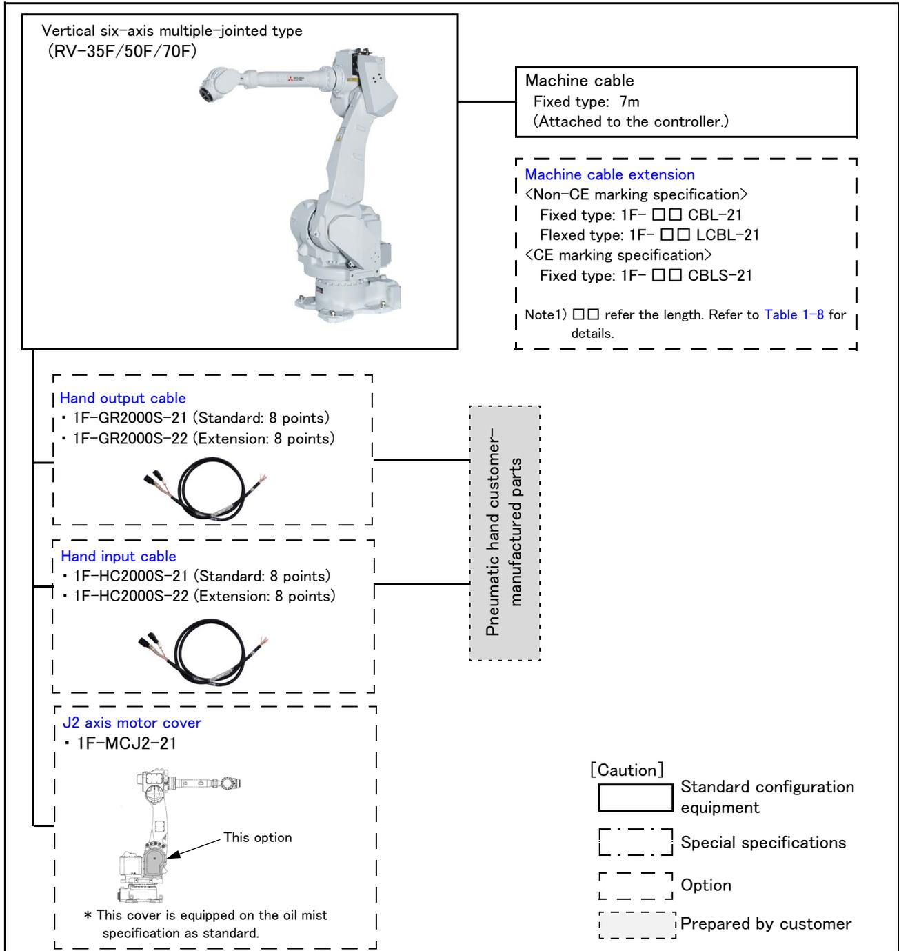
Fig.1-2 : Structural equipment (Robot arm)
