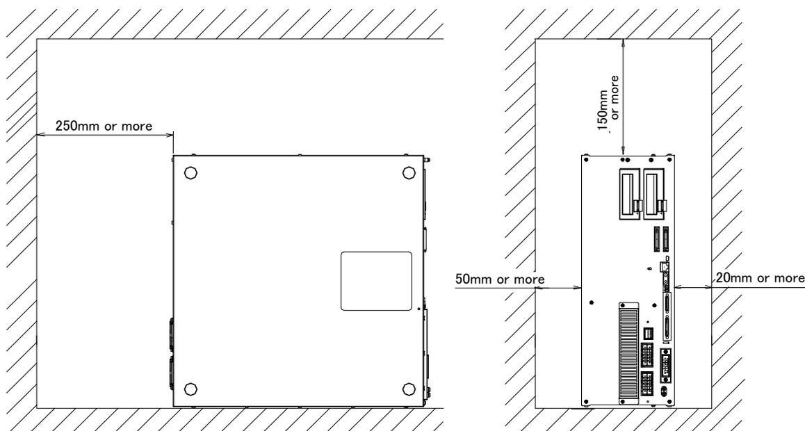
Fig.3-15 : Installation of controller (CR751: RV-13F series)
