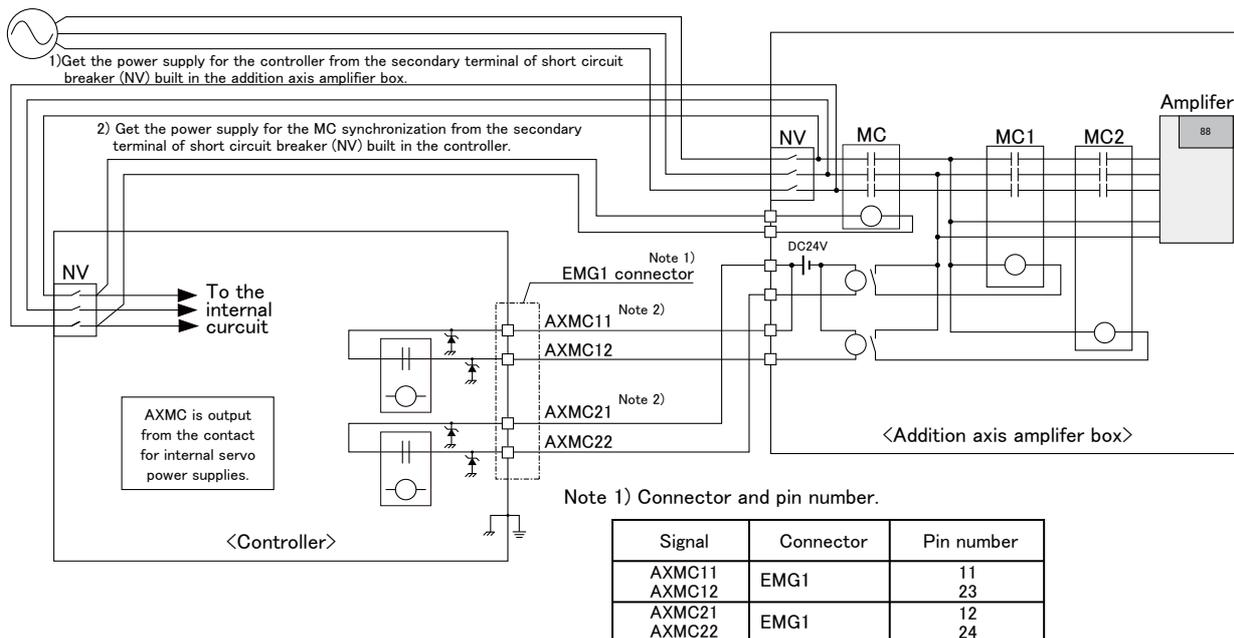
Note 2) This output is opened, if the robot turns off the servo by occurrence of alarm etc.
