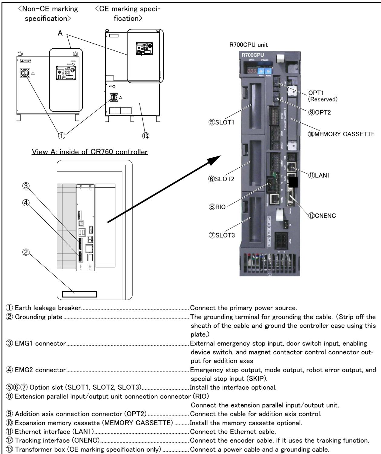
Fig.3-5 : Names of controller parts (inside of CR760)
