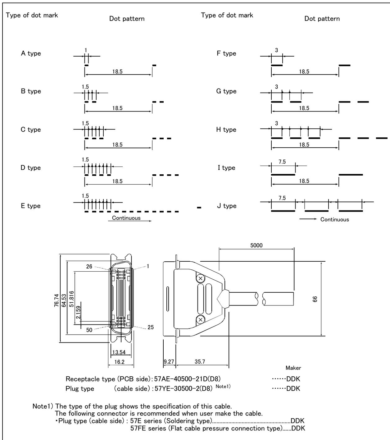
Fig.3-65 : Connections and outside dimensions
