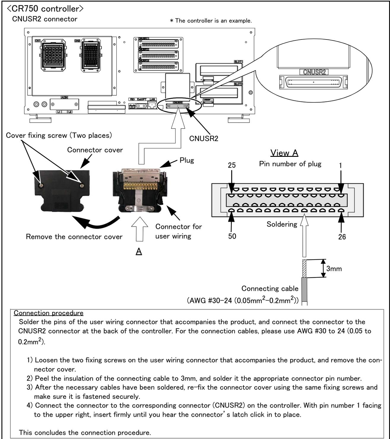
Fig.3-21 : Method of wiring for external emergency stop connection (CR750 (CNUSR2))
