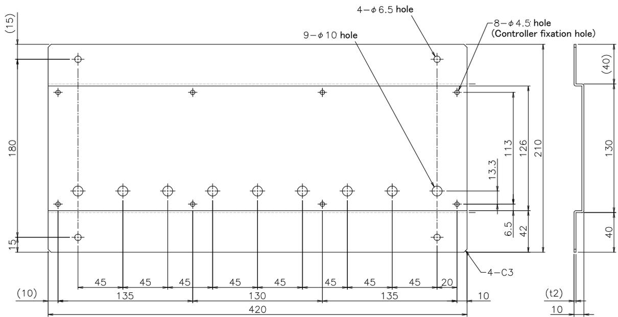
Fig.3-16 : Metal plate for fixation to placing vertically (Reference for CR751: RV-13F series)
