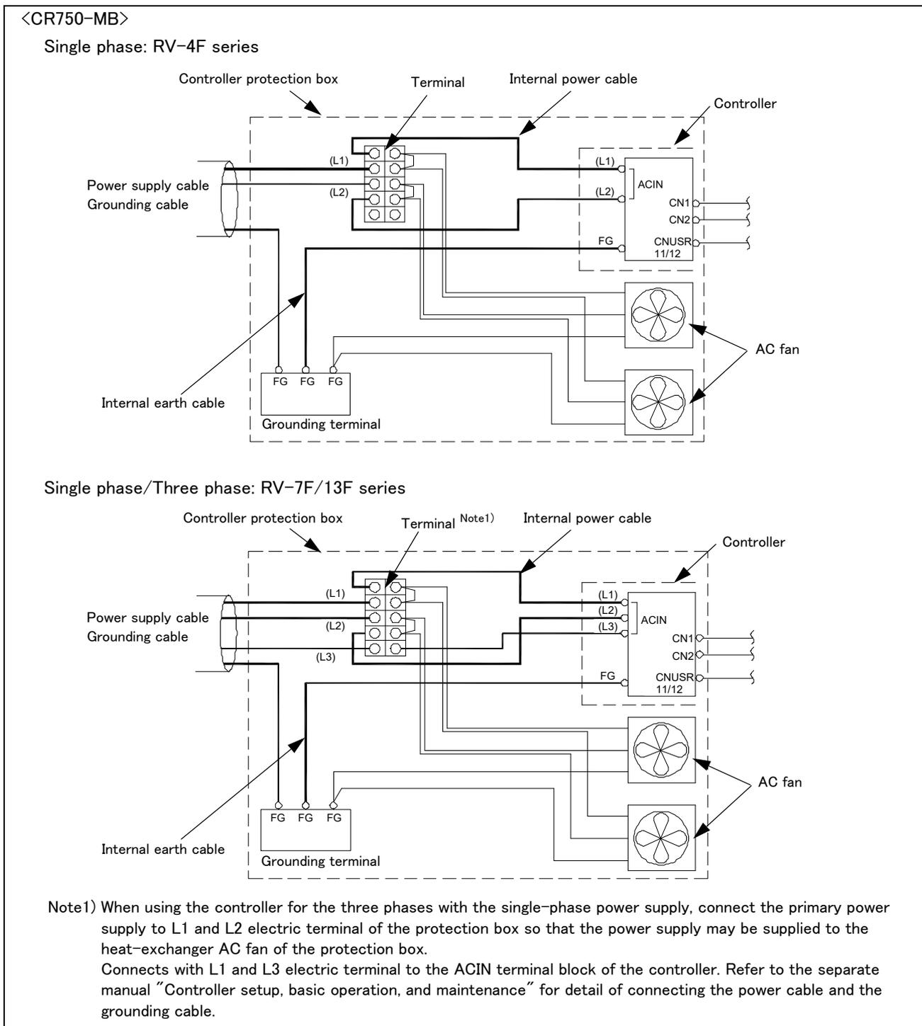
Fig.3-72 : Wiring system diagram (CR750-MB)
