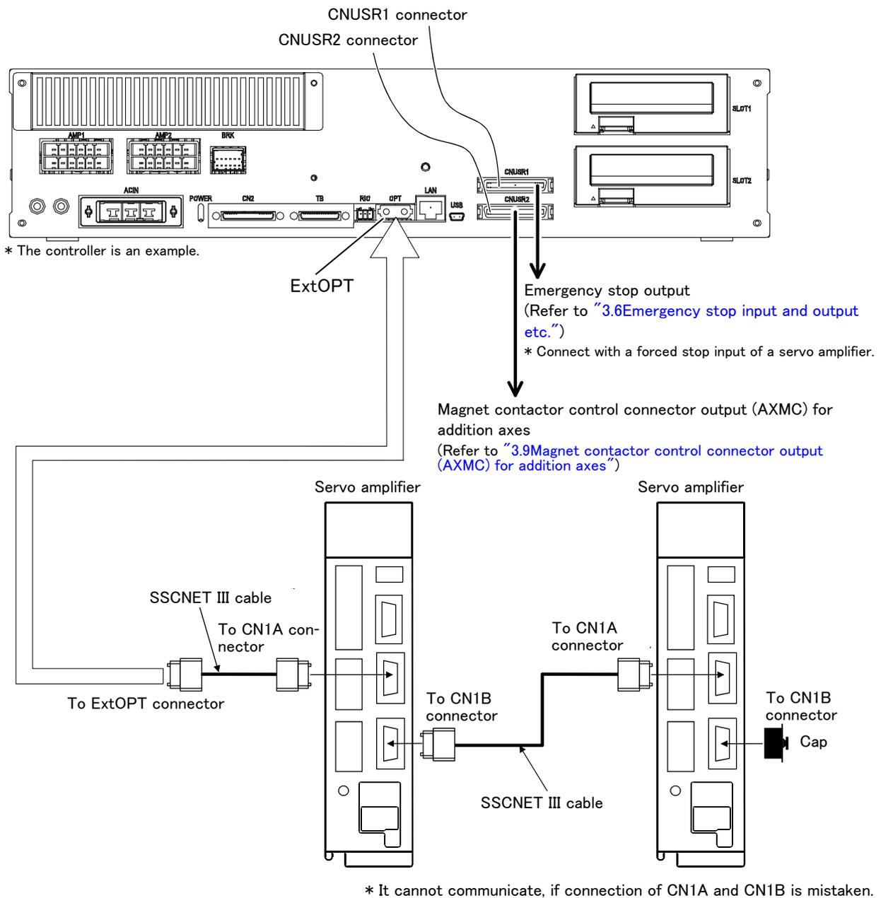
Fig.3-36 : Example of addition axis connection (CR751)
