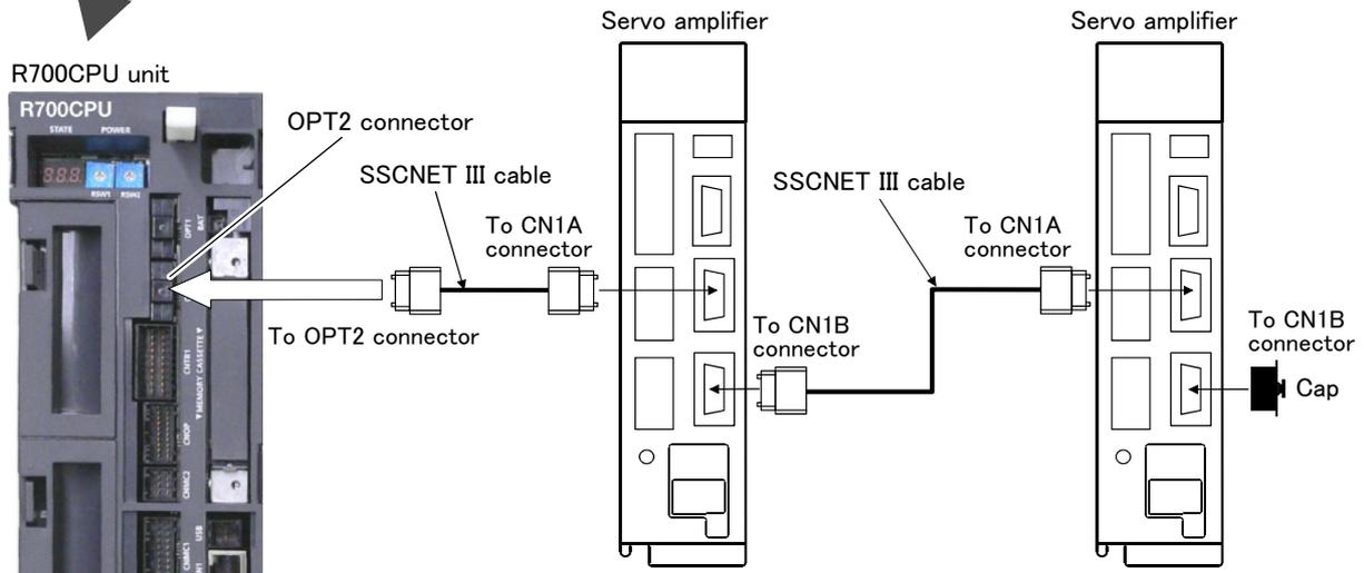
\* It cannot communicate, if connection of CN1A and CN1B is mistaken.
