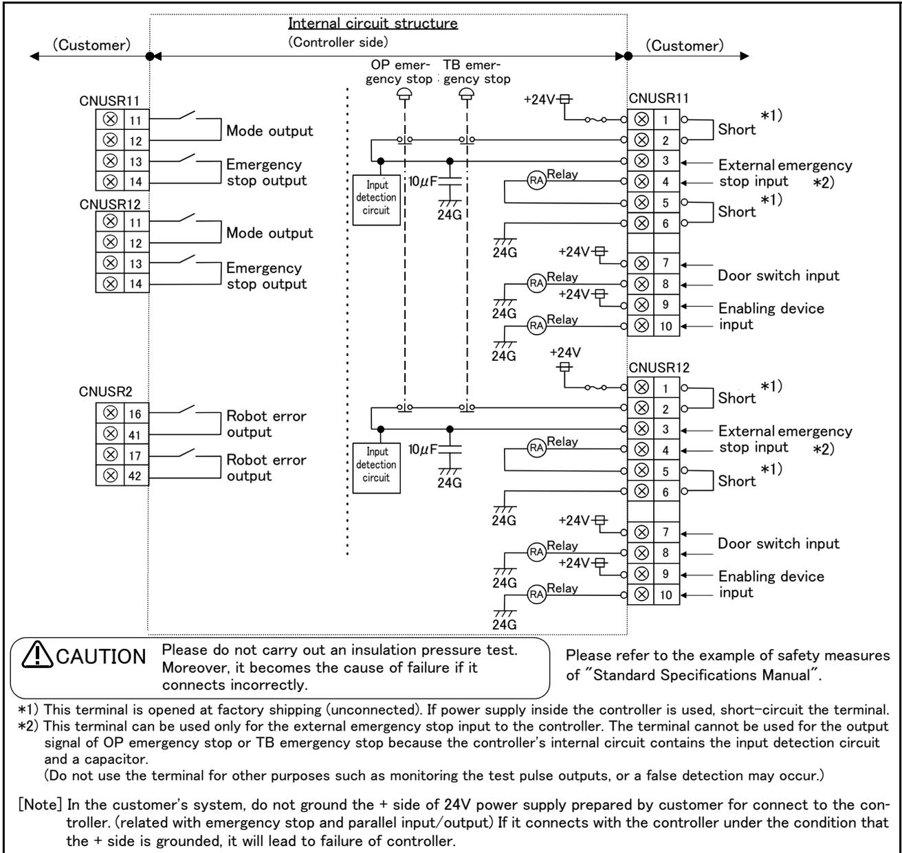
Fig.3-19 : External emergency stop connection (CR750)
