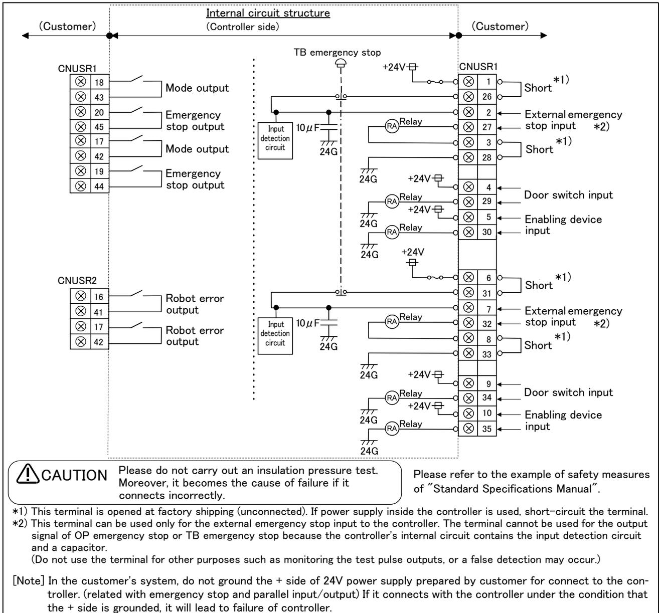
Fig.3-23 : External emergency stop connection (CR751)
