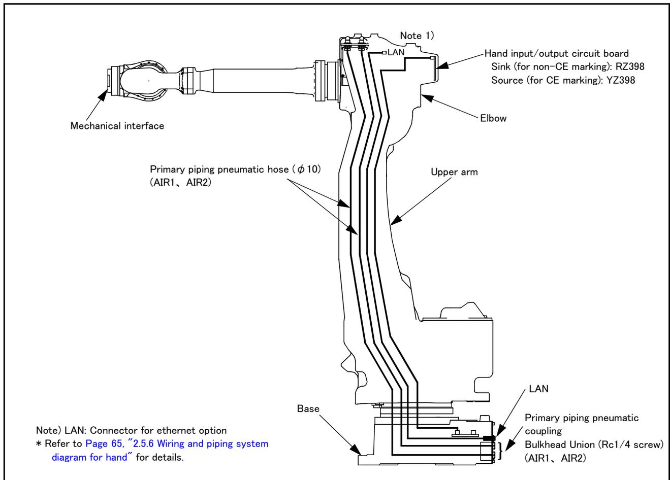
Fig.2-32 : RV-35F/50F/70F series wiring and piping for hand
