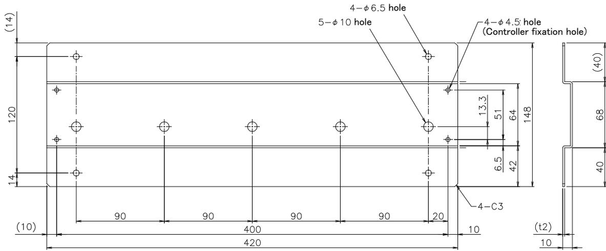
Fig.3-14 : Metal plate for fixation to placing vertically (Reference for CR751: RV-4F/7F series)
