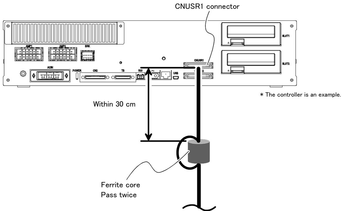
Fig.3-22 : Emergency stop cable connection (CR751)
