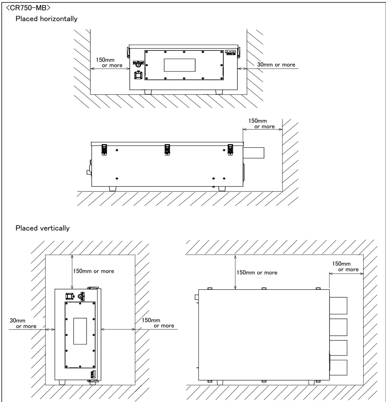
Fig.3-74 : Installation dimensions (CR750-MB)
