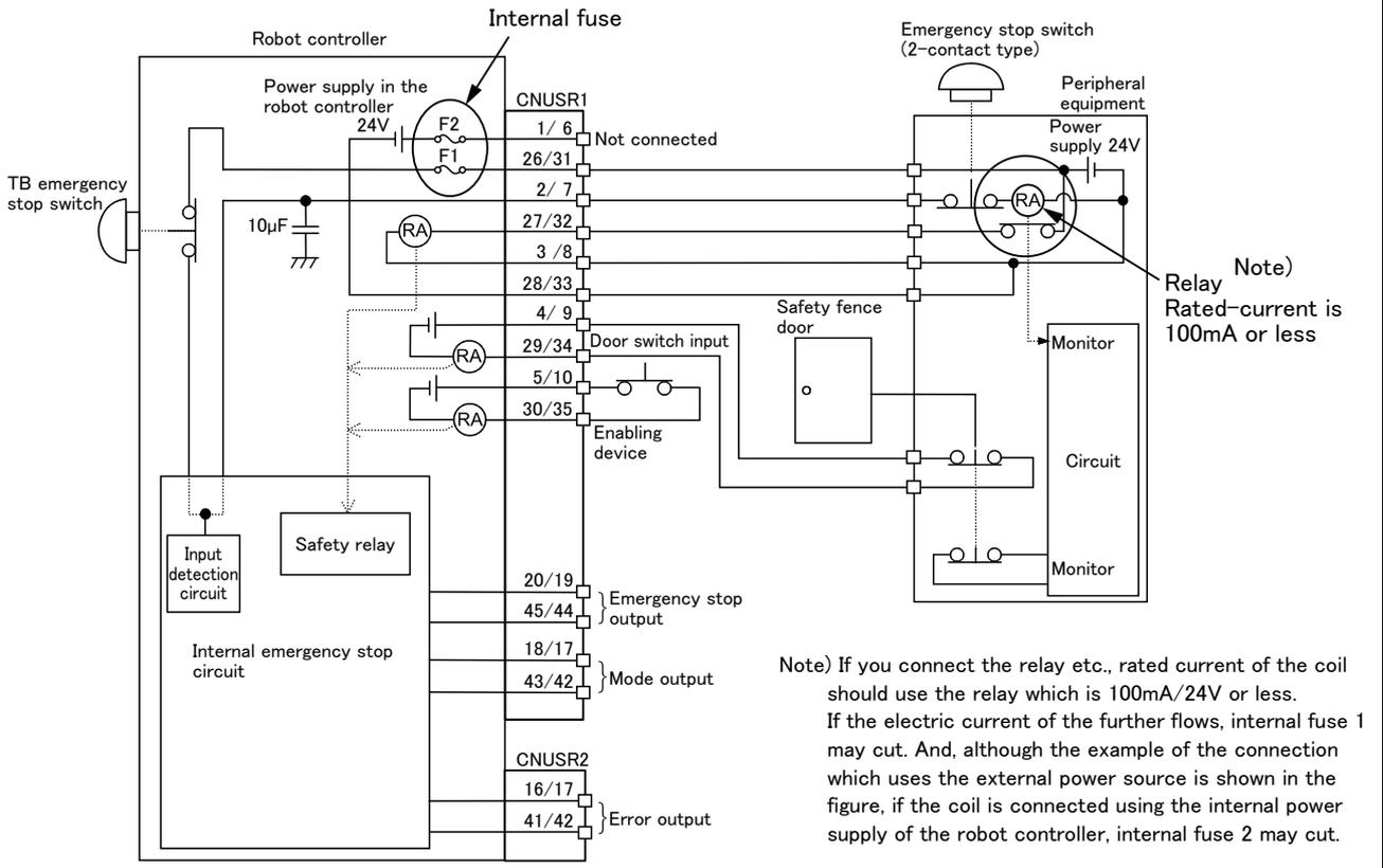
Fig.6-17 : Limitations when connecting the relay etc. (CR751)
