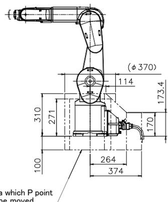
Fig.2-16 : Operating range diagram: RV-7FL
