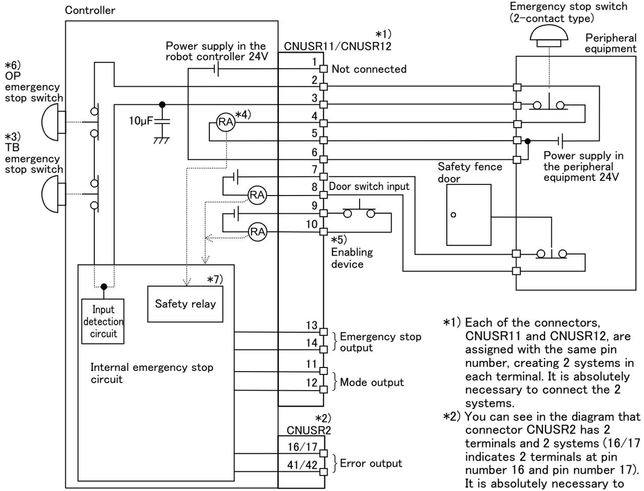
\*1) Each of the connectors, CNUSR11 and CNUSR12, are assigned with the same pin number, creating 2 systems in each terminal. It is absolutely necessary to connect the 2 systems.
