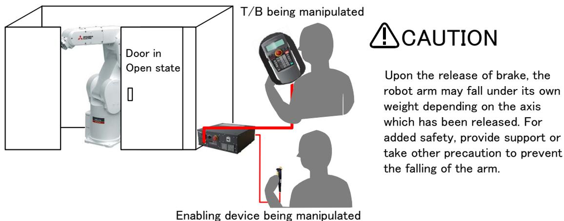
Fig.3-31 : Brake release operation
