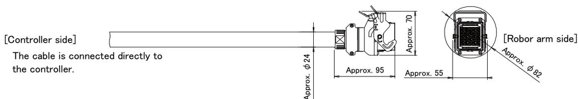
Note) If using an optional machine cable extension, refer to Page 85, "(1) Machine cable extension" in a diameter of the cable.
