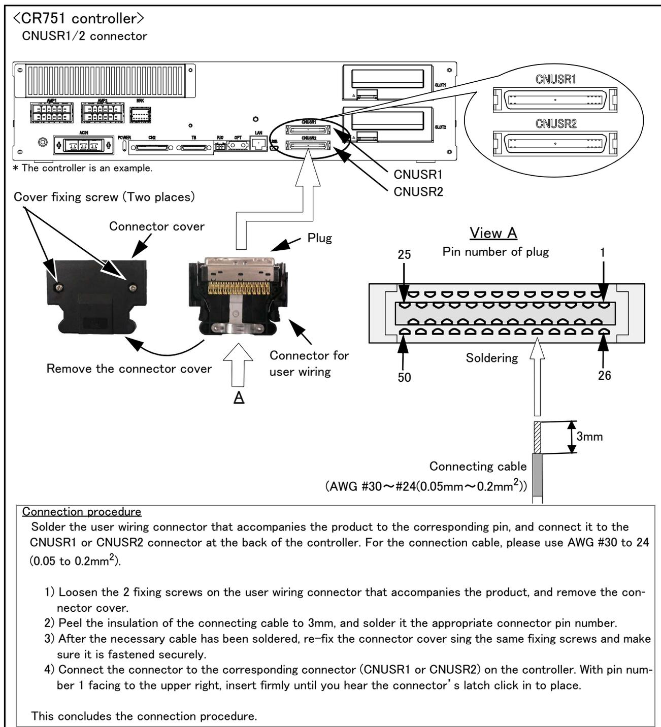
Fig.3-24 : Method of wiring for external emergency stop connection (CR751 (CNUSR1/2))
