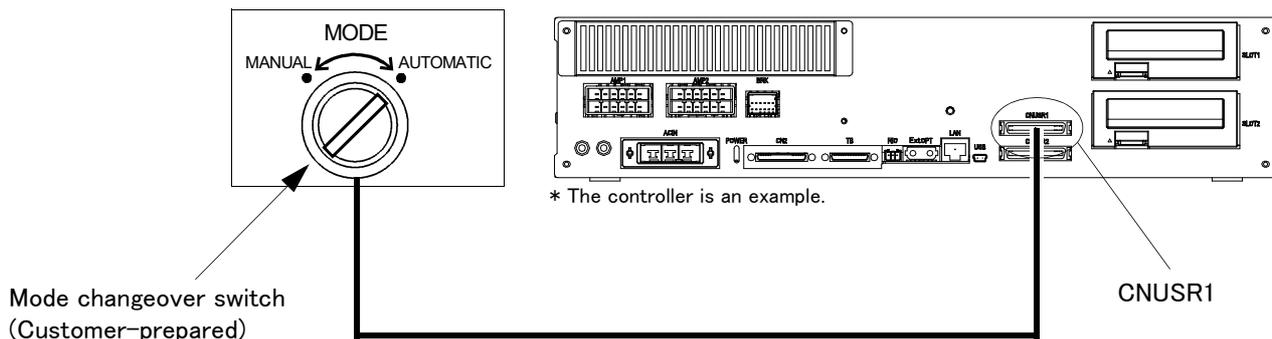
Fig.3-32 : Mode changeover switch image figure (CR751)
