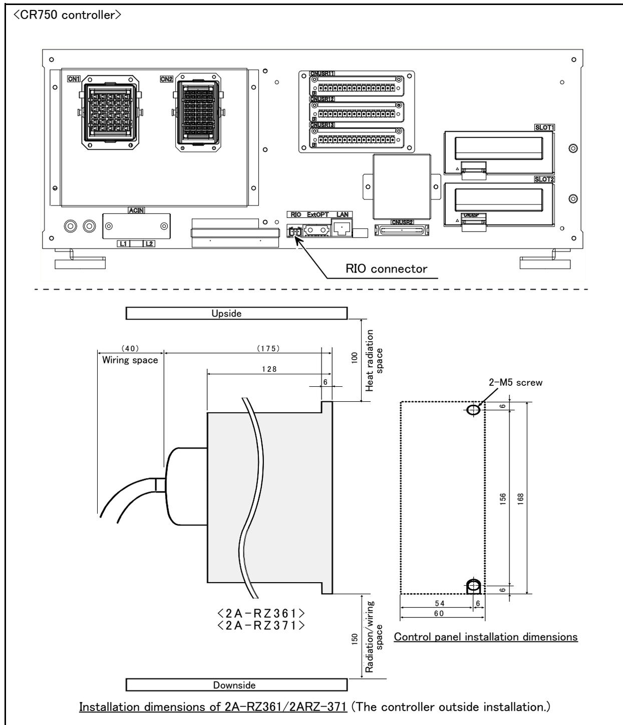
Fig.3-56 : Installing the parallel I/O unit (CR750)
