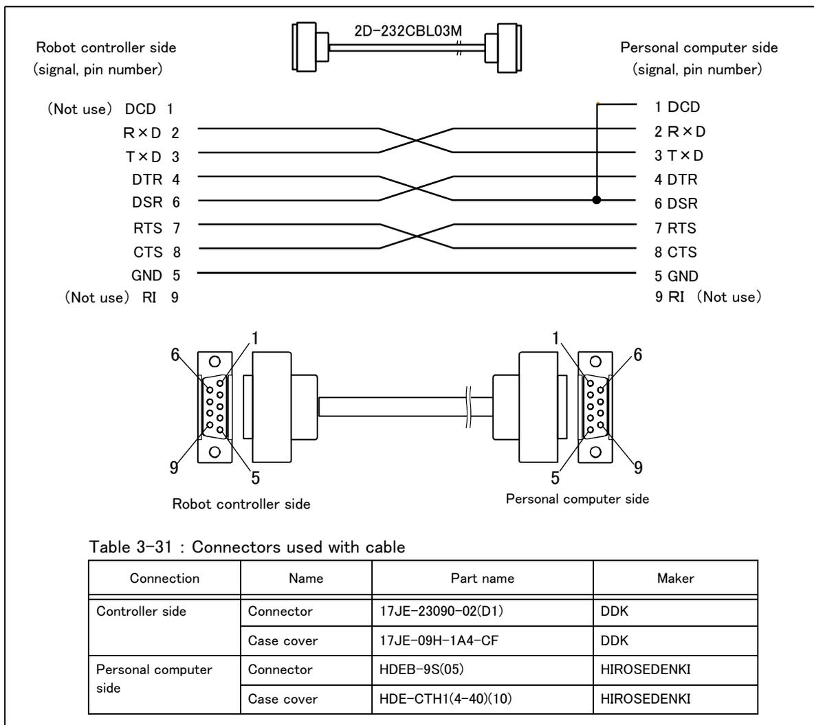
Fig.3-66 : Personal computer cable connection
