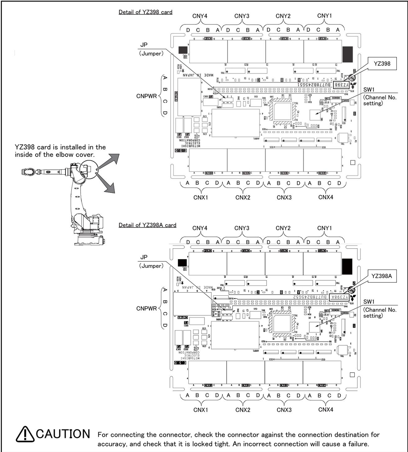
Fig.2-41 : Detail of hand I/O card (YZ398)
