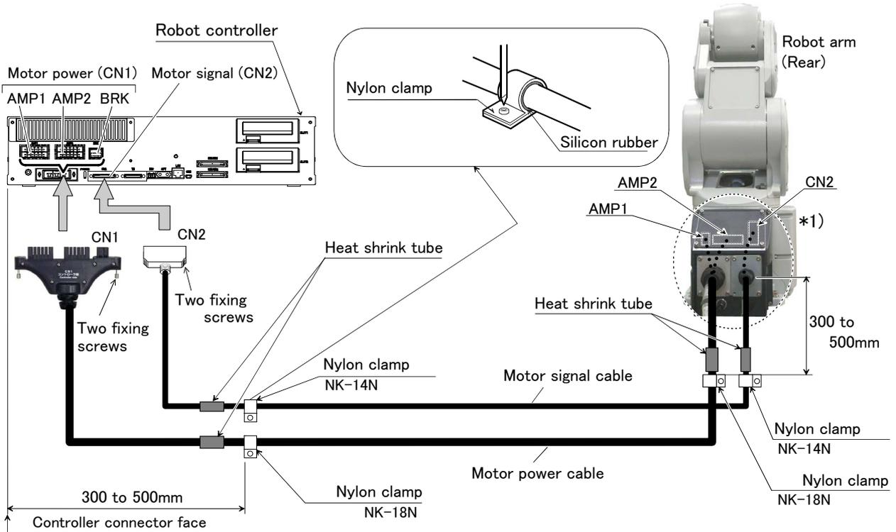
\*1) Connect the robot arm side connector to the connector which is inside the CONBOX cover.
