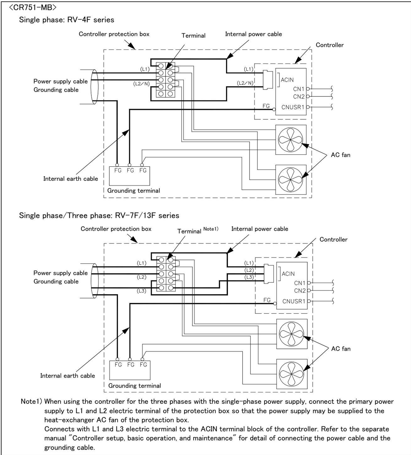
Fig.3-73 : Wiring system diagram (CR751-MB)
