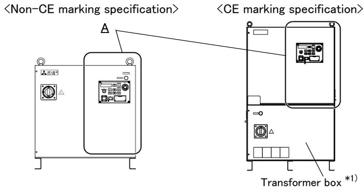
\*1) It is necessary to open the transformer box's door when performing this connection work.
