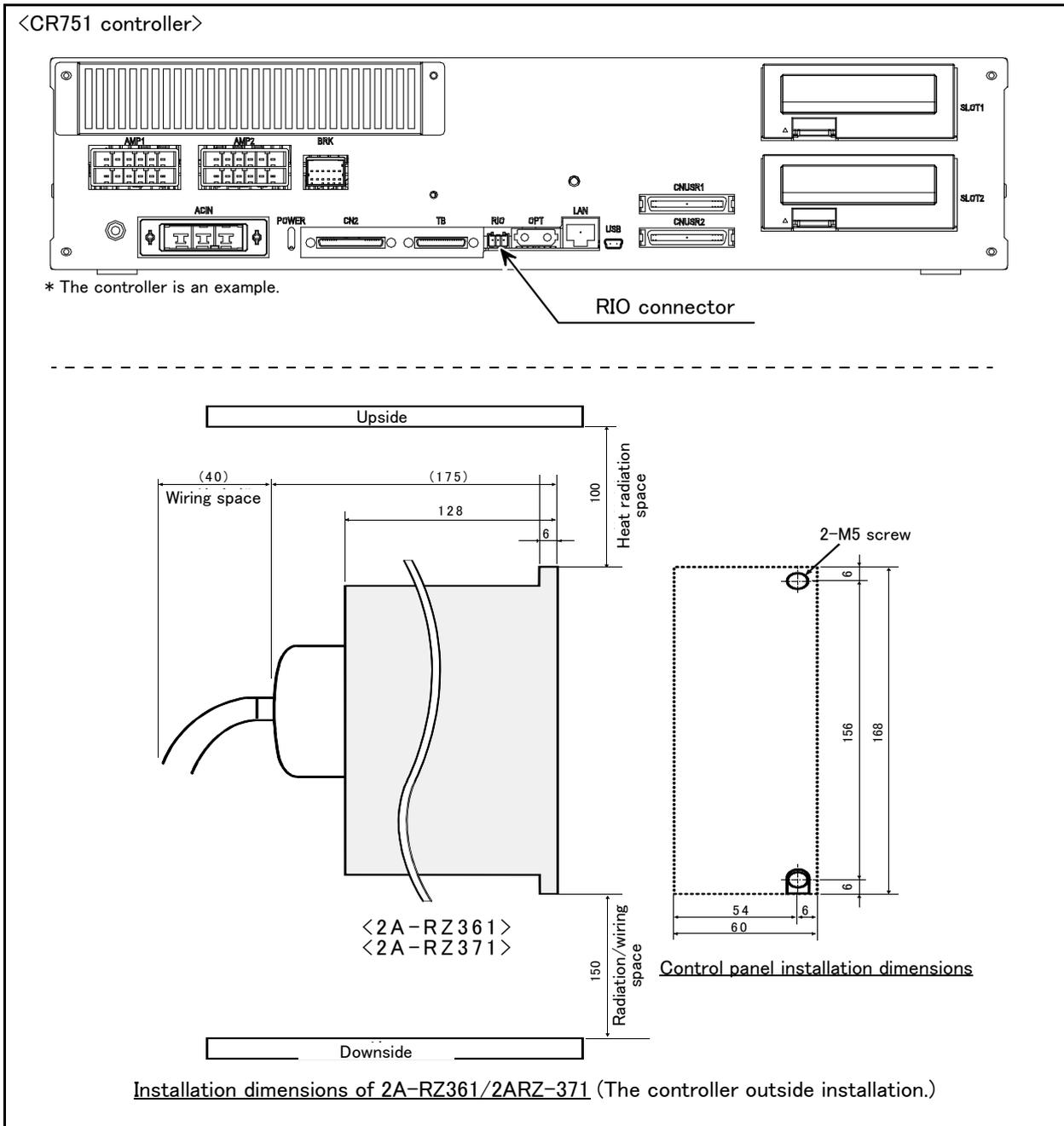
Fig.3-57 : Installing the parallel I/O unit (CR751)
