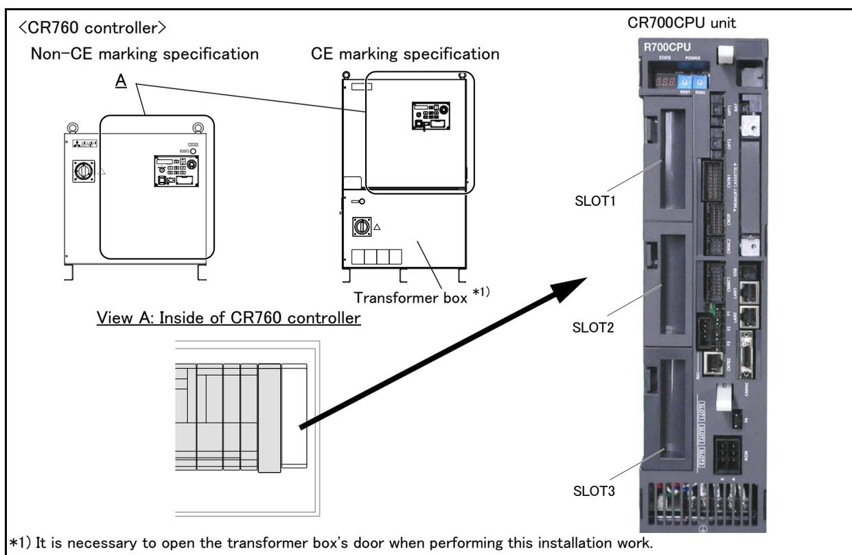
\*1) It is necessary to open the transformer box's door when performing this installation work.
