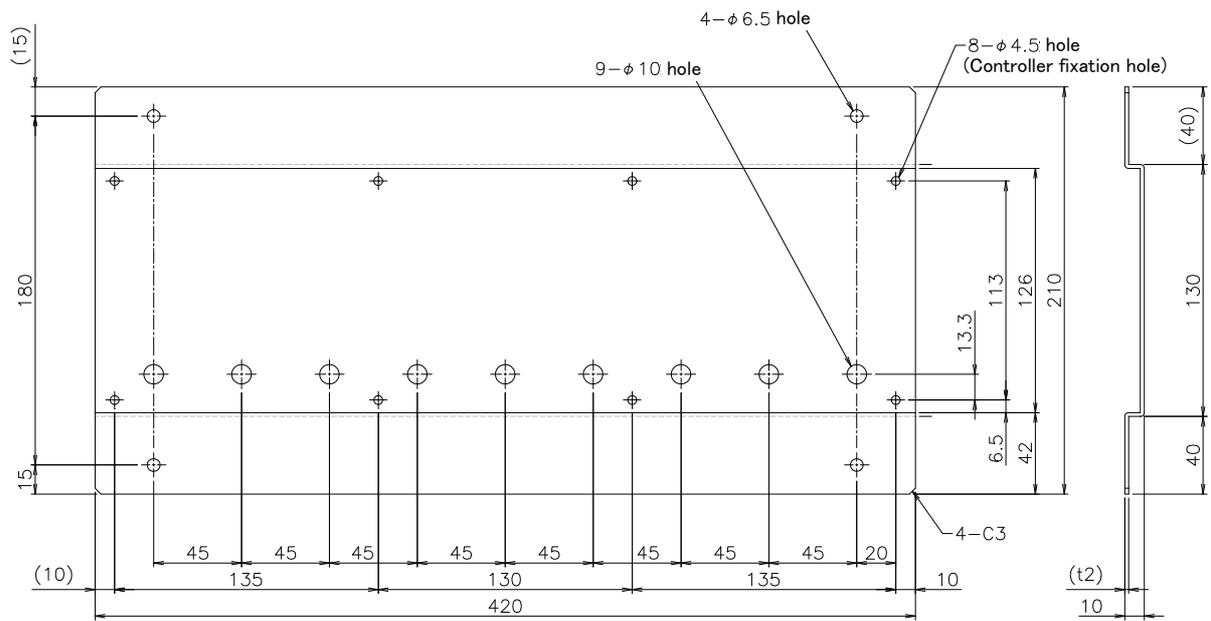
Fig.3-12 : Metal plate for fixation to placing vertically (Reference for CR750)
