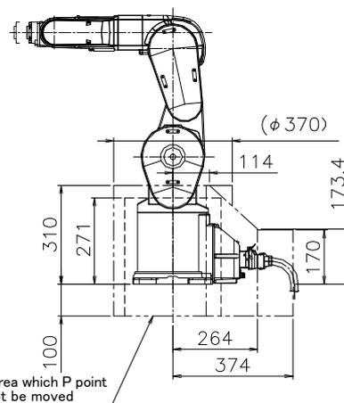
Fig.2-14 : Operating range diagram: RV-7F
