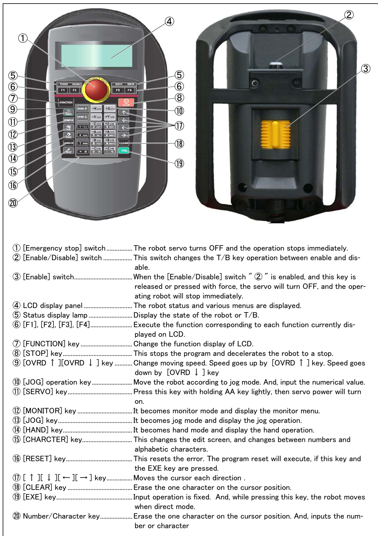
Fig.3-51 : Teaching pendant key layout and main functions
