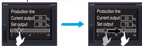
Changing the set output with the slider
