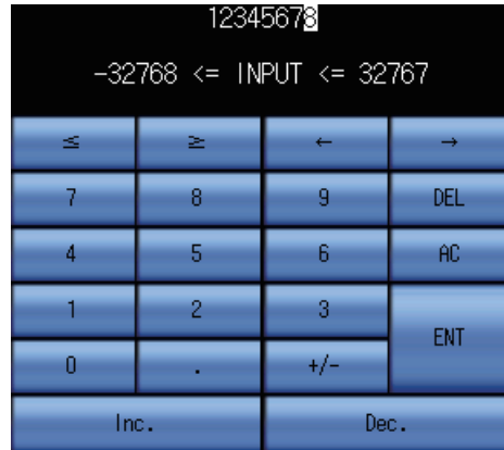
Example) User-created key window (for numerical input (decimal))
