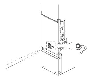
**2.** Open the terminal block cover and insert the side protection cover along the slit on the right side of the terminal block. If the control circuit power supply is wired from the right side, pass the wire through the groove on the side protection cover to prevent it from getting caught.
