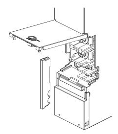
3. Close the terminal block cover and set the lock of the terminal block cover to "LOCK". (Turn it clockwise.)
