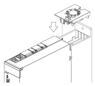
**2.** Tighten the fan unit with screws. Use the same screws as those used for the fan unit before replacement.
