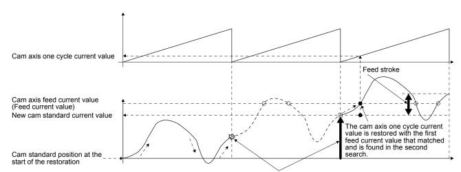
Once the first search fails, the cam standard position is automatically updated and the second search starts so that "Feed current value - New cam standard position" is within the feed stroke amount.
