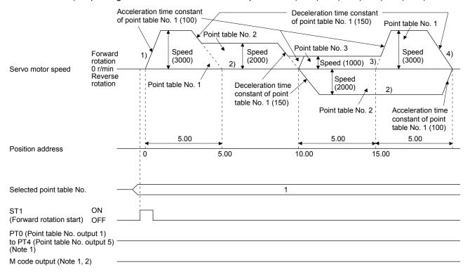
Note 1. PT0 to PT4 and M code are not outputted in automatic continuous operation.
