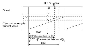
Increase the conveyor travel distance by adding the difference (CPHV - cpos) to the cam axis one cycle current value. Adjust the filter time constant for acceleration/deceleration at compensation with [Cam control data No. 61 Cam position compensation time constant].
