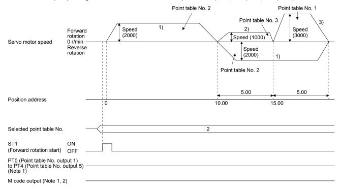
Note 1. PT0 to PT4 and M code are not outputted in automatic continuous operation.
