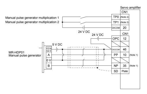
Note 1. To assign PP and NP, set [Pr. PD44] and [Pr. PD46] to "0 0 \_ \_ ".
