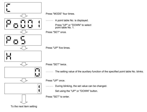
Press the "UP" or "DOWN" button to switch to other item of the same point table No. Press the "MODE" button to switch to the next point table No.
