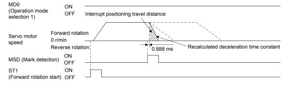
(b) If the interrupt travel distance is large during acceleration, the servo motor stops with the deceleration time constant after rotating with the command speed at which MSD (Mark detection) turned on.
