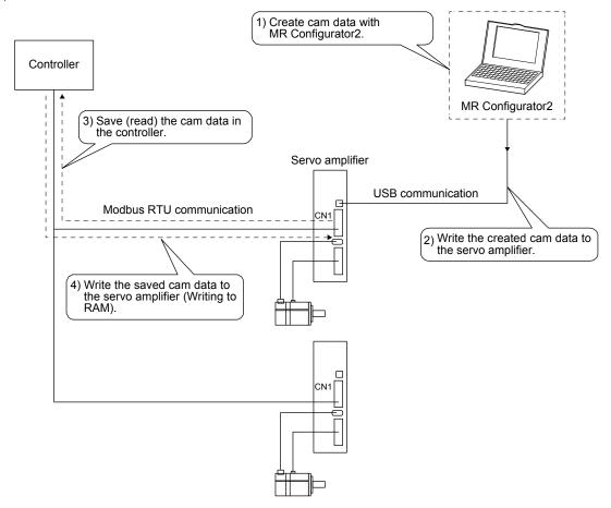
The cam No., cam axis one cycle length, and cam stroke amount of the cam control data can be written to the servo amplifier from the controller. Set them using Cam number setting (2D80h), Cam axis one cycle length setting (2D84h), and Cam stroke length setting (2D85h). Refer to section 6.1.7 (1) for the cam control data.
