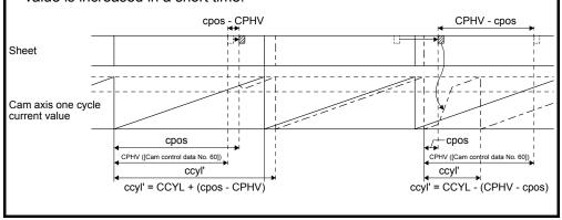
The cam position compensation processing compensates the difference between the target position for detecting the sensor and the actual position for detecting the sensor by shifting the cam axis one cycle current value. ccyl', the cam axis one cycle length (sheet length) after compensation, is calculated as follows:
