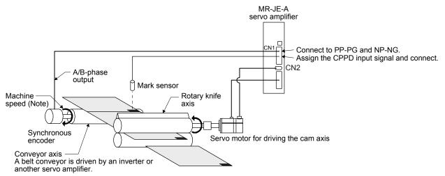
Note. Set the machine speed of the input axis to a value that satisfies the following equation.
