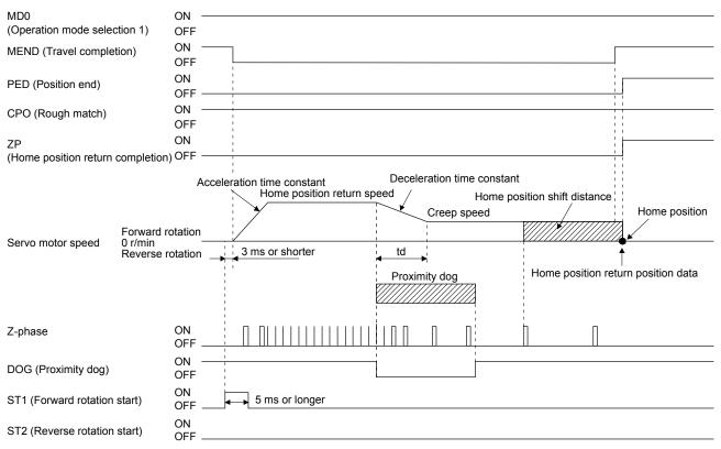
The setting value of [Pr. PT08 Home position return position data] is used as the position address at the home position return completion.
