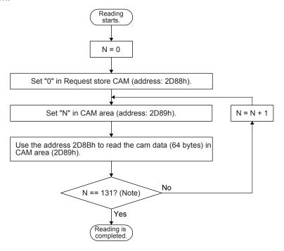
Note. The size of cam data is fixed to 8388 bytes. Thus, N, the setting range of the cam storage area is 0 to 131. Only a part of cam data cannot be read. Read the cam data stored in all areas.
