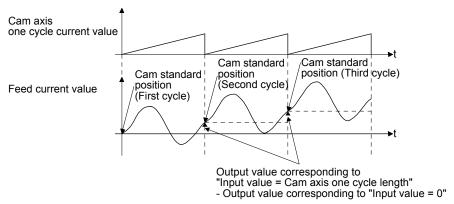
For to-and-fro control, use the output value corresponding to "Input value = Cam axis one cycle length" that is equal to output value corresponding to "Input value = 0".
