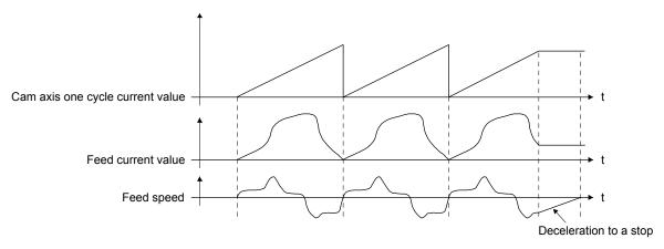
When using a positioning command (internal command) for the input axis, inputting a temporary stop or switching the operation mode decelerates the input axis to stop. Since the output axis stops in synchronization with the input axis, the synchronous relationship is kept and the cam control does not stop.
