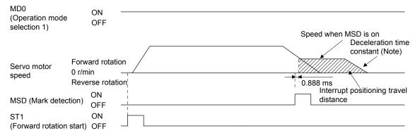
Note. Deceleration time constant of the point table at the time of start is applied for the point table method, and deceleration time constant set by the program in execution is applied for the program method.
