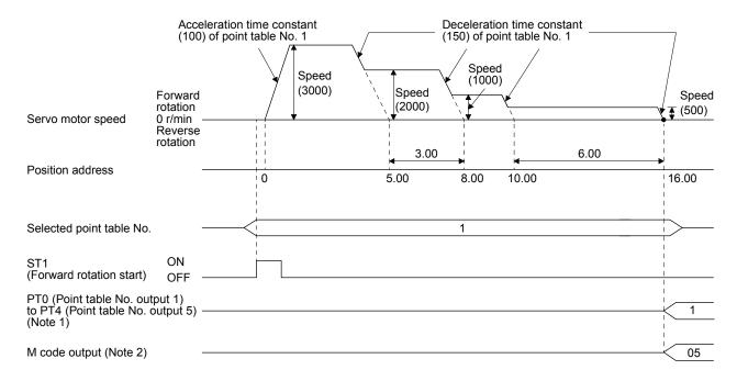
Note 1. For MR-JE-\_A servo amplifiers, up to four points of DO are available; therefore, PT0 to PT4 cannot be outputted simultaneously.
