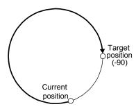
When the position data of -360.000 degrees is specified, the servo motor rotates in the CW direction. (A)
