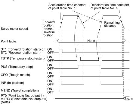
Note. For MR-JE-\_A servo amplifiers, up to four points of DO are available; therefore, PT0 to PT4 cannot be outputted simultaneously.
