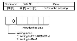
When changing the speed data frequently using communication, set "1" to the write mode to change only the RAM data in the servo amplifier.
