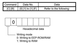
When changing the auxiliary function frequently using communication, set "1" to the write mode to change only the RAM data in the servo amplifier.
