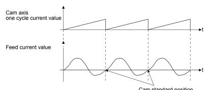
Cam standard position (Does not change because the stroke ratio is 0%.)
