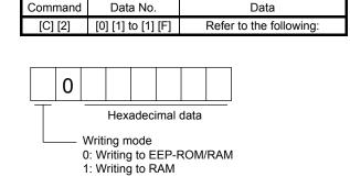
When changing the M code frequently using communication, set "1" to the write mode to change only the RAM data in the servo amplifier.
