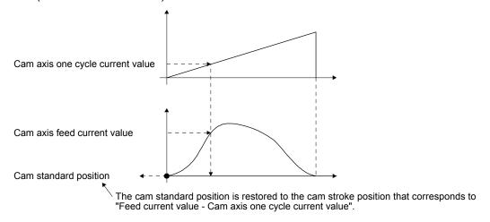
The following shows an example for restoring the cam standard position to start an operation from a point where both the feed current value and the cam axis one cycle current value are 0" in the cam whose cam data start position is not "0".
