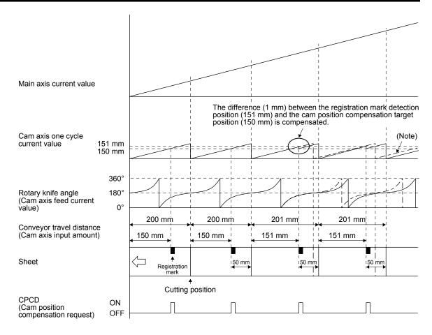
Note. The dot-and-dash line in the above figure shows a waveform of when compensation is not executed.
