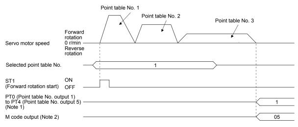
Note 1. For MR-JE-\_A servo amplifiers, up to four points of DO are available; therefore, PT0 to PT4 cannot be outputted simultaneously.
