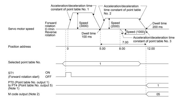
Note 1. For MR-JE-\_A servo amplifiers, up to four points of DO are available; therefore, PT0 to PT4 cannot be outputted simultaneously.
