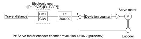
Set the electronic gear within the following range. Setting out of the range will trigger [AL. 37 Parameter error].
