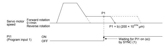
When the travel distance set by the "ITP" command is smaller than the travel distance required for deceleration, the actual deceleration time constant becomes smaller than the setting value of the "STB" command.
