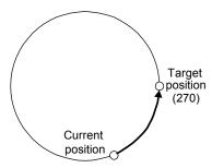
When the position data of -90.000 degrees is specified, the servo motor rotates in the CCW direction.
