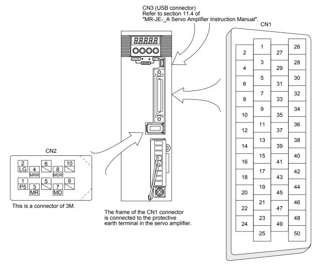
The device assignment of the CN1 connector pins changes depending on the control mode. For the pins which are given parameters in the related parameter column, their devices can be changed using those parameters.
