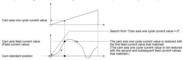
2) Searching from a value in the middle of the cam axis one cycle current value (Cam data start position = 0)
