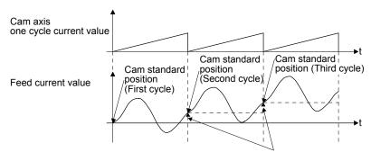
Cam stroke amount × Stroke ratio at the last point
