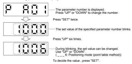
To shift to the next parameter, press the "UP" or "DOWN" button. After changing [Pr. PA01], cycle the power to enable the setting.
