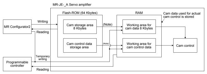
Note. When the power is turned on, the cam data and the cam control data are copied from the Flash-ROM to the RAM.
