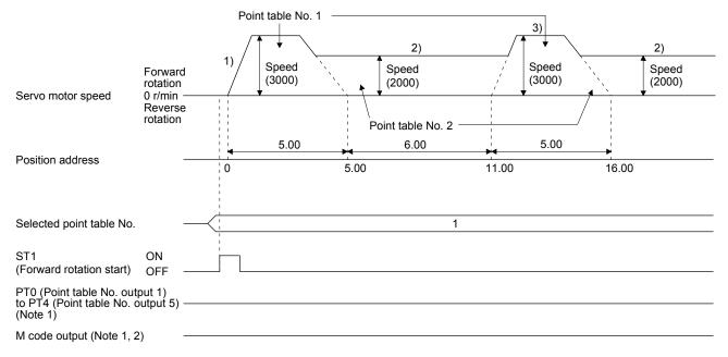
Note 1. PT0 to PT4 and M code are not outputted in automatic continuous operation.
