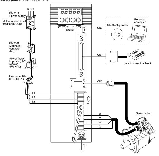
Note 1. For 1-phase 200 V AC to 240 V AC, connect the power supply to L1 and L3. Leave L2 open. For power supply specifications, refer to section 1.3 of "MR-JE-\_A Servo Amplifier Instruction Manual".
