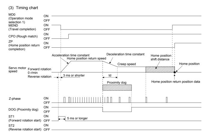
The setting value of [Pr. PT08 Home position return position data] is used as the position address at the home position return completion.
