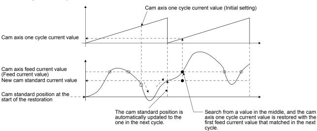
3) Searching from a value in the middle of the cam axis one cycle current value (Cam data start position ≠ 0)
