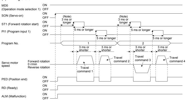
Note. The detection of external input signals is delayed by the time set in the input filter setting of [Pr. PD29]. Considering the output signal sequence from the controller and signal variations due to hardware, configure a sequence that changes the program selection earlier.
