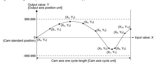
If "input value = 0" and "input value = cam axis one cycle length" are not set in the coordinate data, a control is executed by the line created from the closest two points.
