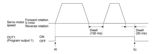
2) Program example 2 Using [Pr. PT23] to [Pr. PT25], you can switch off OUT1 (Program output 1) to OUT3 (Program output 3) automatically.
