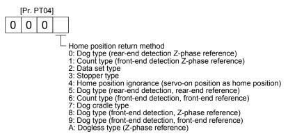
(b) Select the starting direction for the home position return with [Pr. PT04 Home position return type]. Setting "0" starts the home position return in a direction of increasing the address from the current position. Setting "1" starts the home position return in a direction of decreasing the address from the current position.
