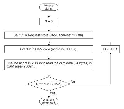
Note. The size of cam data is fixed to 8388 bytes. Thus, N, the setting range of the cam storage area is 0 to 131. Only a part of cam data cannot be written. Write the cam data stored in all areas.
