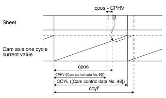
Decrease the conveyor travel distance by subtracting the difference (cpos - CPHV) from the cam axis one cycle current value. Adjust the filter time constant for acceleration/deceleration at compensation with [Cam control data No. 61 Cam position compensation time constant].
