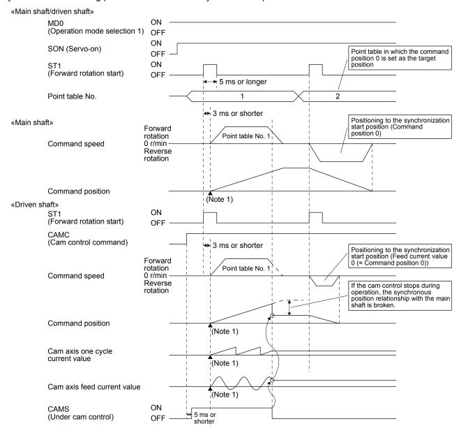
The above shows an example for when the synchronization starting point is the point where both command position and feed current value are "0".
