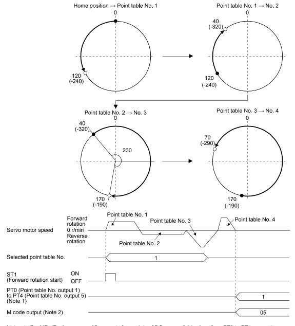
Note 1. For MR-JE-\_A servo amplifiers, up to four points of DO are available; therefore, PT0 to PT4 cannot be outputted simultaneously.
