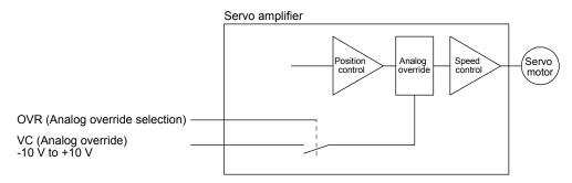
Select a changed value by using OVR (Analog override selection).
