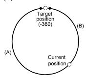
b) When using the shortest rotation specification ( [Pr. PT03] = \_ 1 \_ \_)
