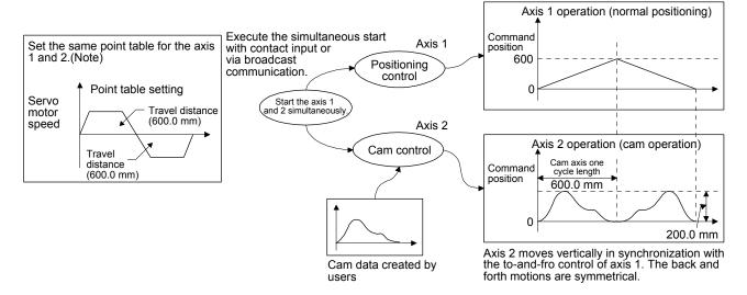
Note. Input the same positioning commands (point table data) to the driven shaft (axis 2) as those for the main shaft (axis 1).
