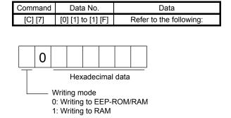
When changing the acceleration time constant frequently using communication, set "1" to the write mode to change only the RAM data in the servo amplifier.
