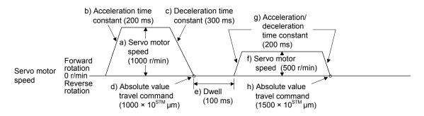
Using the S-pattern acceleration/deceleration time constants reduces abrupt movements at acceleration or deceleration. When the "STD" command is used, [Pr. PC03 S-pattern acceleration/deceleration time constant] does not function.
