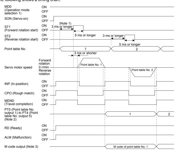
Note 1. The detection of external input signals is delayed by the set time in the input filter setting of [Pr. PD29].
