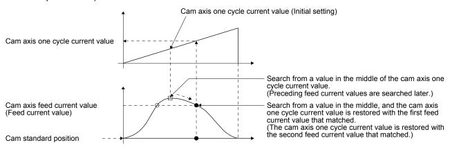
3) Searching from a value in the middle of the cam axis one cycle current value (Cam data start position ≠ 0)
