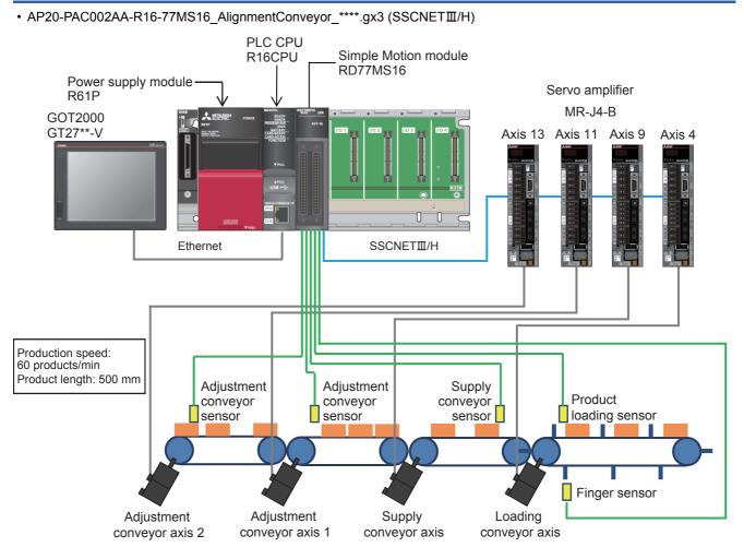
AP20-PAC002AA-R16-77GF16\_AlignmentConveyor\_\*\*\*\*.gx3 (CC-Link IE Field Network)
