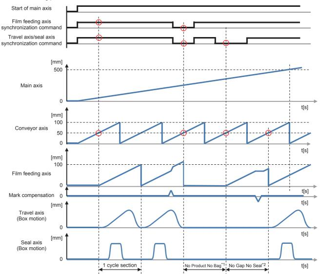
\*1 When workpieces are not conveyed or spaces between workpieces are too wide, this function stops the travel axis, seal axis, and film feeding axis to prevent packaging mistakes.
