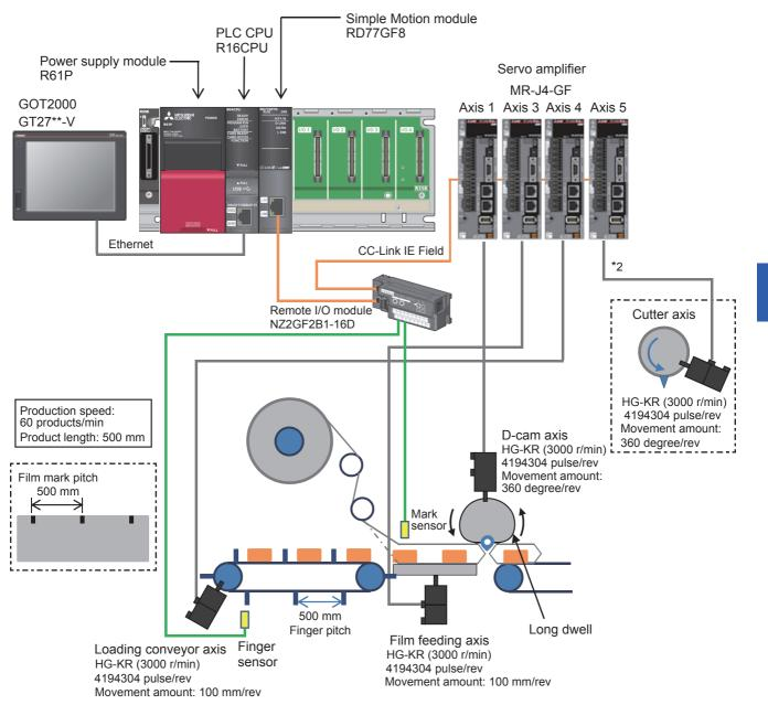
\*2 The end seal part has been configured with the long dwell. This application package also includes programs to generate cam patterns for using the rotary cutter.
