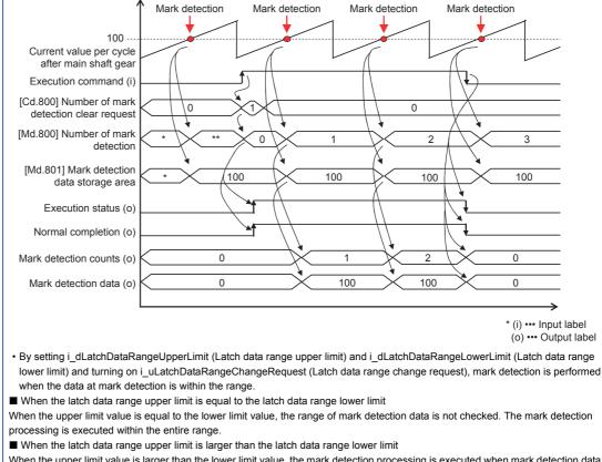
When the upper limit value is larger than the lower limit value, the mark detection processing is executed when mark detection data is "equal to or larger than the lower limit value and smaller than the upper limit value".
