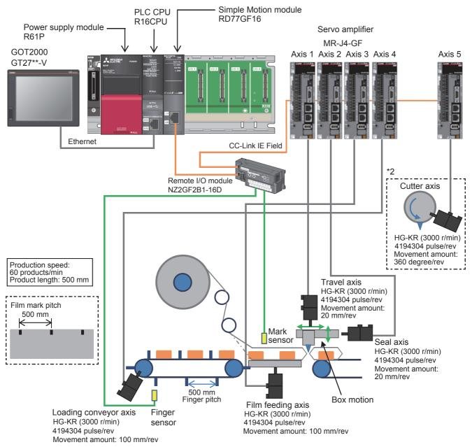
\*2 The end seal part has been configured with the box motion. This application package also includes programs to generate cam patterns for using the rotary cutter.
