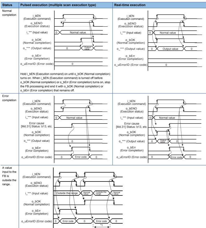
\*1 When a value outside the range is input during normal operation, an error code is output but the previous operation continues. After that, when a normal value is input, the error code is cleared.
