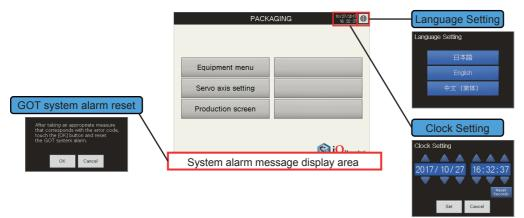
The following shows the basic layout of a main screen.
