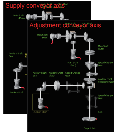
Alignment conveyor Each axis synchronous control setting
