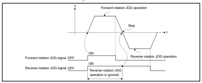
(2) If the JOG operation signal turns ON during deceleration due to OFF of the JOG operation signal, the axis decelerates to a stop down to speed 0 and then resumes JOG operation.
