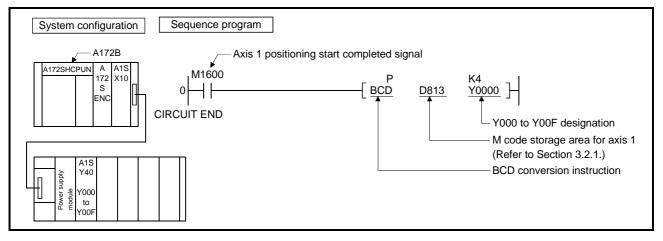
(2) A program that outputs the M code for axis 1 from Y000 to Y00F to an external destination on completion of positioning and after conversion to BCD code, is shown here.
