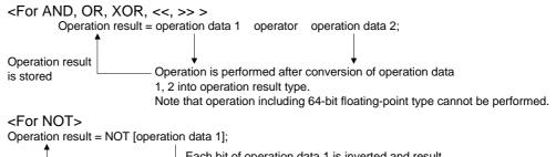
Each bit of operation data 1 is inverted and result of inversion is stored into operation result.
