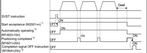
Fig. 3.5 Positioning Completed Signal ON/OFF Timing
