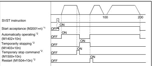
Fig. 3.2 Temporarily Stopping Signal ON/OFF Timing
