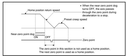
(2) Adjust the position where the near-zero point dog turns OFF so that the "home position return second travel" becomes half of the travel corresponding to one motor revolution.
