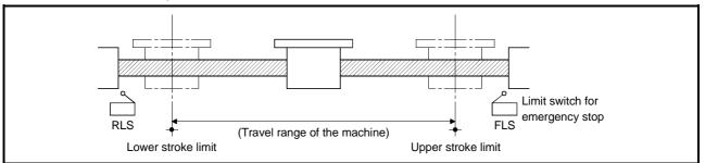
Fig. 4.1 Travel Range When Setting the Upper Stroke Limit Value and Lower Stroke Limit Value
