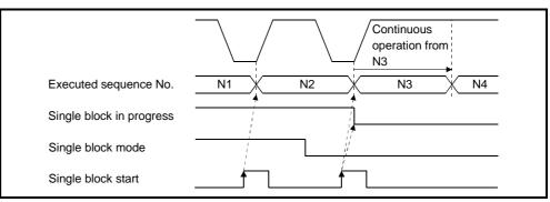
(5) How to perform continuous operation from a start (Ordinary operation) With the single block in progress signal OFF, start a program with SVST to run the program continuously.
