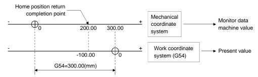
On completion of a home position return, the machine value is equal to 200.00(mm) and the present value to -100.00(mm).
