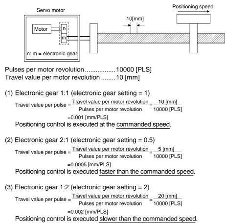
The relationship between the commanded speed (positioning speed set in the servo program) and actual speed (actual positioning speed) is shown below for different electronic gear settings.
