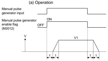
Output speed (V1) = (number of input pulses/ms) $\times$  (manual pulse generator 1-pulse input magnification setting) Travel (L) = (travel per pulse)  $\times$  number of input pulses $\times$  (manual pulse generator 1-pulse input magnification setting)
