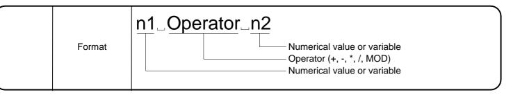
Program designed to carry out positioning according to the result of the specified operation.
