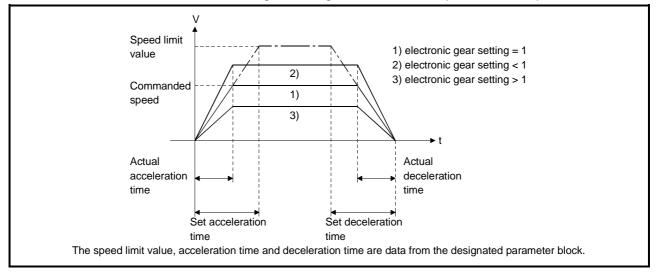
Figure 7.2 Relationship Between Commanded Speed and Actual Speed
