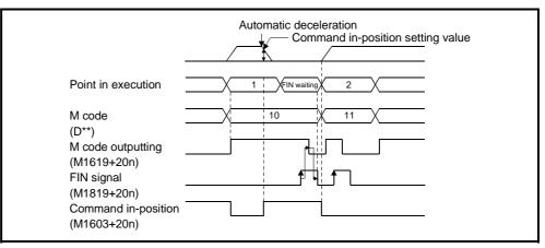
2) When the axis moves to the next point without automatic deceleration being made by positioning to the executed point during FIN waiting If the axis moves to the next point without automatic deceleration, the command in-position signal does not turn ON.
