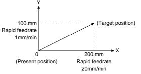
After the above program is run, the target position reaching time of each axis is as follows.
