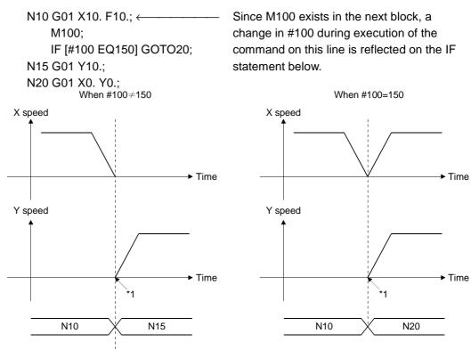
\*1 When M100 is executed, CP does not continue from N10 to N15 or from N10 to N20 and the axis decelerates to a stop once after execution of N10.
