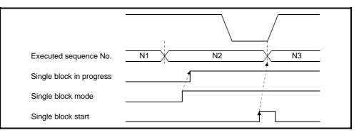
A macro instruction block, e.g. arithmetic operation, is preread during execution of the move instruction for PTP (e.g. G00) or CP (e.g. G01). Therefore, if the single block function is executed while the macro instructions are preread during motion, the executed block number and executed sequence number displayed are those in the preread area.
