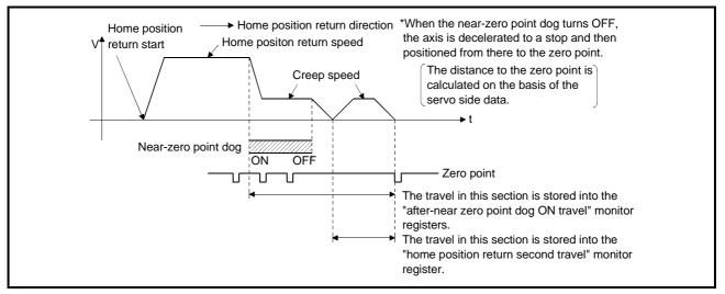
Fig. 7.3 Near-Zero Point Dog Type Home Position Return Operation
