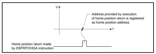
Fig. 7.5 Data Setting Type Home Position Return Operation
