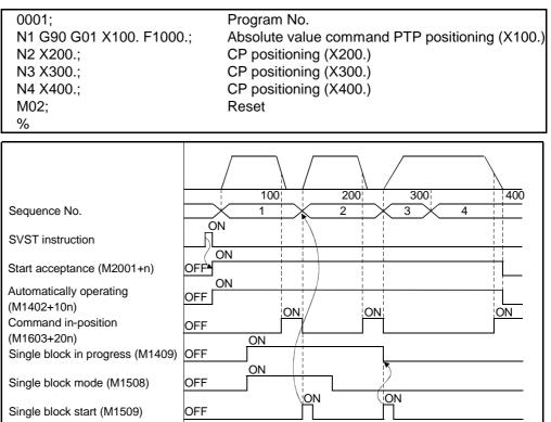
Fig. 3.3 Single Block Signal Timings
