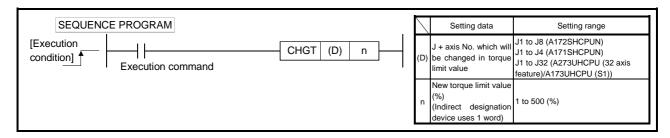
This instruction changes the torque limit value on the leading edge (OFF to ON) of the CHGT instruction execution command in the sequence program.
