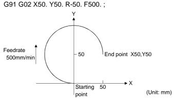
$\bullet$  Program which draws a circular arc of less than  $180^\circ$  at a positive circular arc radius (R) value.
