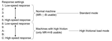
(2) Increase the response setting step by step starting from the low-speed response setting, observing the vibration and stop stabilization of the motor and machine immediately before stopping as you do so. If the machine resonates, decrease the set value.
