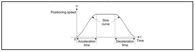
As shown below, the S curve ratio setting serves to select the part of the sine curve to be used as the acceleration and deceleration curve.
