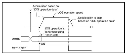
(2) Set the axes for JOG operation to the JOG operation simultaneous start axis setting area (D1015).
