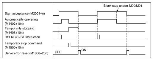
(c) When the error reset command is turned ON during automatic operation (M1402+10n/M4002+10n ON), the above reset processing is performed after the stop processing is carried out under the temporary stop command (M1500+10n/M4400+10n).
