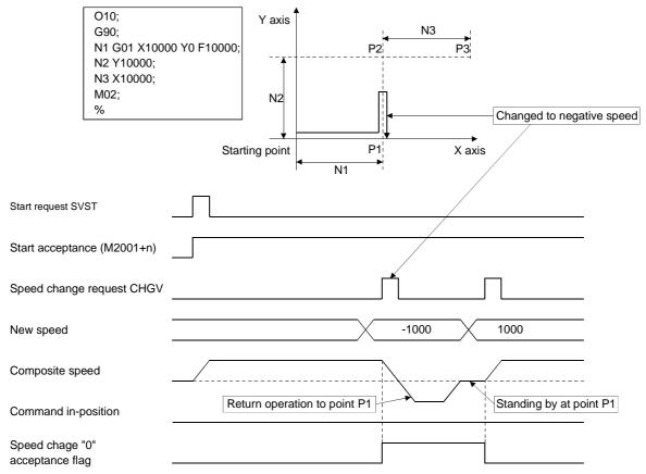
When a speed change is made to negative speed during positioning to P2 in the N2 block as shown above, the axis returns to P1 along the track specified in the program and stands by at P1.
