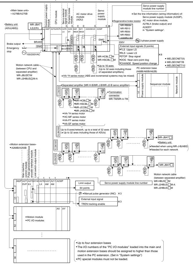
The system configuration example of the motion controller (SV43) is shown below.
