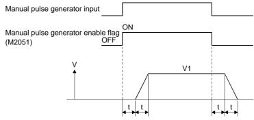
Output speed (V1) = (number of input pulses/ms)  $\times$  (manual pulse generator 1-pulse input magnification setting) Travel (L) = (travel per pulse)  $\times$  (number of input pulses)  $\times$  (manual pulse generator 1-pulse input magnification setting)
