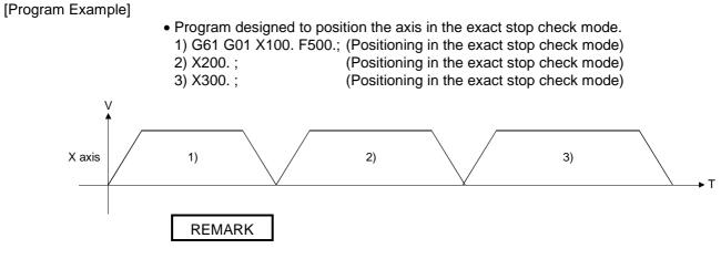
• Only the rapid feedrate may be the specified speed in G00. To specify the speed every time PTP positioning is executed, you can use G61 and G01.
