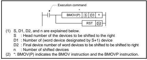
Fig.4.2. Format for Right Shift Using BMOV(P) Instruction and RST Instruction
