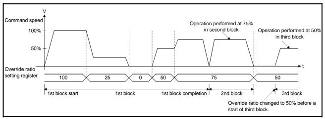
Fig. 7.7 Operation Timing at Override Ratio Setting
