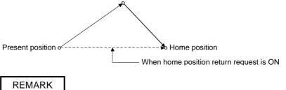
• When the G28 command is given, a home position return is made at rapid feedrate.
