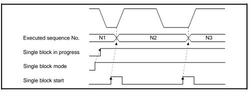
(4) How to start operation continuously during execution of single block Turn ON the single block mode signal. In this state, turn the single block start signal from OFF to ON. This turns OFF the single block in progress signal and starts the program running continuously.
