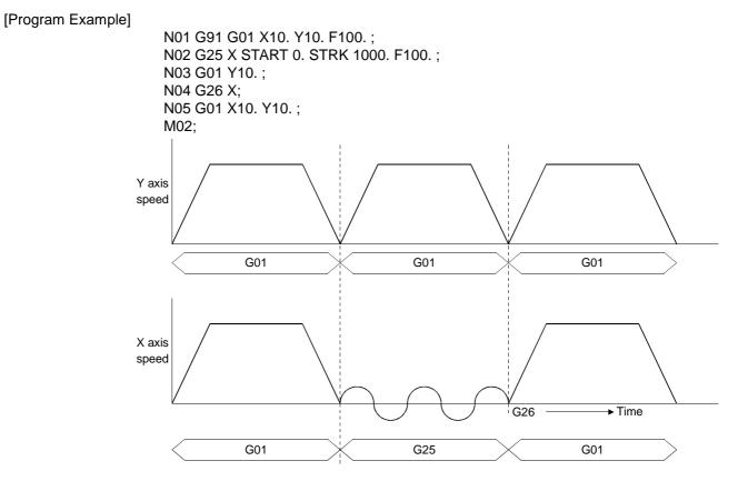
• If the start command of the X axis (high-speed oscillation start axis) is described in the N03 block, a minor error (error code: 581) is displayed when this block is executed, and this program is suspended.
