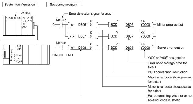
Appendix 4.5 Magnitude Comparison and Four Fundamental Operations of 32-Bit Monitor Data
