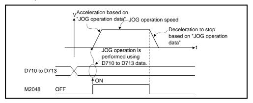
(2) Set the axes for JOG operation to the JOG operation simultaneous start axis setting areas (D710 to D713).
