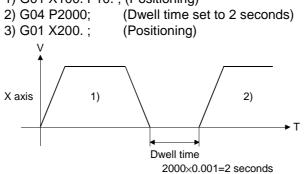
The X axis is positioned to 100., stops there for 2 seconds, and starts positioning operation to 200. again.
