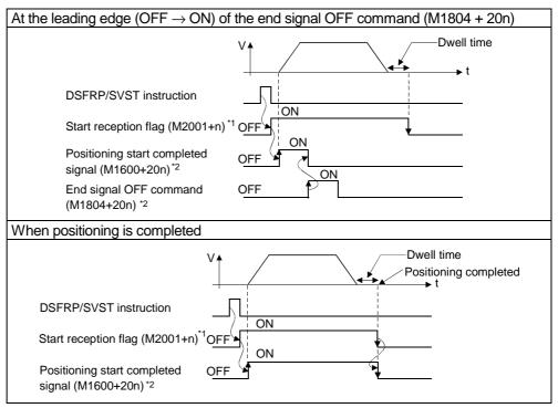
Fig. 3.4 Positioning Start Completed Signal ON/OFF Timing
