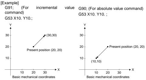
• Positioning data can be set by direct designation (numerical value) or indirect designation (variable: #\*\*\*\*).
