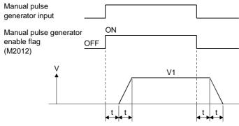
Output speed (V1) = (number of input pulses/ms) $\times$  (manual pulse generator 1-pulse input magnification setting) Travel (L) = (travel per pulse) $\times$  number of input pulses $\times$ (manual pulse generator 1-pulse input magnification setting)
