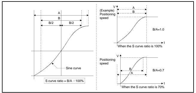
Note: Under G00 including M code, G01, G02, G03 or G32, the S curve ratio is ignored and operation is always performed at the ratio of 0%.
