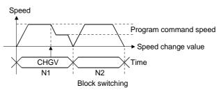
\*7: The F (speed) command is used. Note that it is clamped at the speed change value.
