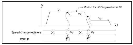
Fig. 7.6 Operation Timing for Speed Change
