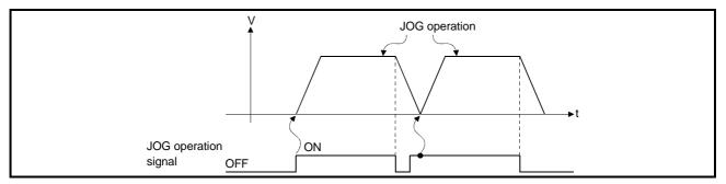
(3) In the test mode using the peripheral device, JOG operation under control of the JOG operation signal (M1802+20n/M1803+20n/M3202+20n/M3203+20n) is not performed.
