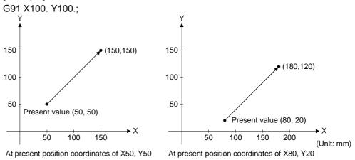
• Positioning data can be set by direct designation (numerical value) and indirect designation (variable: #\*\*\*\*).
