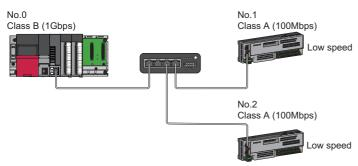
No.0: Master station No.1, No.2: Remote station Class A: CC-Link IE TSN Class A device Class B: CC-Link IE TSN Class B device
