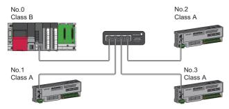
No.0: Master station No.1, No.2, No.3: Remote station Class A: CC-Link IE TSN Class A device Class B: CC-Link IE TSN Class B device When the "Communication Mode" is "Multicast", communication may not be possible depending on the communication
