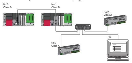
No.0: Master station No.1: Local station No.2, No.3: Remote station (1), (2): Ethernet device Class A: CC-Link IE TSN Cla
