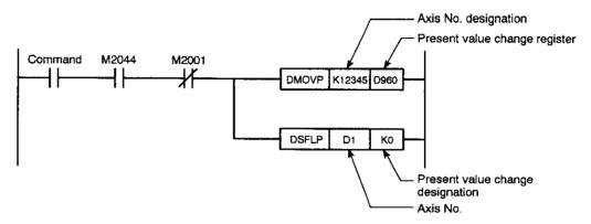
(2) Virtual servomotor speed change program (axis 1, A273UHCPU 8-axis specification):
