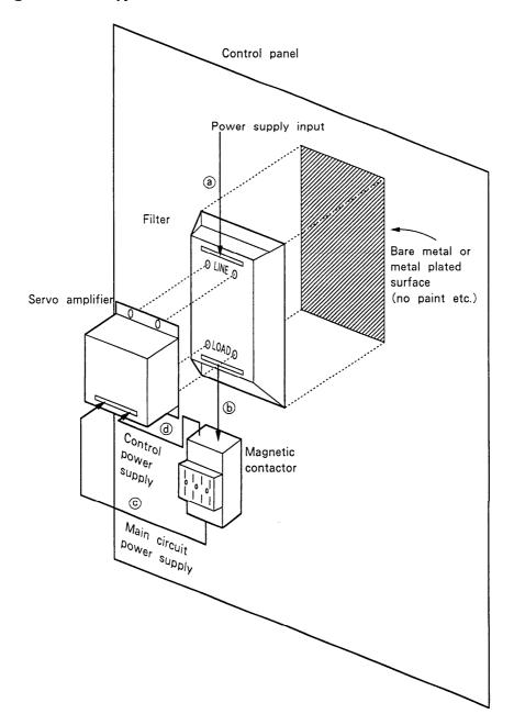
The filter is installed between the servo amplifier and panel as shown above. The surface inside the panel where the filter is to be installed must be bare metal or metal plated surface so that the rear surface of the filter electrically contacts the panel. The filter input wire @ must be kept as far apart from the output wires ⑤, ⓒ and ⑥. Keep the wiring (⑥, ⓒ, ⑥) between the filter and servo amplifier as short as possible. (Total 1.5 m or less.)
