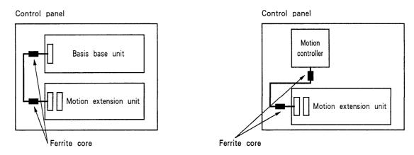
Always install one ferrite core to the motion extension base connection cable and PLC extension base connection cable using a batch shield cable. Place the ferrite core at a position within 10 cm from each basic base unit (motion controller). By installing a ferrite core on the extension side, the noise measures will be more effective.
