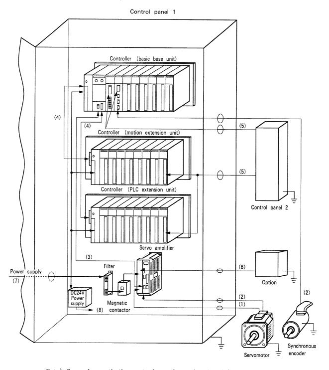
Note) Securely earth the control panel, option 1 and 2, and the motor.
