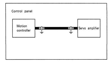
(4) Motion extension base connection cable, PLC extension base connection cable
