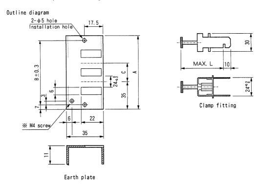
\*) This is the screw hole for earthing. Connect to the earth plate on the control panel.
