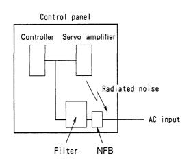
The power supply line noise is eliminated by the filter, but cable contains noise again because of the noise radiated in the control panel.
