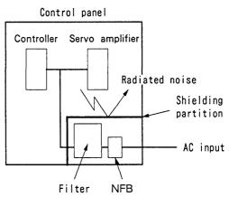
Use a metal plate, etc., for the shielding partition. Make sure there are no gaps.
