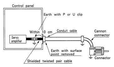
(B) Using shield cable and conduit
