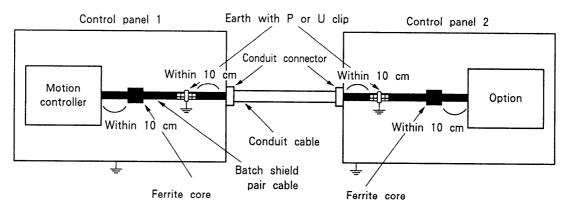
(B) Using shield cable and conduit
