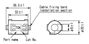
(3) For A278LX, A273EX, I/O cable and other cables: ZCAT3035-1330 (TDK)
