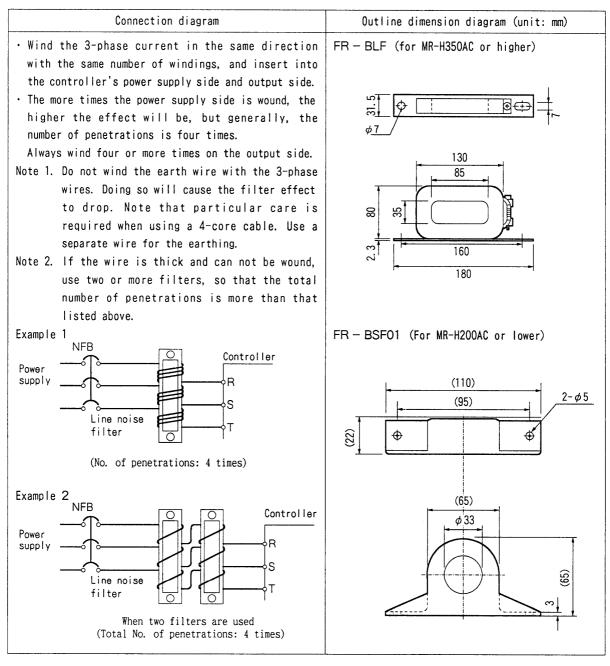
This noise line filter can be used on the feedback cable and control signal cable, etc., in addition to the power line and output line. In this case, the No. of penetrations is approx. 4 times.
