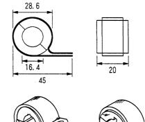
(2) For PLC extension base connection cable: ZCAT2032-0930 (TDK)
