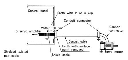
(C) Using shield cable and conduit
