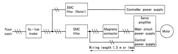
(2)When the servo amplifier does not have a control power supply input (MR-J)
