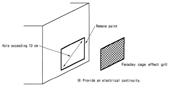
(4) The control panel door must be accurately earthed with the control panel unit. If the door earthing is insufficient, the door itself will act as a large antenna and will radiate noise.
