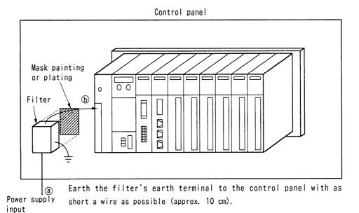
The filter is installed in the panel as shown above. Mask the painted surface of the panel where the filter is to be installed, or plate the surface, so that the rear surface securely contacts the panel.
