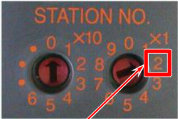
Station #2: Remote I/O station (AJ65BTC1-32T, 32-point, transistor output)
