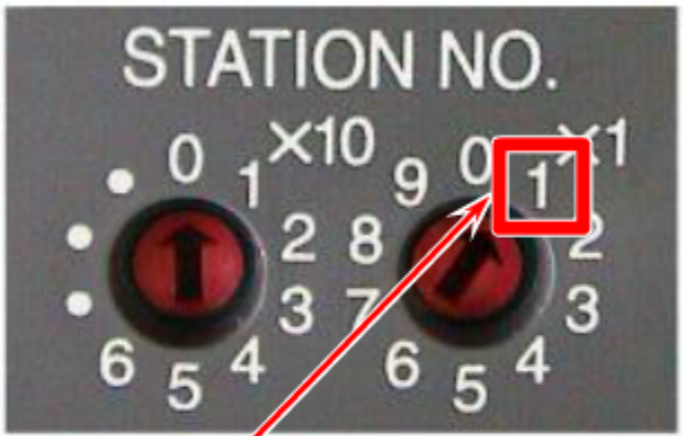
Station #1: Remote I/O station (AJ65BTB2-16D, 16-point, DC input)
