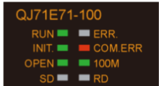
Example of "COM.ERR" indicator ON status
