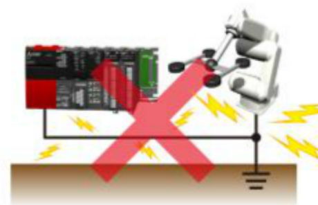
(3) Common grounding....Not allowed
