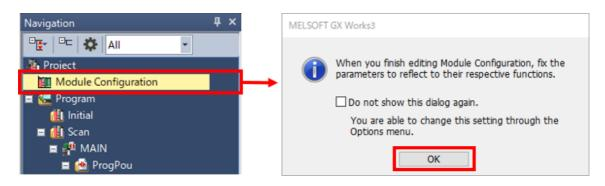
When the module configuration diagram opens, drag and drop the module from the Element Selection window on the right side, and create a module configuration diagram in the same way as that for the system configuration diagram (Section 2.2). For the Motion module, drag and drop a module with (S) at the end of the model.
