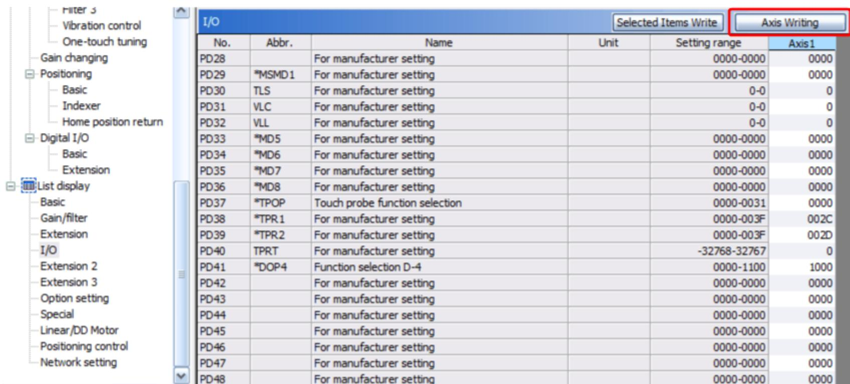
The screenshot shows a software interface for configuring a servo amplifier. On the left, there is a tree view of configuration categories. In the center, a table lists I/O parameters with columns for No., Abbr., Name, Unit, Setting range, and Axis1. The 'Axis Writing' button at the top right of the table is highlighted with a red box.
