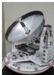
Antenna inside the radome
