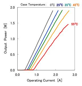
Figure 1: Power-current characteristics
