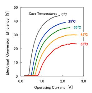
Figure 2: Conversion efficiency-current characteristics
