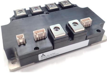
Dual switch (Half-Bridge)
