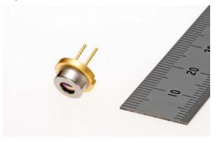
High-power 638nm-wavelength red-laser diode (ML562G86)
