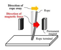
(1) The permanent magnet applies a magnetic force to the rope near the rope terminal so as to amplify the rope sway.
